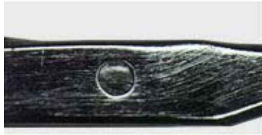
Figure 2.7 Abraded needle ( http://gbu.groz-beckert.com/gbu/gbu_default_e.asp )
