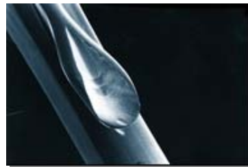
Figure 2.4 Worn Latch
