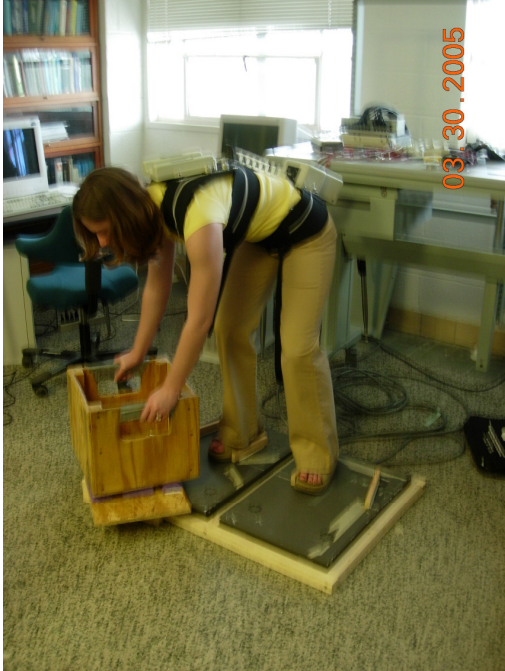
Figure 2.1 Lifting task Apparatus with Box Lowered to Platform
