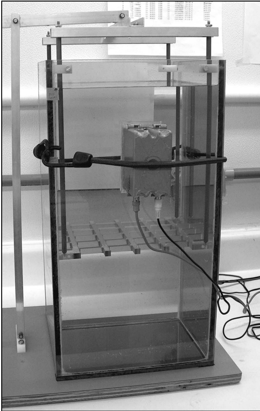
Figure 4. Position of miniature video camera during turbulence experiments.
