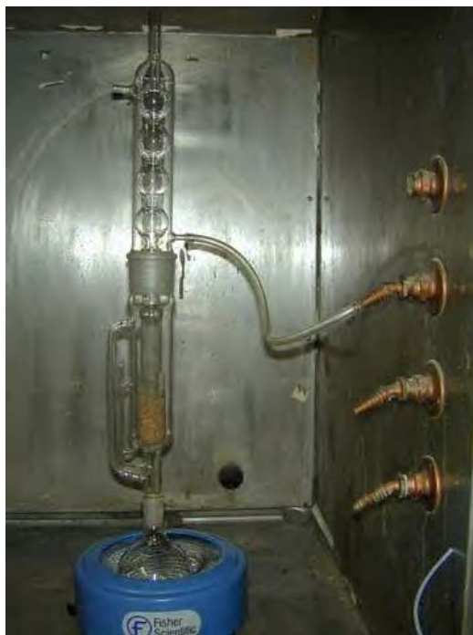
Figure 3.1 Soxhlet extraction setup used for toluene ethanol extractives determination
