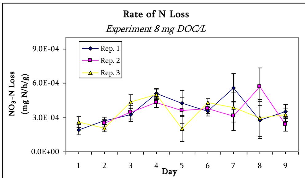
Figure B4. Rate of  $\text{NO}_3\text{-N}$  loss ( $\text{mg N/h/g}$ ) as a function of time for  $8 \text{ mg C/L}$ . Conditions: Argon-purged solution containing  $\approx 5.00 \text{ mg N/L NO}_3^-$  at  $25^\circ\text{C}$ .
