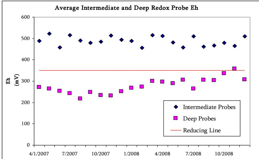
Figure 3. Average Eh in intermediate and deep probes corresponding to intermediate and deep well depth.
