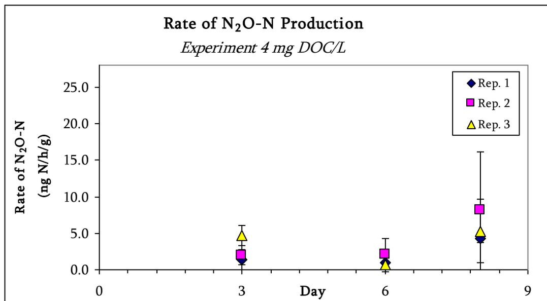
Figure C3. Rate of N<sub>2</sub>O-N production (ng N/h/g) as a function of time for 4 mg C/L. Conditions: Argon-purged solution containing  $\approx 5.00$  mg N/L NO<sub>3</sub><sup>-</sup> at 25°C.
