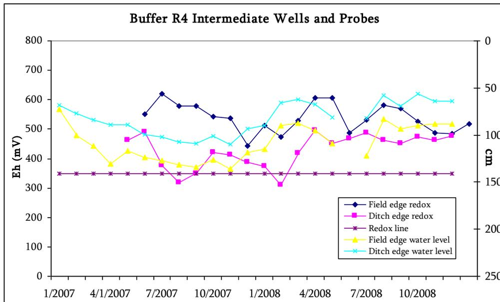
Figure 13. Average groundwater depth and redox measurements for intermediate wells in R4.
