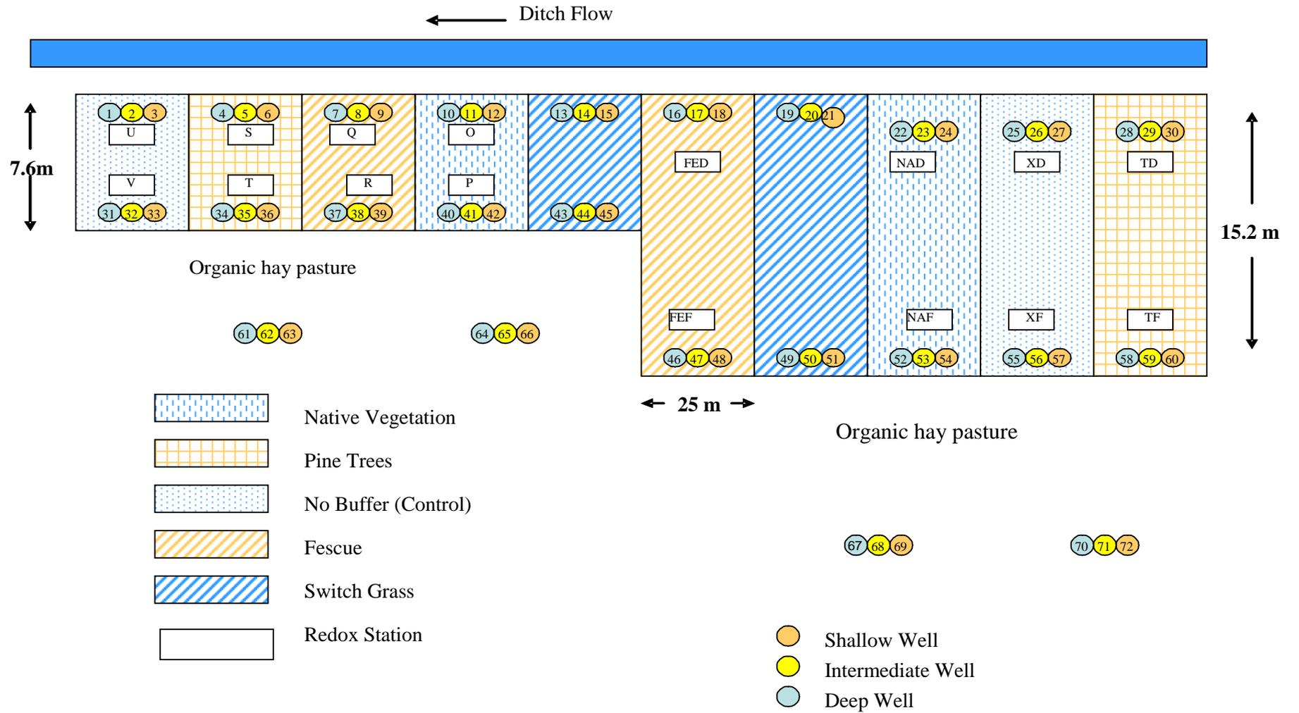
Figure 2. Well numbers and vegetation treatments in R1. Figure not to scale.
