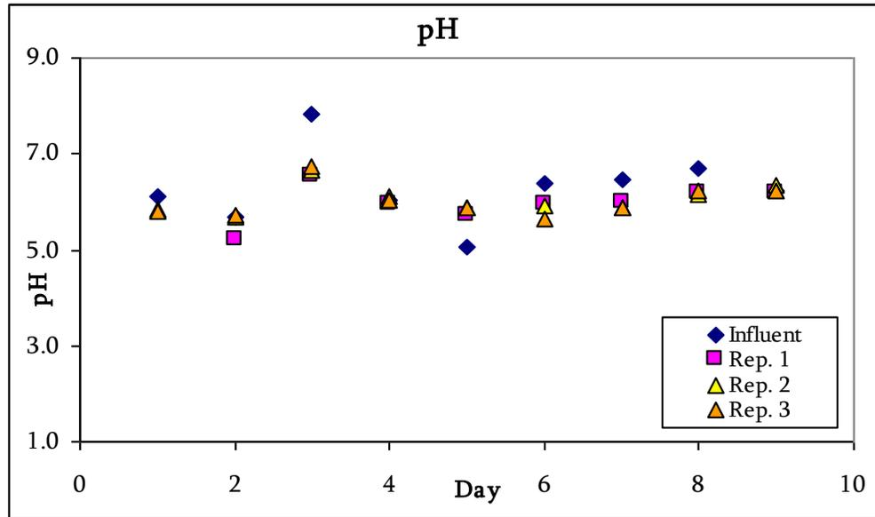
Figure 2. Example pH values as a function of time for a column experiment. Conditions: Argon-purged solution containing 5.0 mg N-NO<sub>3</sub>/L at 25°C.
