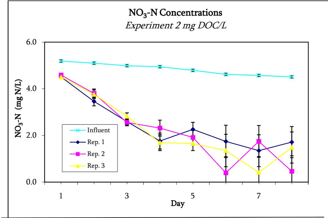
Figure A2. Concentration changes between influent  $\text{NO}_3\text{-N}$  and effluent  $\text{NO}_3\text{-N}$  (mg N/L) as a function of time for 2 mg C/L. Conditions: Argon-purged solution containing  $\approx 5.00$  mg N/L  $\text{NO}_3^-$  at 25°C
