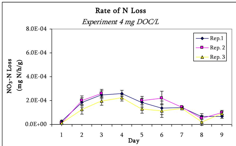
Figure B3. Rate of  $\text{NO}_3\text{-N}$  loss ( $\text{mg N/h/g}$ ) as a function of time for  $4 \text{ mg C/L}$ . Conditions: Argon-purged solution containing  $\approx 5.00 \text{ mg N/L NO}_3^-$  at  $25^\circ\text{C}$ .
