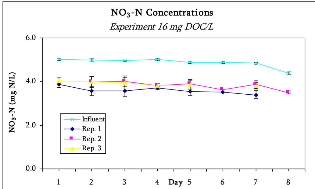
Figure A6. Concentration changes between influent NO<sub>3</sub>-N and effluent NO<sub>3</sub>-N (mg N/L) as a function of time for 16 mg C/L Conditions: Argon-purged solution containing ≈ 5.00 mg N/L NO<sub>3</sub><sup>-</sup> at 25°C.
