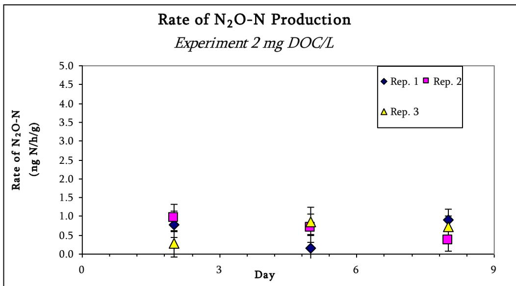
Figure C2. Rate of N<sub>2</sub>O-N production (ng N/h/g) as a function of time for 2 mg C/L. Conditions: Argon-purged solution containing  $\approx 5.00$  mg N/L NO<sub>3</sub><sup>-</sup> at 25°C
