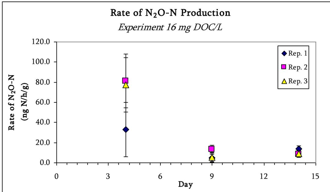
Figure 8. Rate of N<sub>2</sub>O-N production (ng N/h/g) as a function of time for experiment 16 mg DOC/L. Conditions: Argon-purged solution containing  $\approx 5.0$  mg N-NO<sub>3</sub>/L at 25°C.
