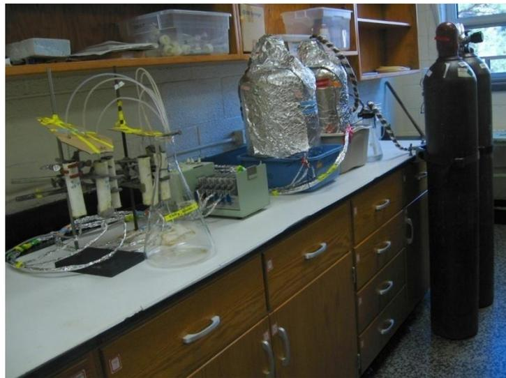
Figure 1. Laboratory set-up; solution (in foil covered carboys). Solution was pumped to soil columns, with flow-rate regulated by a peristaltic pump. Effluent was collected from exit tubing of each column. Conditions: Argon-purged solution containing  $5.0 \text{ mg N/L NO}_3^-$  at  $25^\circ\text{C}$ .
