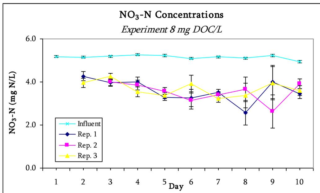
Figure 5. Example of concentration data for a column experiment. Conditions: Argon purged solution containing 5.0 mg N-NO<sub>3</sub>/L at 25°C.
