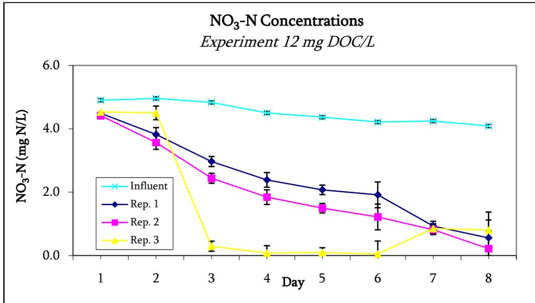
Figure A5. Concentration changes between influent NO<sub>3</sub>-N and effluent NO<sub>3</sub>-N (mg N/L) as a function of time for 12 mg C/L Conditions: Argon-purged solution containing ≈ 5.00 mg N/L NO<sub>3</sub><sup>-</sup> at 25°C.
