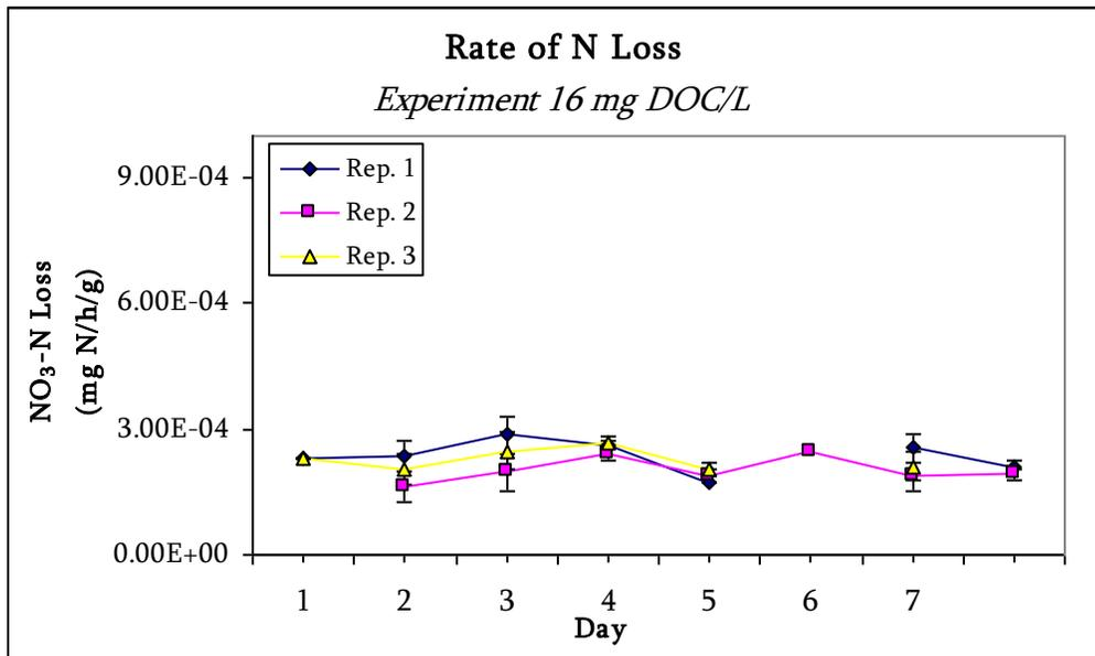
Figure B6. Rate of  $\text{NO}_3\text{-N}$  loss (mg N/h/g) as a function of time for  $16 \text{ mg C/L}$ . Conditions: Argon-purged solution containing  $\approx 5.00 \text{ mg N/L NO}_3^-$  at  $25^\circ\text{C}$ .
