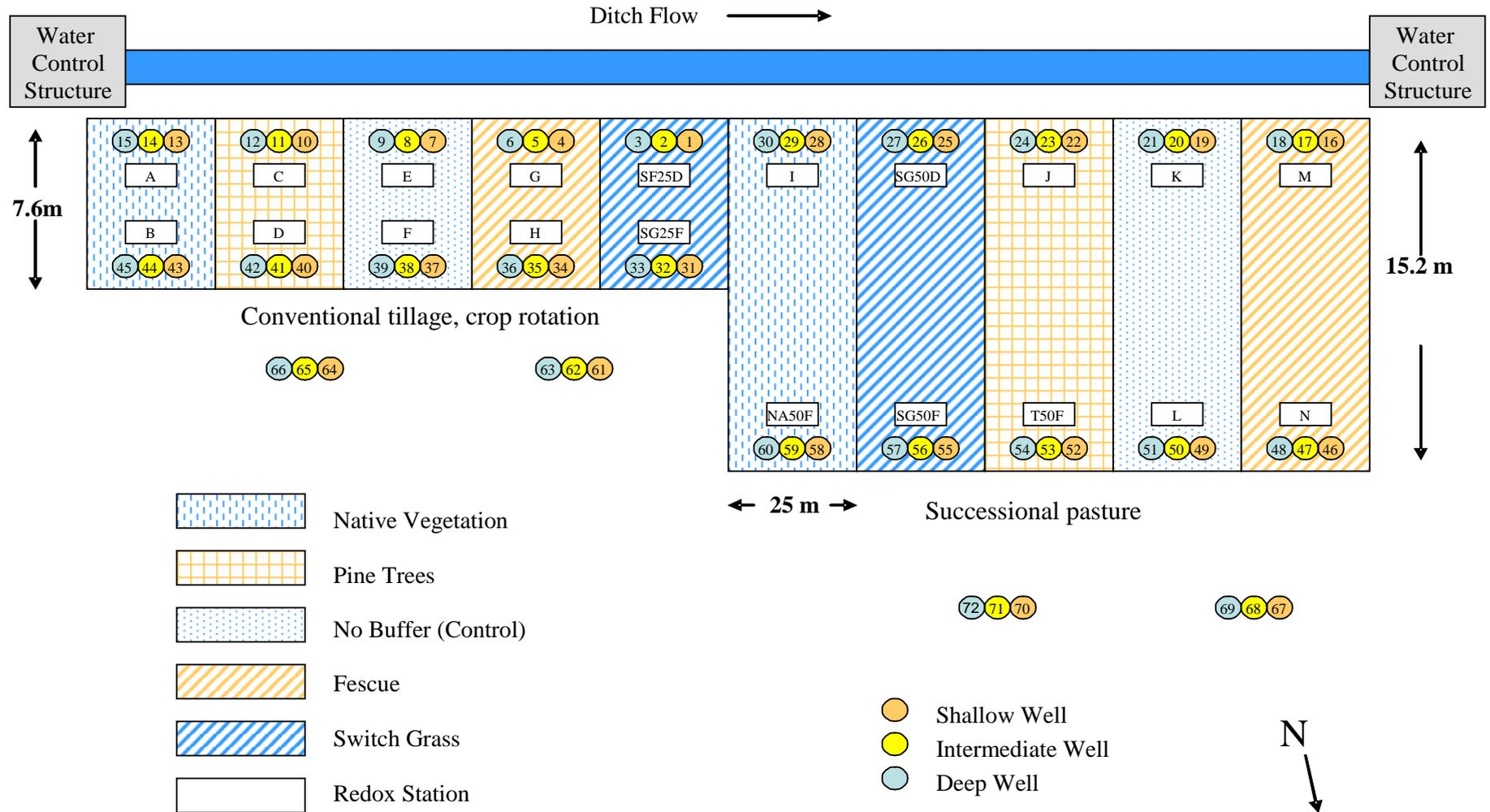
Figure 3. Well numbers and vegetation treatments in R2N. Figure not to scale.
