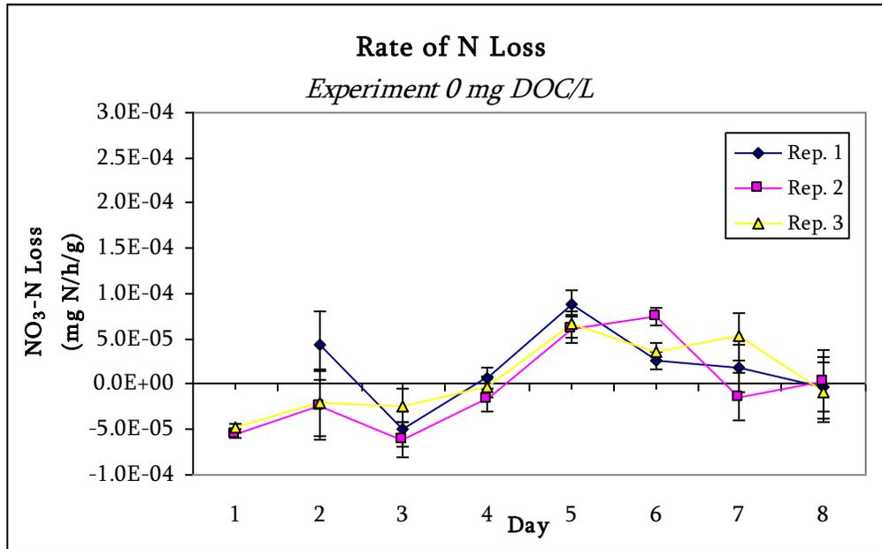
Figure B1. Rate of  $\text{NO}_3\text{-N}$  loss (mg N/h/g) as a function of time for 0 mg C/L. Conditions: Argon-purged solution containing  $\approx 5.00$  mg N/L  $\text{NO}_3^-$  at 25°C.
