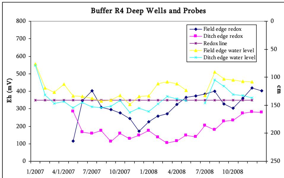
Figure 12. Average groundwater depth and redox measurements for deep wells in R4.
