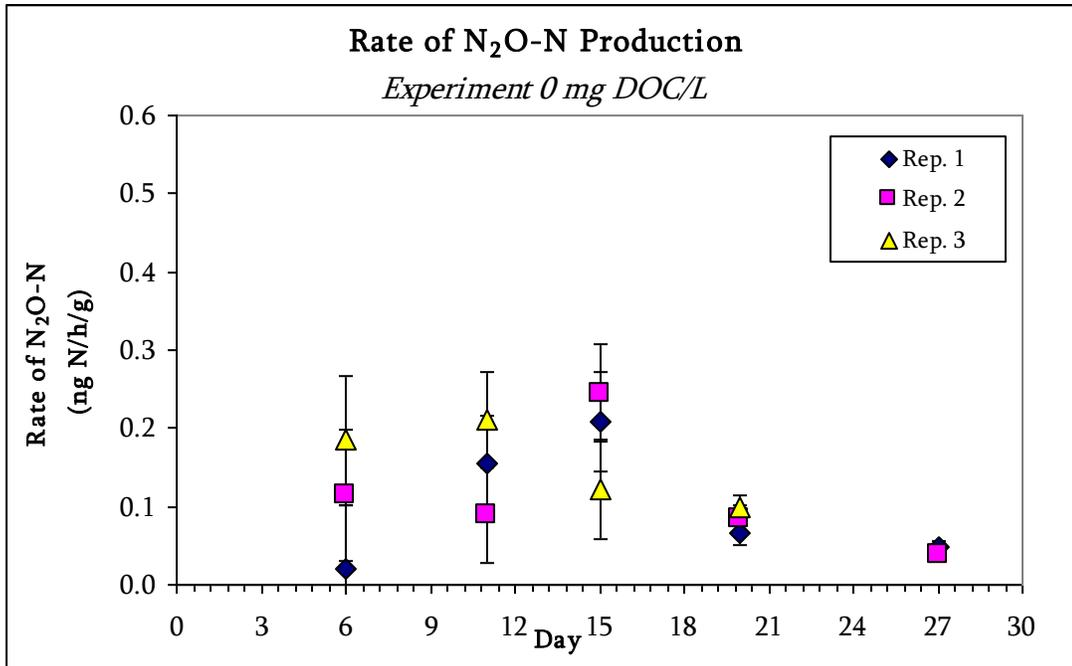
Figure C1. Rate of N<sub>2</sub>O-N production (ng N/h/g) as a function of time for 0 mg C/L. Conditions: Argon-purged solution containing  $\approx 5.00$  mg N/L NO<sub>3</sub><sup>-</sup> at 25°C.
