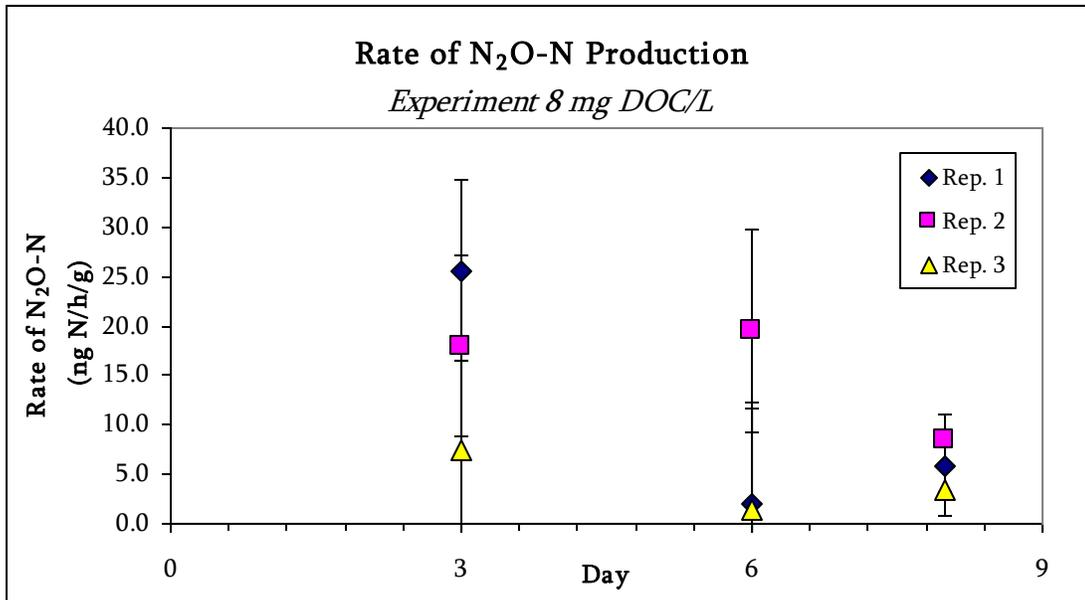
Figure C4. Rate of N<sub>2</sub>O-N production (ng N/h/g) as a function of time for 8 mg C/L. Conditions: Argon-purged solution containing  $\approx 5.00$  mg N/L NO<sub>3</sub><sup>-</sup> at 25°C.
