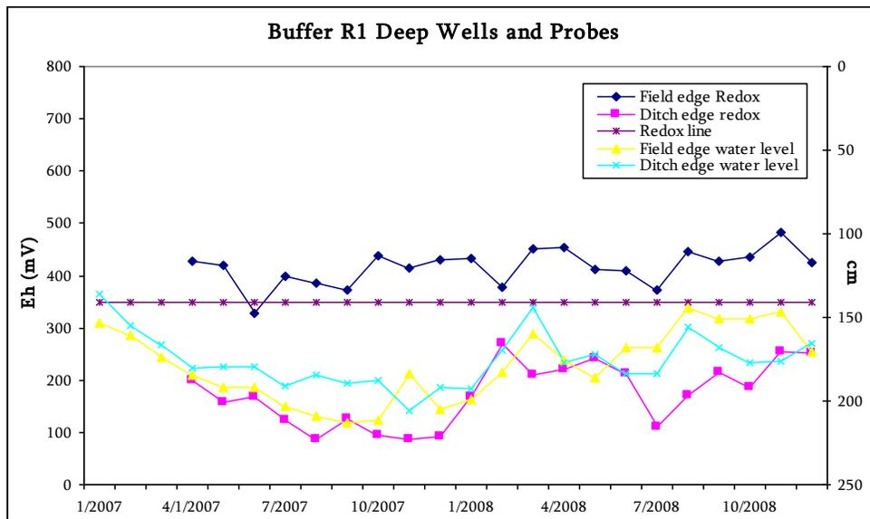
Figure 8. Average groundwater depth and redox measurements for deep wells.
