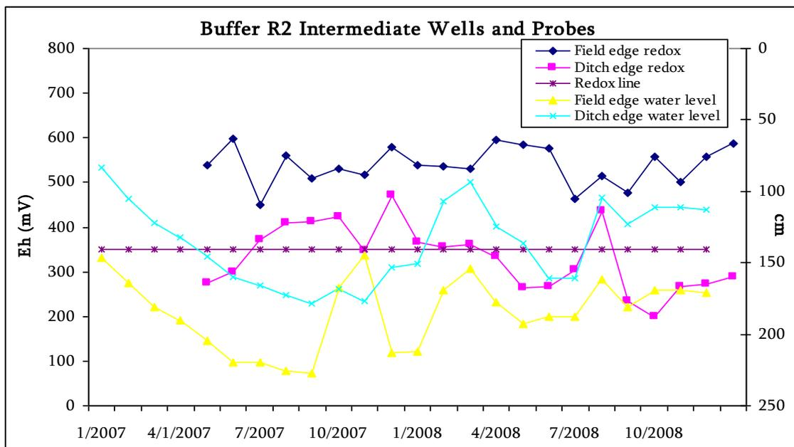
Figure 11. Average groundwater depth and redox measurements for intermediate wells in R2.
