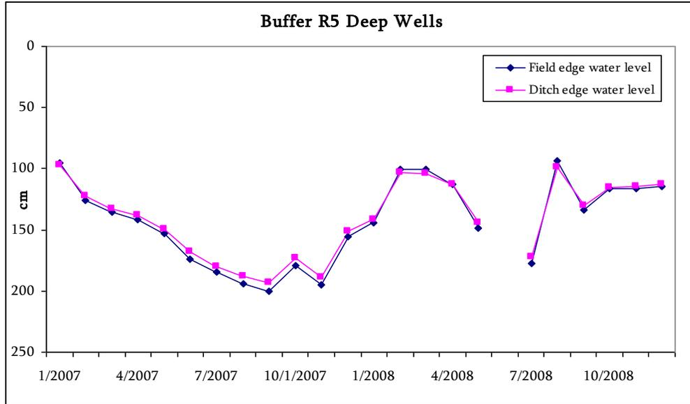
Figure 8. Water table data for deep wells in R5N. Water table depth is recorded as cm below soil surface.
