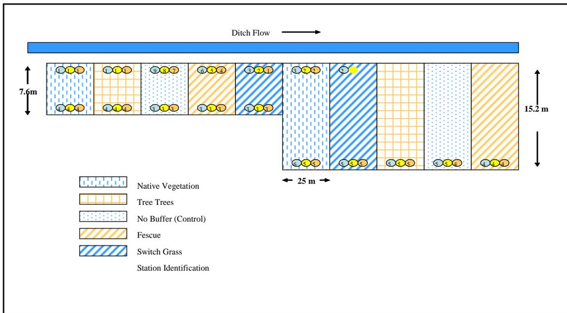
Figure 1. Example of buffer at CEFS illustrating well nest location, and vegetation treatment establishment. Not to scale.
