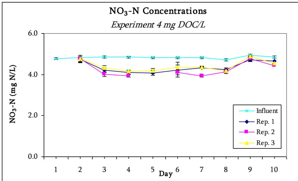
Figure A3. Concentration changes between influent NO<sub>3</sub>-N and effluent NO<sub>3</sub>-N (mg N/L) as a function of time for 4 mg C/L. Conditions: Argon-purged solution containing ≈ 5.00 mg N/L NO<sub>3</sub><sup>-</sup> at 25°C.
