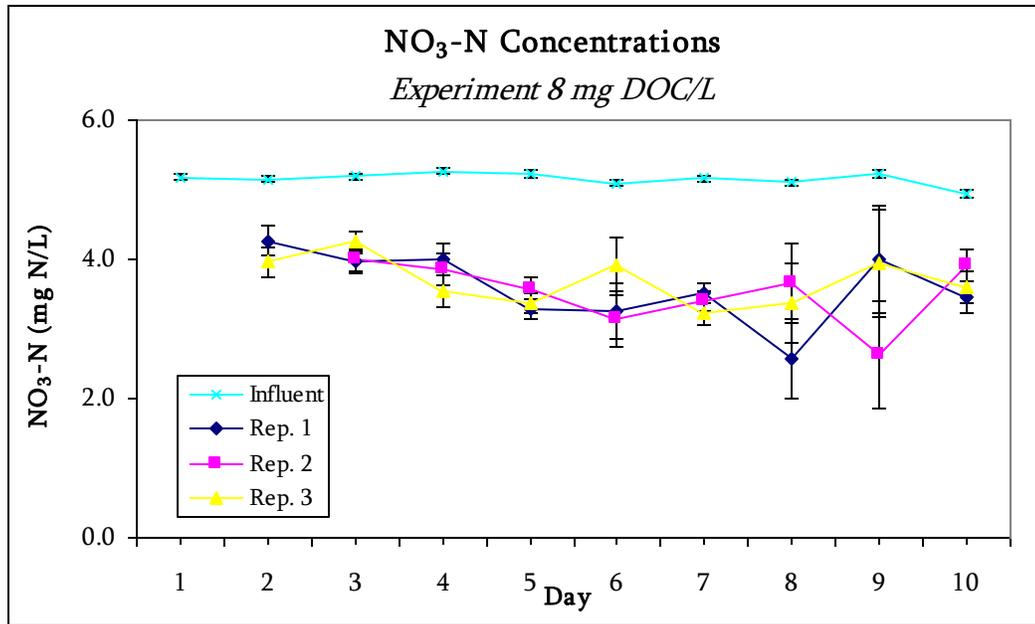
Figure A4. Concentration changes between influent NO<sub>3</sub>-N and effluent NO<sub>3</sub>-N (mg N/L) as a function of time for 8 mg C/L Conditions: Argon-purged solution containing ≈ 5.00 mg N/L NO<sub>3</sub><sup>-</sup> at 25°C.
