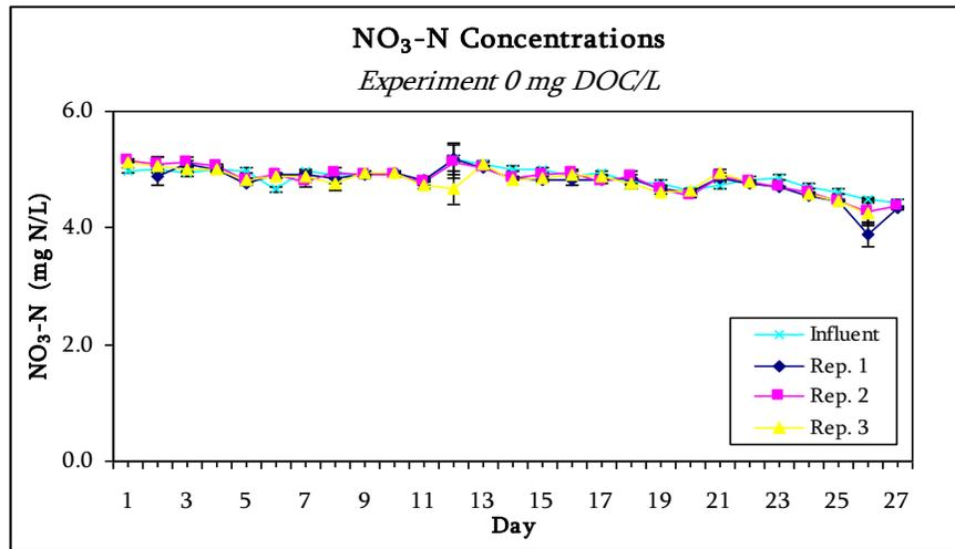
Figure 4. Example of concentration data for a column experiment. Conditions: Argon-purged solution containing 5.0 mg N- $\text{NO}_3/\text{L}$  at 25°C.
