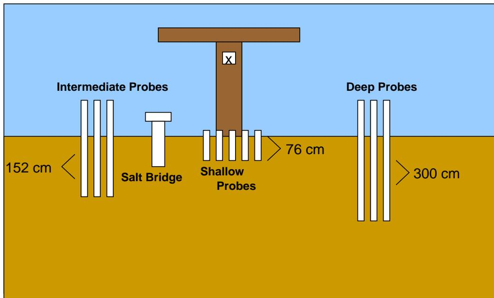
Figure 7. Redox probe depths and establishment around salt bridges for R1, R2N, and R4W.
