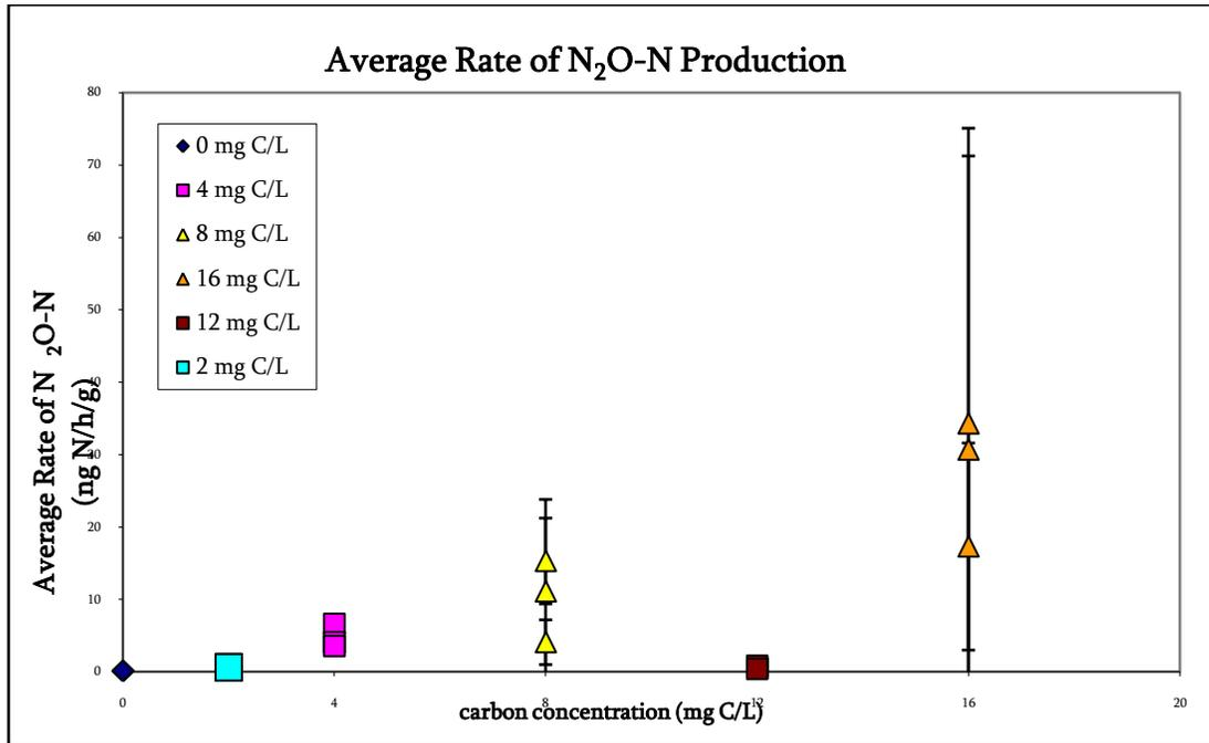
Figure 9. Rate of N<sub>2</sub>O-N production (ng N/h/g) as a function of time DOC concentration. Conditions: Argon-purged solution containing  $\approx 5.0$  mg N/L NO<sub>3</sub> at 25°C.
