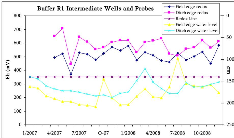
Figure 9. Average groundwater depth and redox measurements for intermediate wells in R1.
