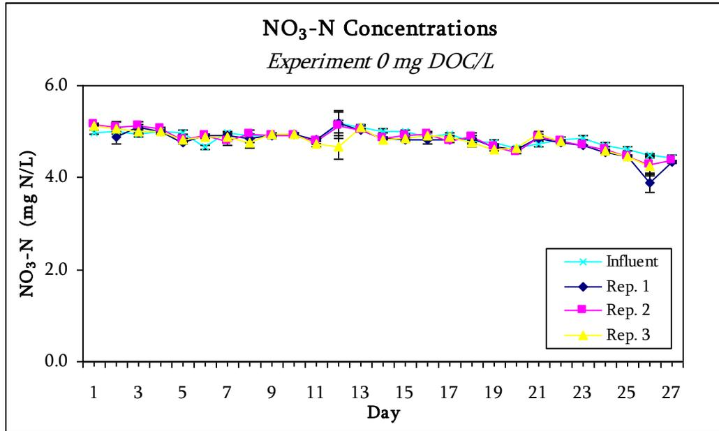
Figure A1. Concentration changes between influent NO<sub>3</sub>-N and effluent NO<sub>3</sub>-N (mg N/L) as a function of time for 0 mg C/L. Conditions: Argon-purged solution containing ≈ 5.00 mg N/L NO<sub>3</sub><sup>-</sup> at 25°C.
