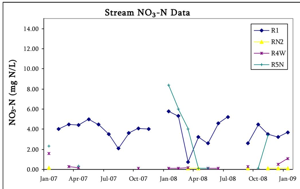
Figure 10. Stream data for drainage ditches adjacent to buffers. Ditches were frequently dry due to drought conditions.
