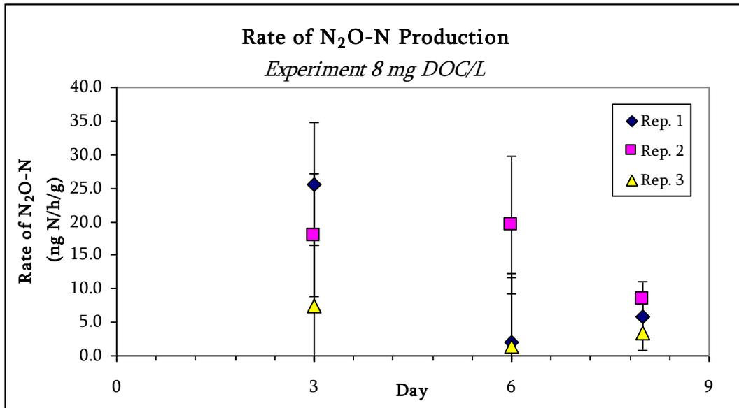
Figure 7. Rate of N<sub>2</sub>O-N production (ng N/h/g) as a function of time for experiment 8 mg DOC/L. Conditions: Argon-purged solution containing 5.0 mg N-NO<sub>3</sub>/L at 25°C.
