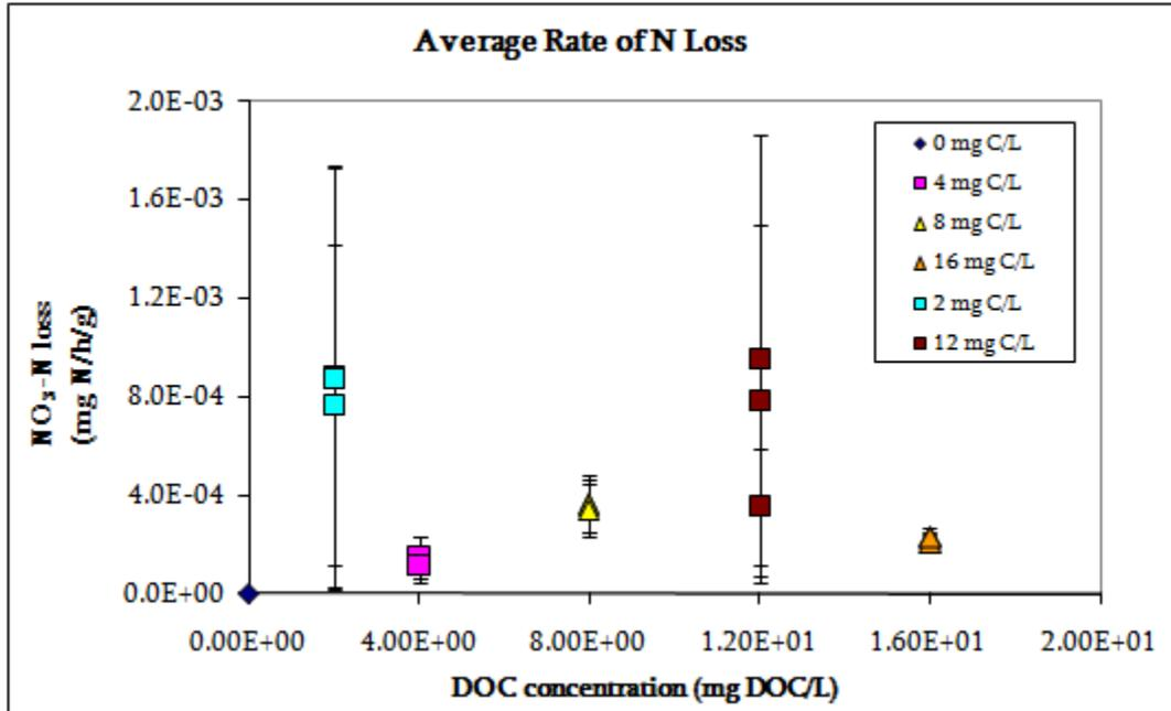
Figure 6. Average rate of NO<sub>3</sub>-N loss (mg N/h/g) as a function of DOC concentration. Conditions: Argon-purged solution containing 0 mg N-NO<sub>3</sub>/L at 25°C.
