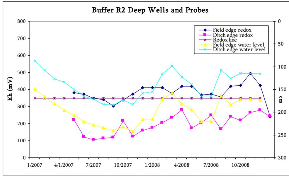
Figure 10. Average groundwater depth and redox measurements for deep wells in R2.
