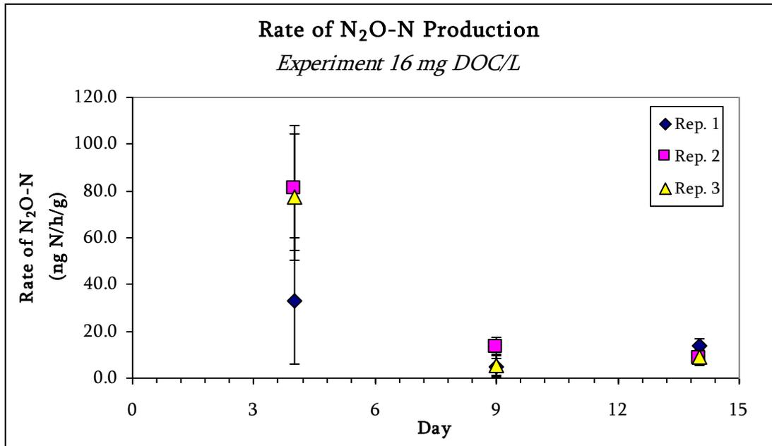
Figure C6. Rate of  $N_2O-N$  production (ng N/h/g) as a function of time for 16 mg  $C/L$ . Conditions: Argon-purged solution containing  $\approx 5.00$  mg N/L  $NO_3^-$  at 25°C.
