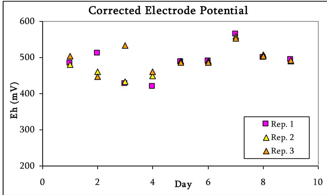
Figure 3. Example of time course of Eh (mV) measured on the outlet of columns. Conditions: Argon-purged solution containing 5.0 mg N/L  $\text{NO}_3^-$  at 25°C.
