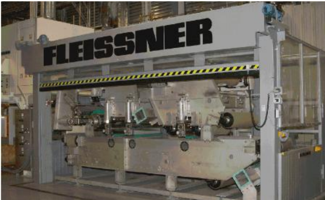
Figure 2.2: Photograph of the NCRC Hydroentangling device
