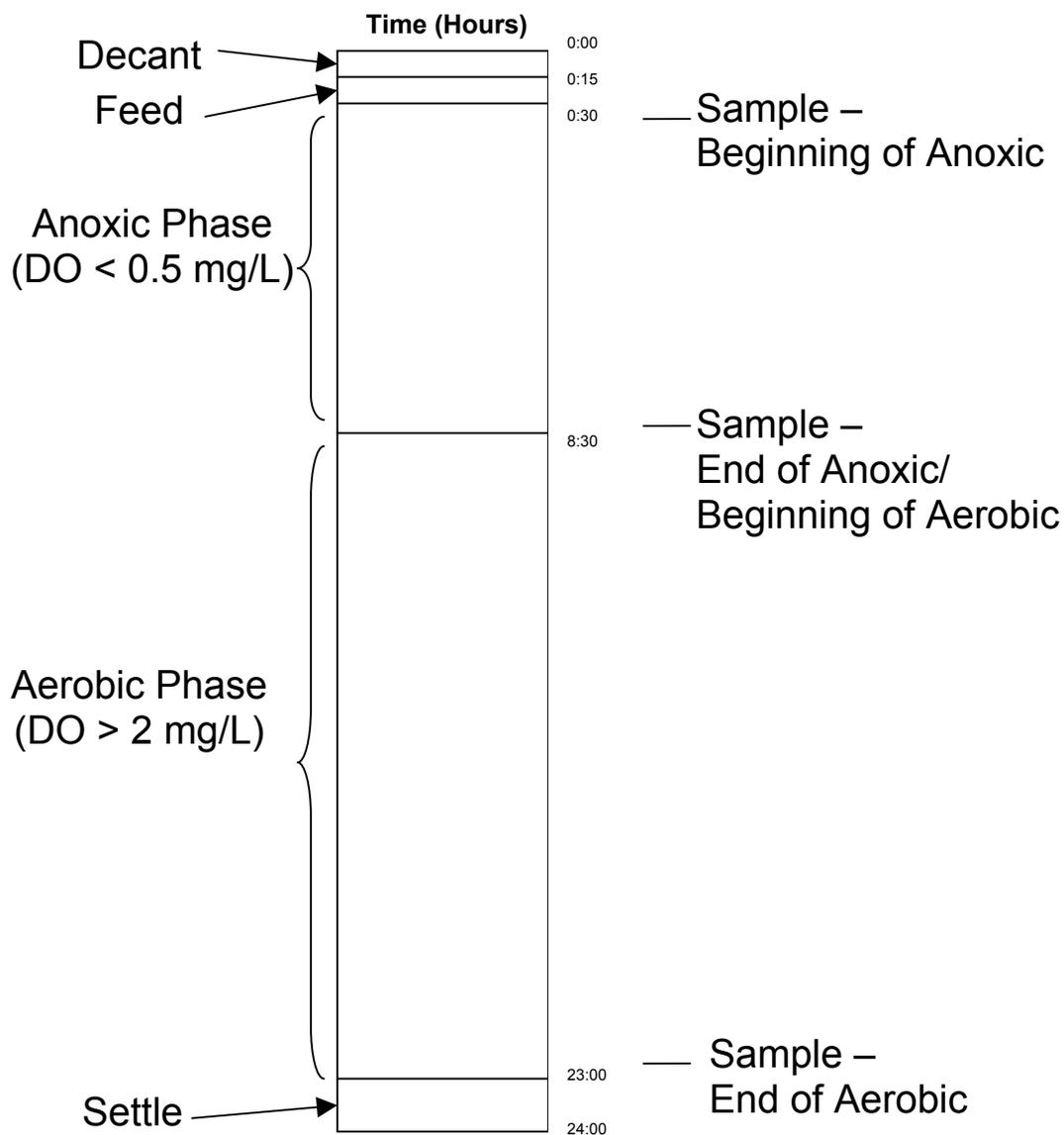
**Figure 3.4 Anoxic/Aerobic Reactor Procedure (One Cycle)**
