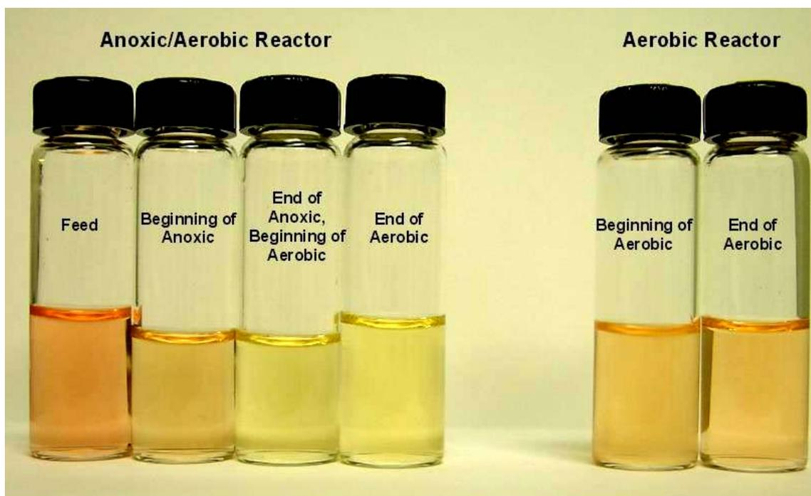
**Figure 4.50 Visual Comparison of Samples Containing Reactive Red 198 and Reactive Yellow 86**
