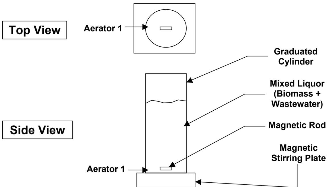
**Figure 3.2 Small Anoxic/Aerobic Reaction Vessel**
