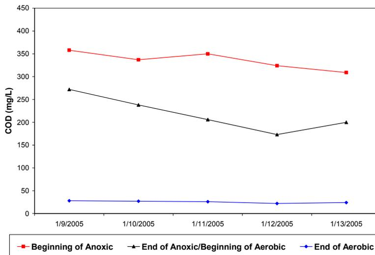
**Figure 4.13 Reactor 1, COD Measurements from 5-Day Period when Acclimated to Non-Colored Influent**
