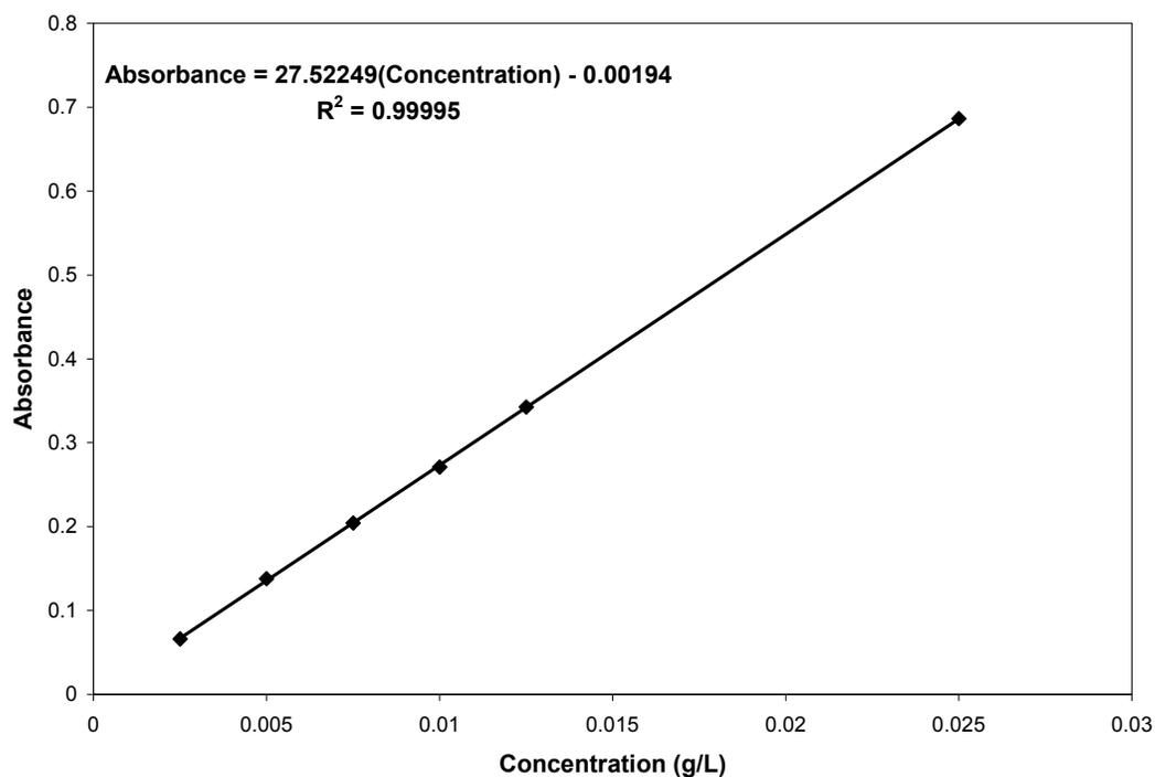
**Figure A-3 Equation for Determination of Dye Concentration in Solution for Reactive Black 5**
