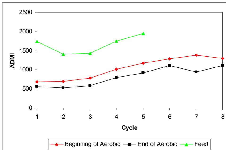
**Figure 4.49 Reactor 7 (Reactive Red 198 and Reactive Yellow 86), ADMI Data for Aerobic Control**
