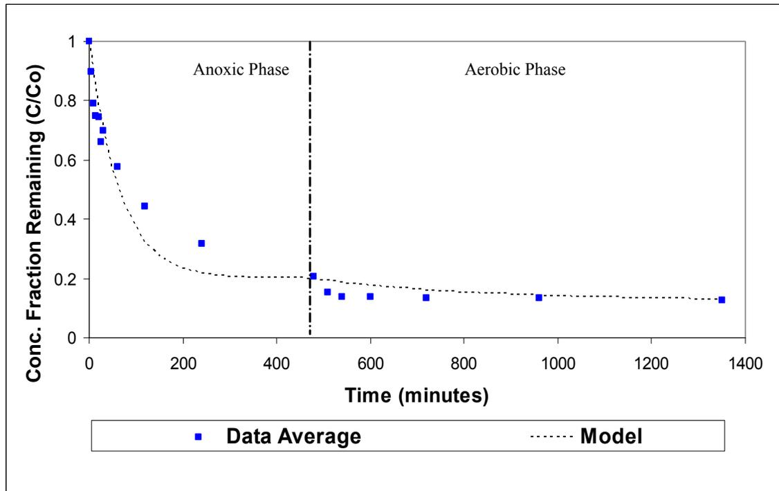
**Figure 4.28, Reactive Red 198, Model vs. Average Measured Data for Anoxic/Aerobic Reactor 1**
