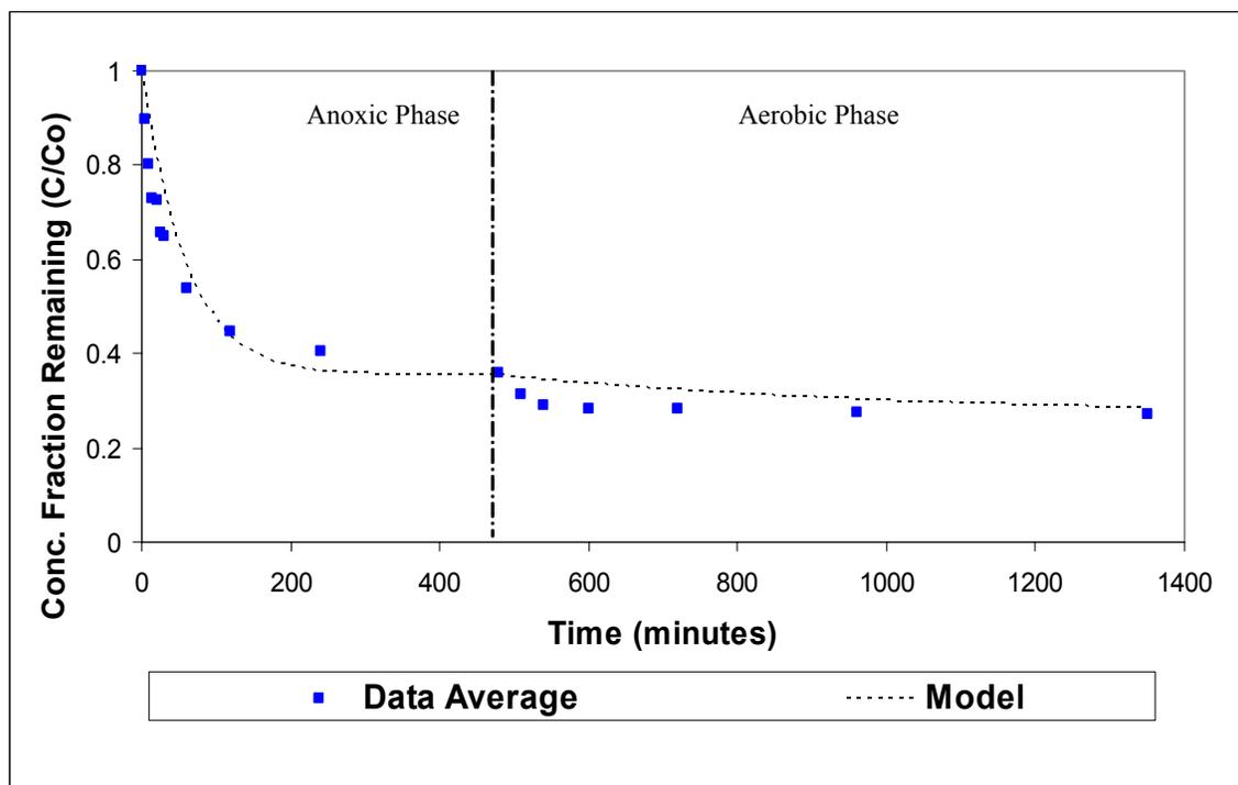
**Figure 4.36 Reactive Black 5, Model vs. Average Measured Data for Anoxic/Aerobic Reactor 2**
