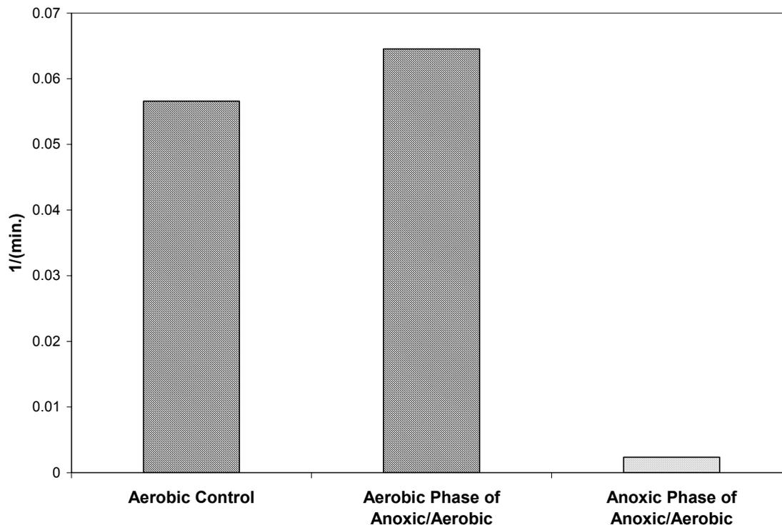
**Figure 4.17 Estimated Rate Constants for COD Removal, Anoxic/Aerobic Process vs. Aerobic Control**
