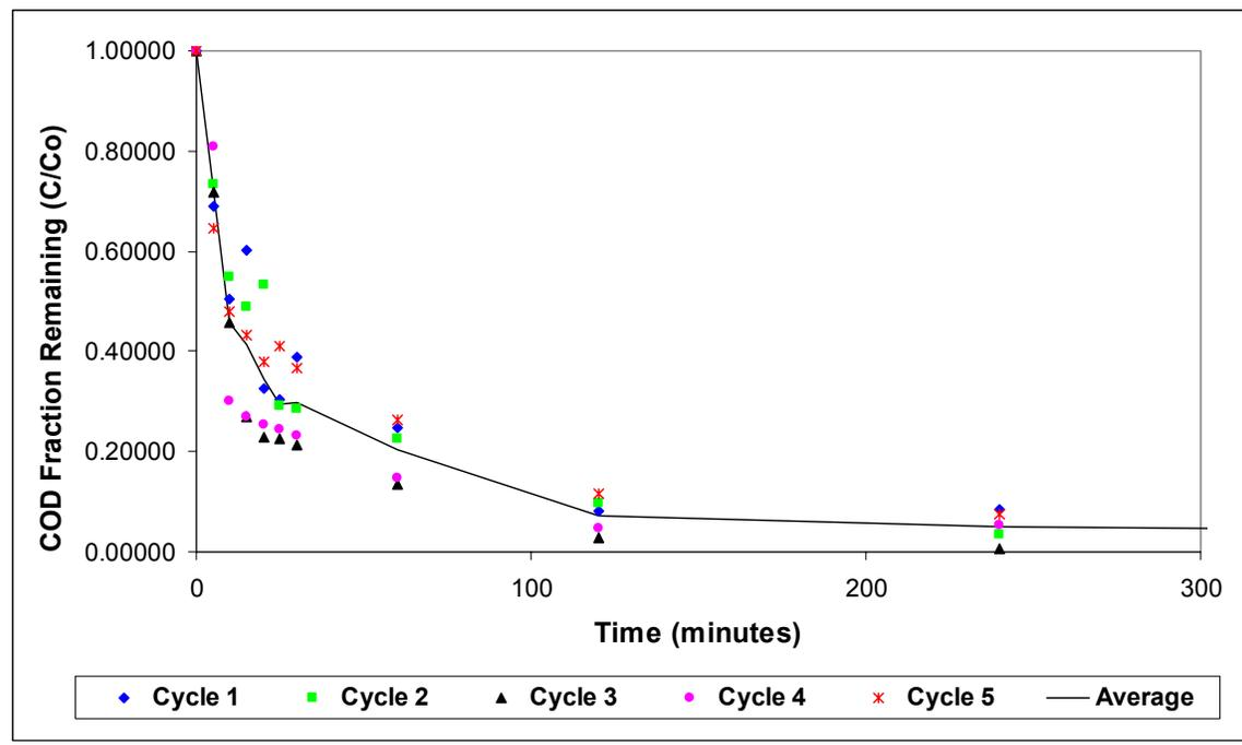
**Figure 4.6 Aerobic Control, COD Fraction Remaining vs. Time**
