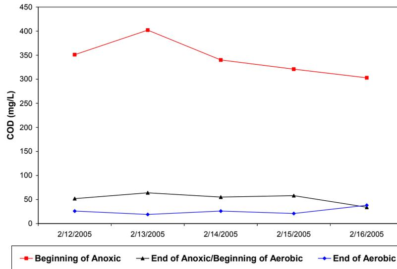
**Figure 4.14 Reactor 1, COD Measurements from 5-Day Period when Acclimated to Colored Influent**
