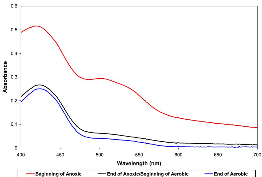
**Figure 4.51 Average Absorbance Spectra, Reactor 1**
