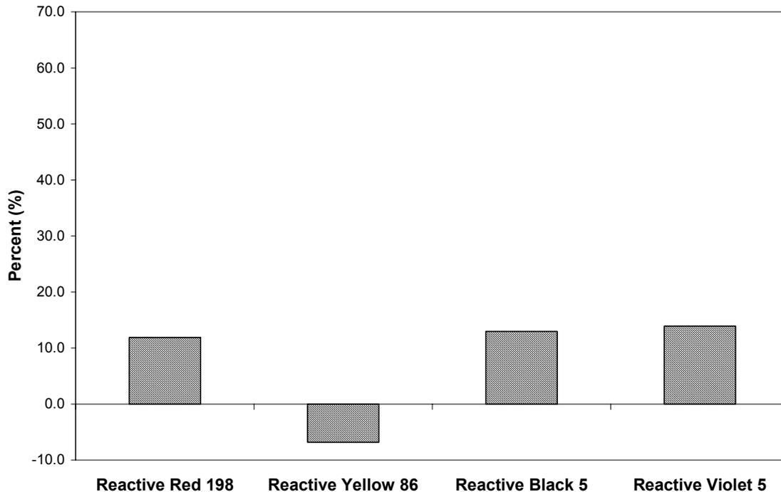
**Figure 4.68 Percent Color Removal by Aerobic Control, Concentration-Based**
