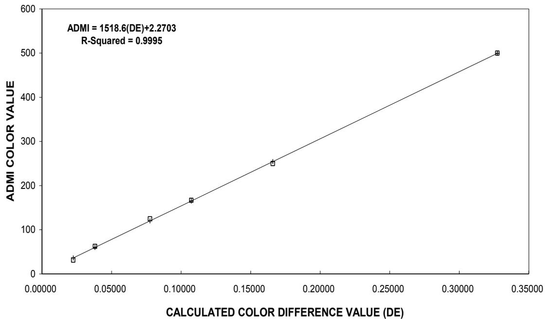
**Figure B-1 ADMI Calibration Curve**
