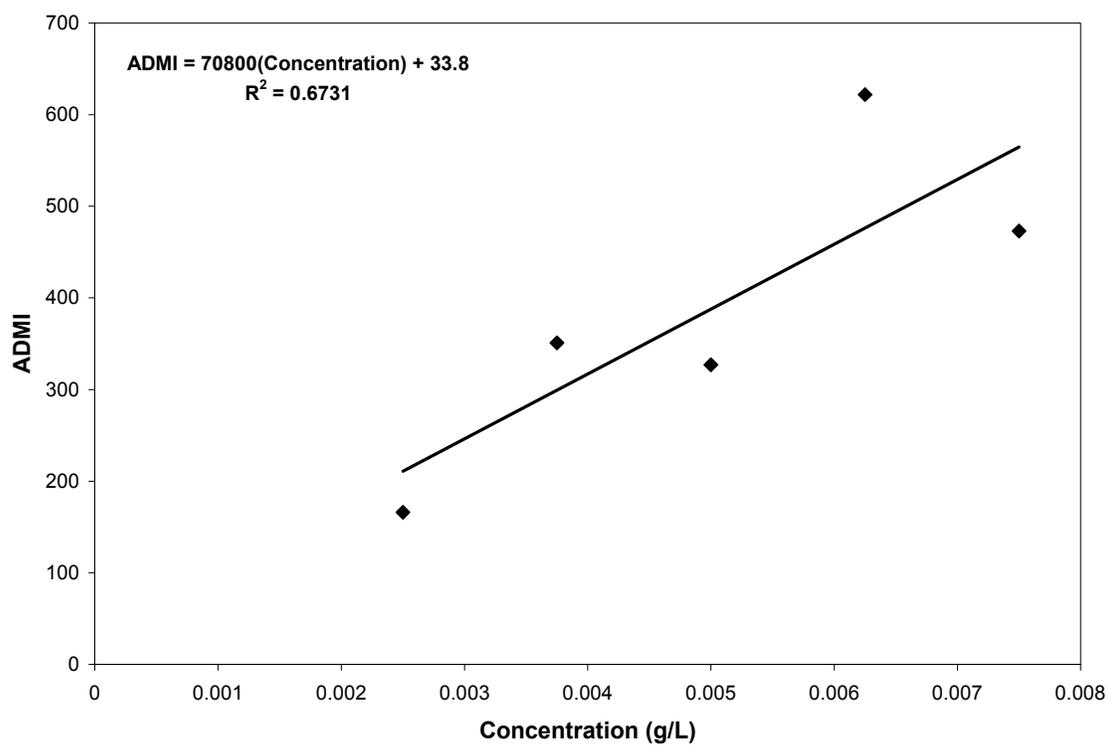
**Figure C-4 Correlation Between Dye Concentration and ADMI for Reactive Violet 5**
