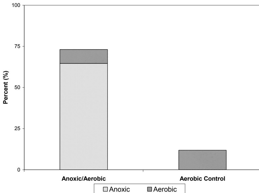
**Figure 4.30 Percent Color Removal (Concentration-Based) for Reactive Red 198, Anoxic/Aerobic vs. Aerobic Control**
