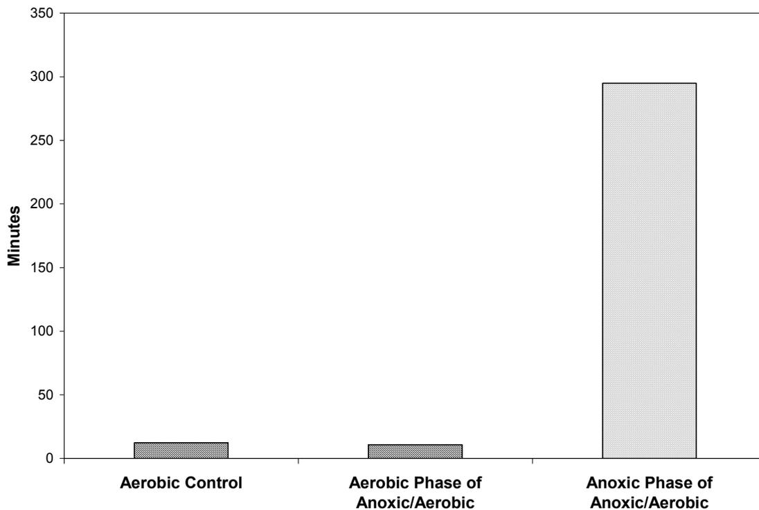
**Figure 4.18 Half-Life for COD Removal, Anoxic/Aerobic Process vs. Aerobic Control**
