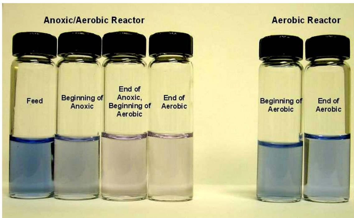
**Figure 4.55 Visual Comparison of Samples Containing Reactive Black 5**
