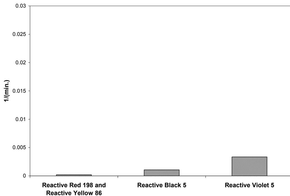
**Figure 4.64 Estimated Rate Constants for Aerobic Phase of Anoxic/Aerobic Process**
