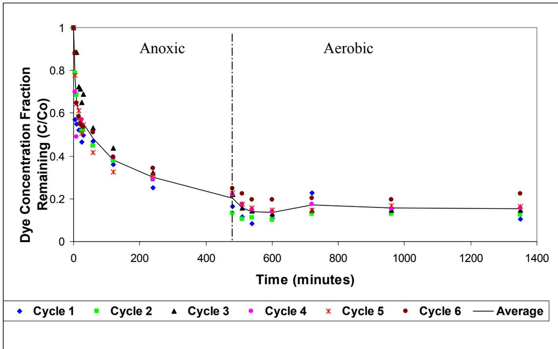
**Figure 4.39 Reactive Violet 5, Concentration Fraction Remaining vs. Time (Reactor 5)**
