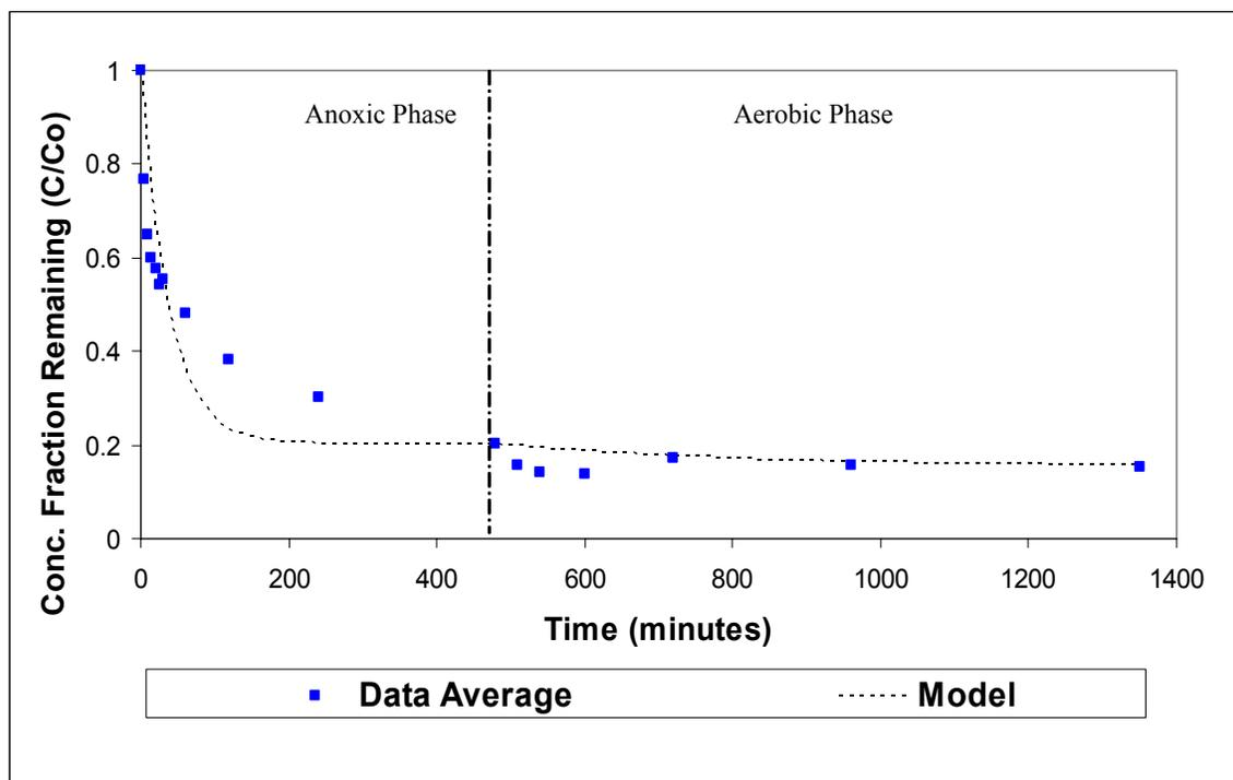
**Figure 4.40 Reactive Violet 5, Model vs. Average Measured Data for Anoxic/Aerobic Reactor 5**
