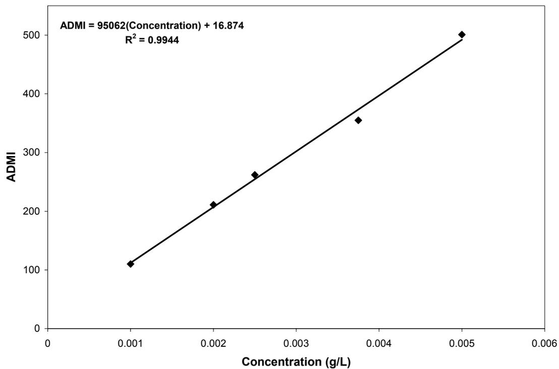
**Figure C-3 Correlation Between Dye Concentration and ADMI for Reactive Black 5**
