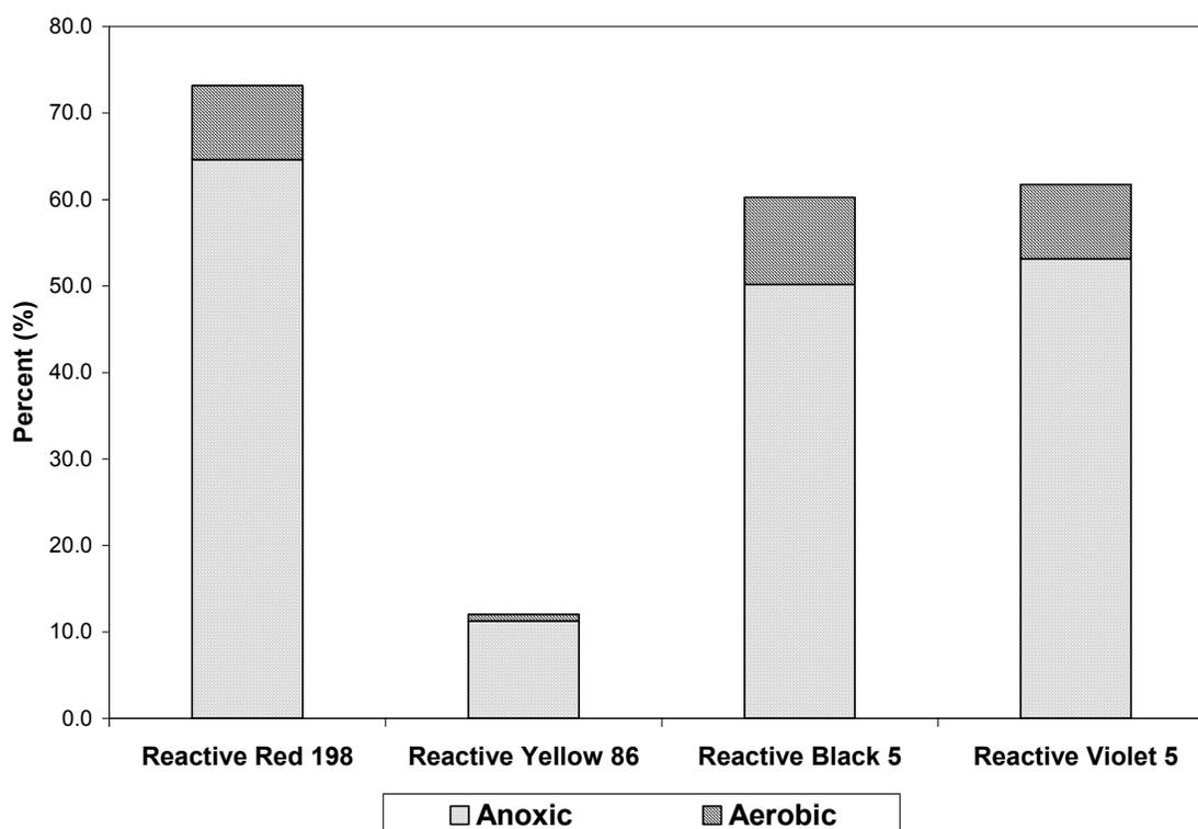
**Figure 4.67 Percent Color Removal by Anoxic/Aerobic Process, Concentration-Based**
