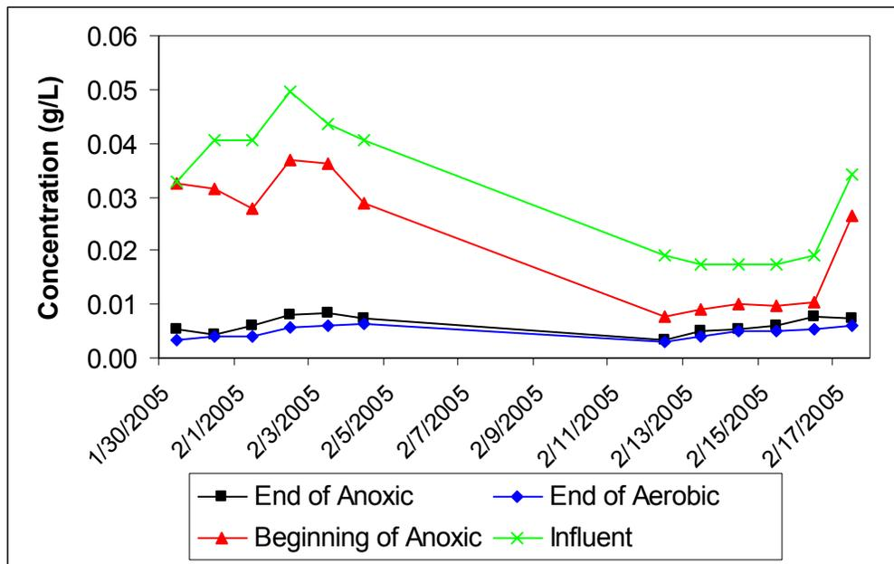
**Figure 4.26 Reactor 5, Concentration of Reactive Violet 5**
