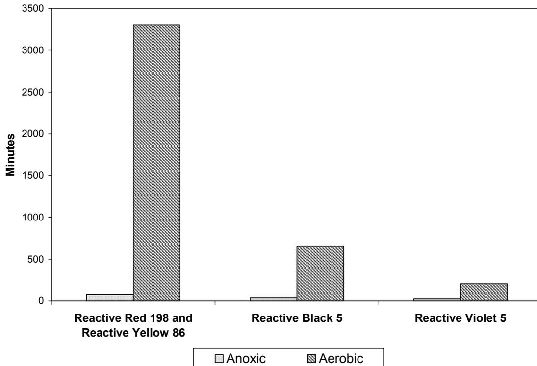
**Figure 4.65 Half-Life for ADMI-Based Color Removal, Anoxic Phase vs. Aerobic Phase of Anoxic/Aerobic Process**
