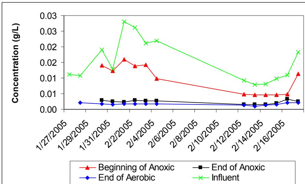
Figure 4.21 Reactor 1, Concentration of Reactive Red 198
