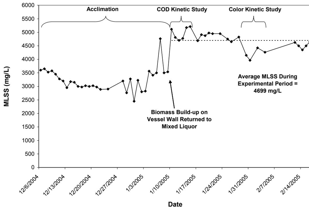
**Figure 4.2 MLSS vs. Time for Large Anoxic/Aerobic Reaction Vessel (Reactor 2)**
