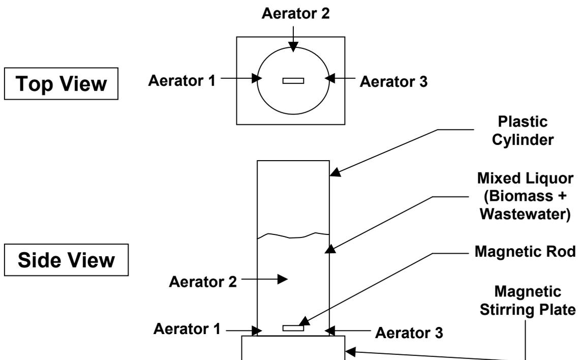
**Figure 3.1 Large Anoxic/Aerobic Reaction Vessel**
