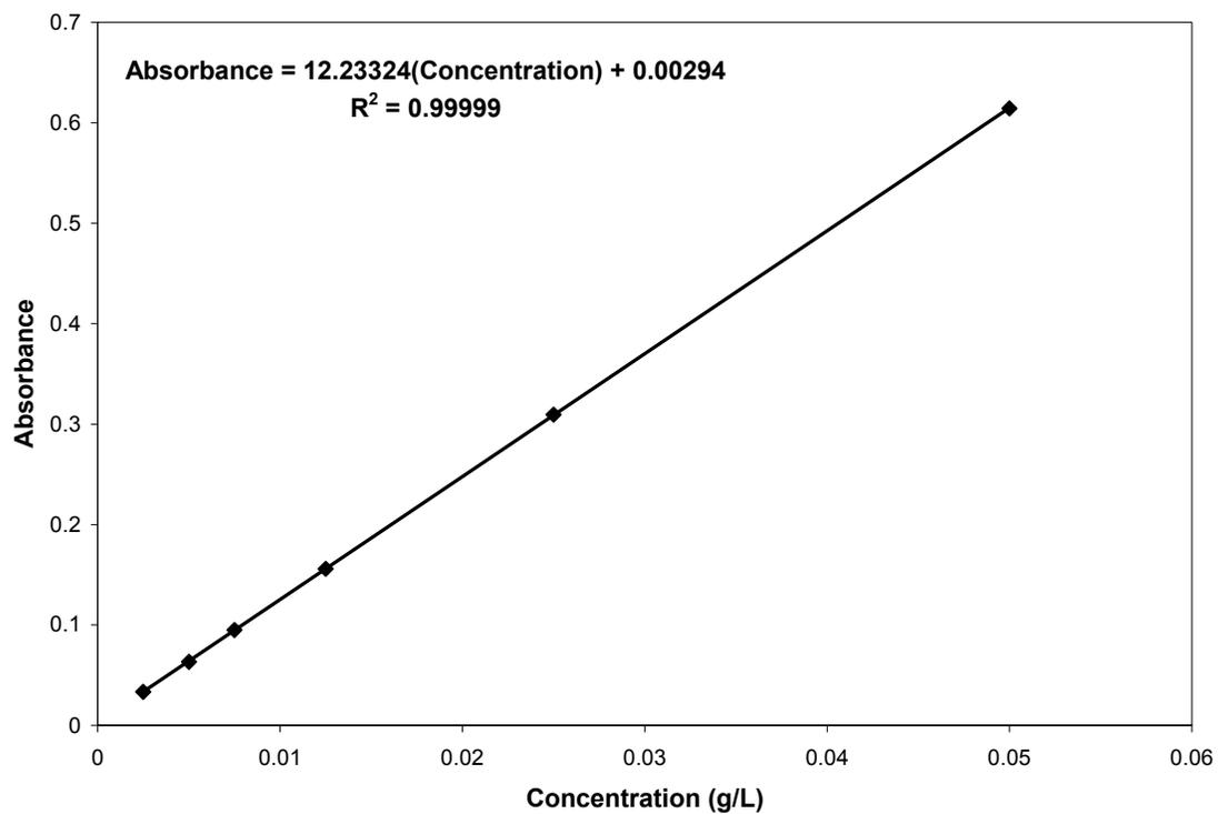
**Figure A-4 Equation for Determination of Dye Concentration in Solution for Reactive Violet 5**
