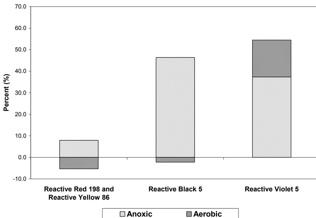
**Figure 4.69 Percent Color Removal by Anoxic/Aerobic Process, ADMI-Based**
