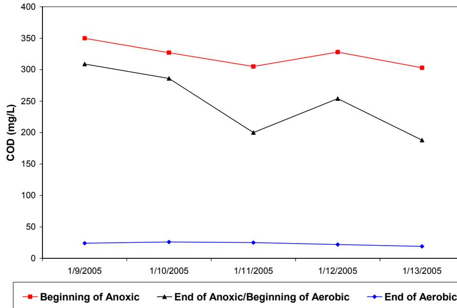
**Figure 4.15 Reactor 2, COD Measurements from 5-Day Period when Acclimated to Non-Colored Influent**
