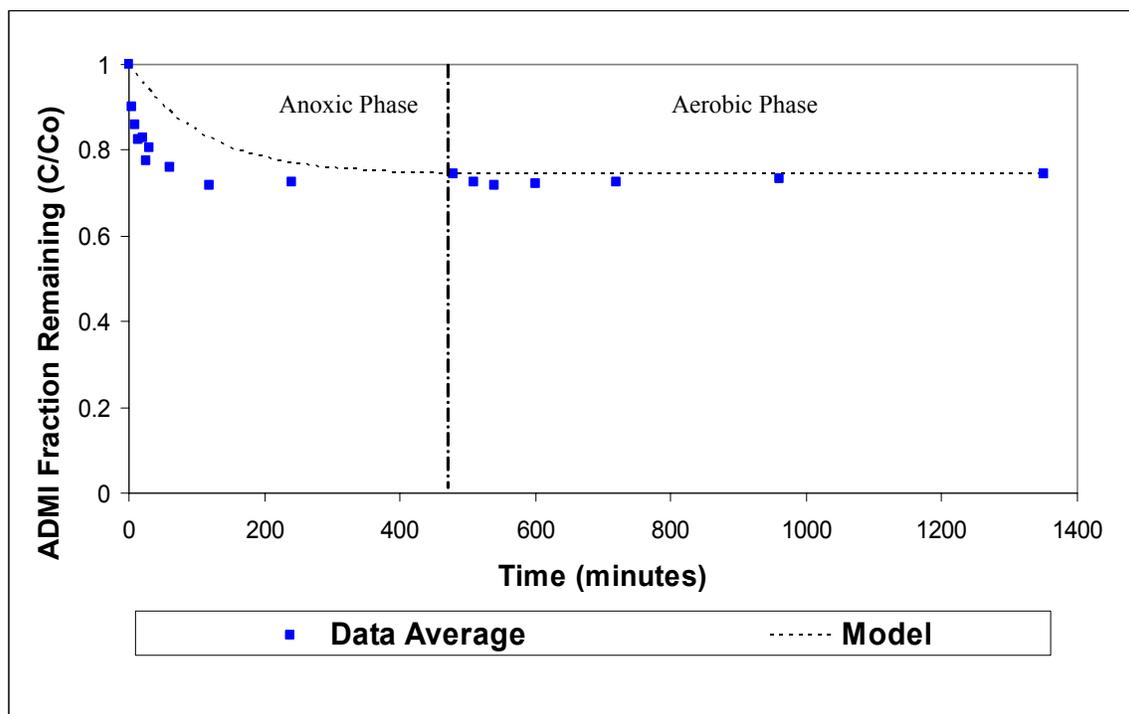
**Figure 4.48 Reactor 1, Model vs. Average Measured Data for Anoxic/Aerobic Process**
