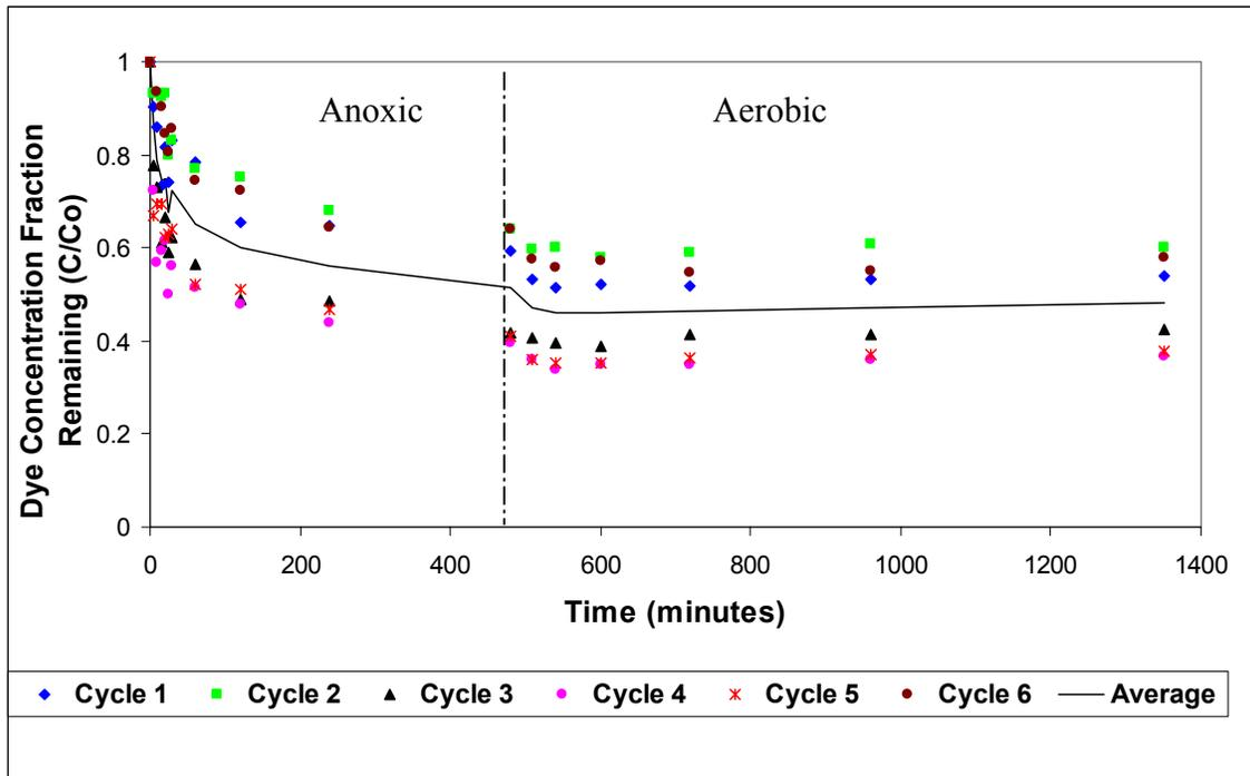
Figure 4.31 Reactive Yellow 86, Concentration Fraction Remaining vs. Time (Reactor 1)
