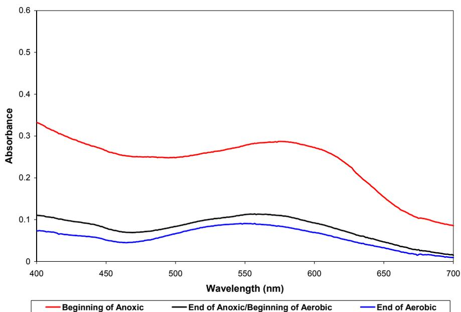
**Figure 4.56 Reactive Black 5, Average Absorbance Spectra, Reactor 2**
