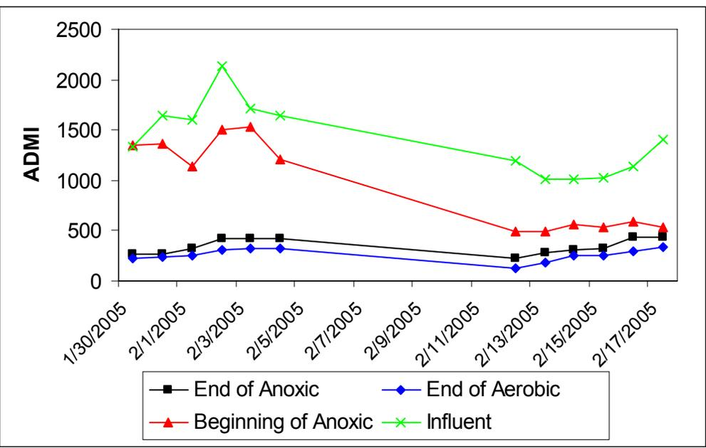
Figure 4.25 Reactor 5, ADMU
