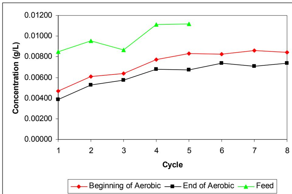
**Figure 4.37 Reactive Black 5, Concentration Data for Aerobic Control (Reactor 8)**
