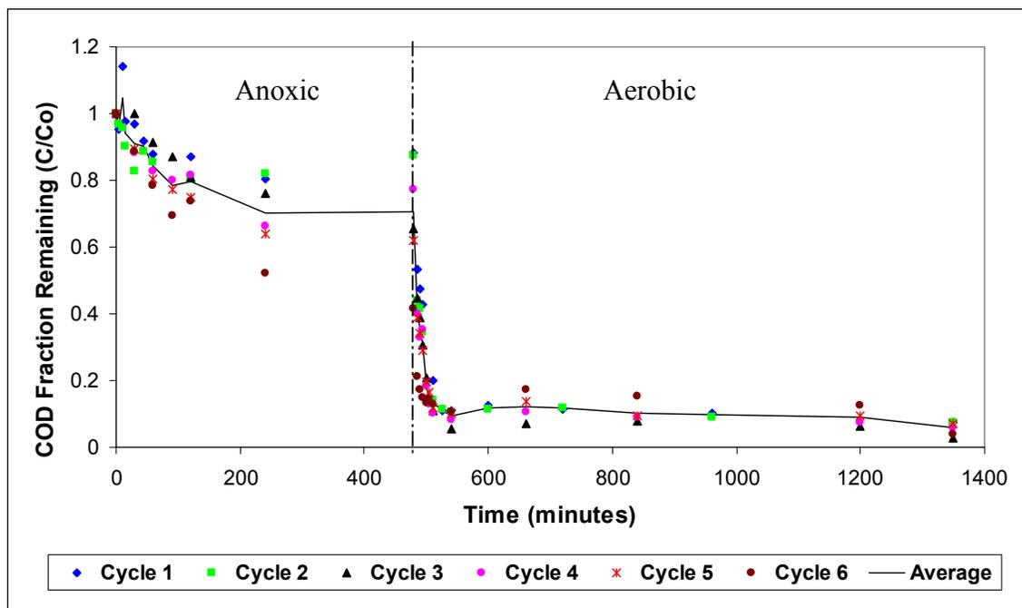
Figure 4.9 Anoxic/Aerobic Reactor 2, COD Fraction Remaining vs. Time
