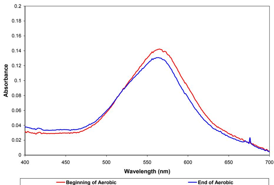
**Figure 4.60 Reactive Violet 5, Average Absorbency Spectra, Reactor 9**
