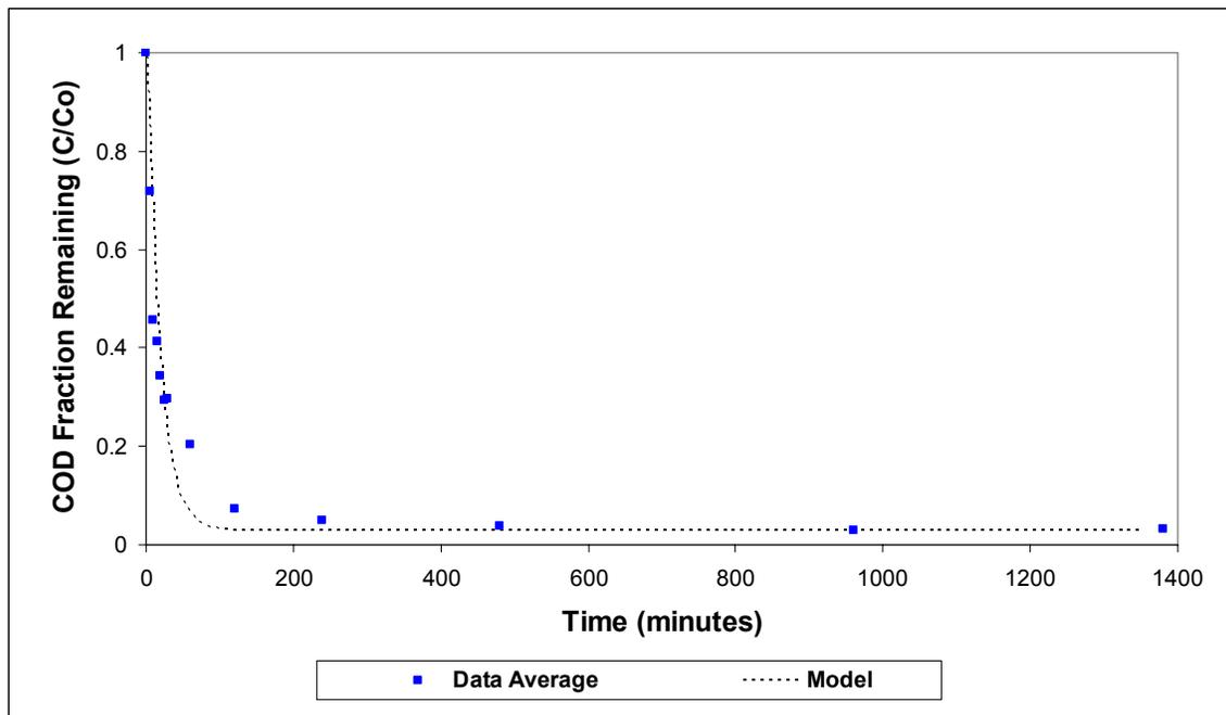
**Figure 4.7 Model vs. Average Measured Data for Aerobic Control**
