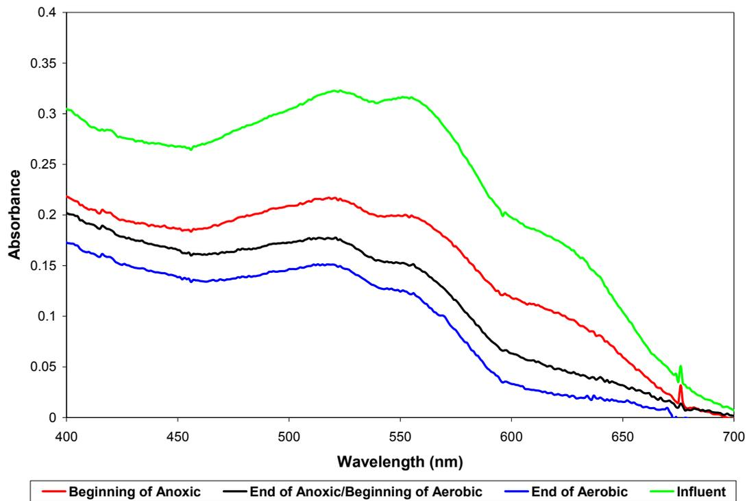
**Figure 6.1 Absorbance Spectra of Samples from Complex Textile Effluent**
