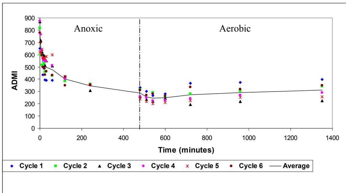
**Figure 4.52 Reactive Black 5, Adjusted ADMI vs. Time**
