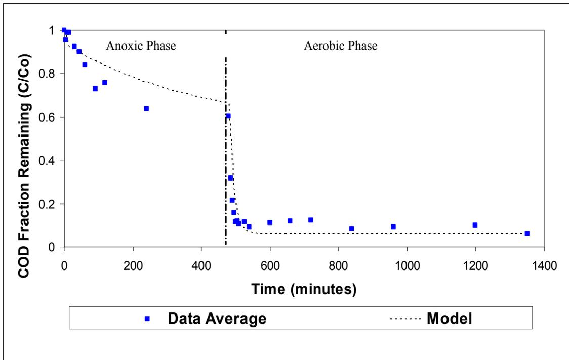
Figure 4.10 Model vs. Average Measured Data for Reactor 1
