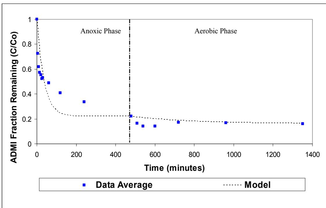
**Figure 4.58 Reactive Violet 5, Model vs. Average Measured Data for Anoxic/Aerobic Process**
