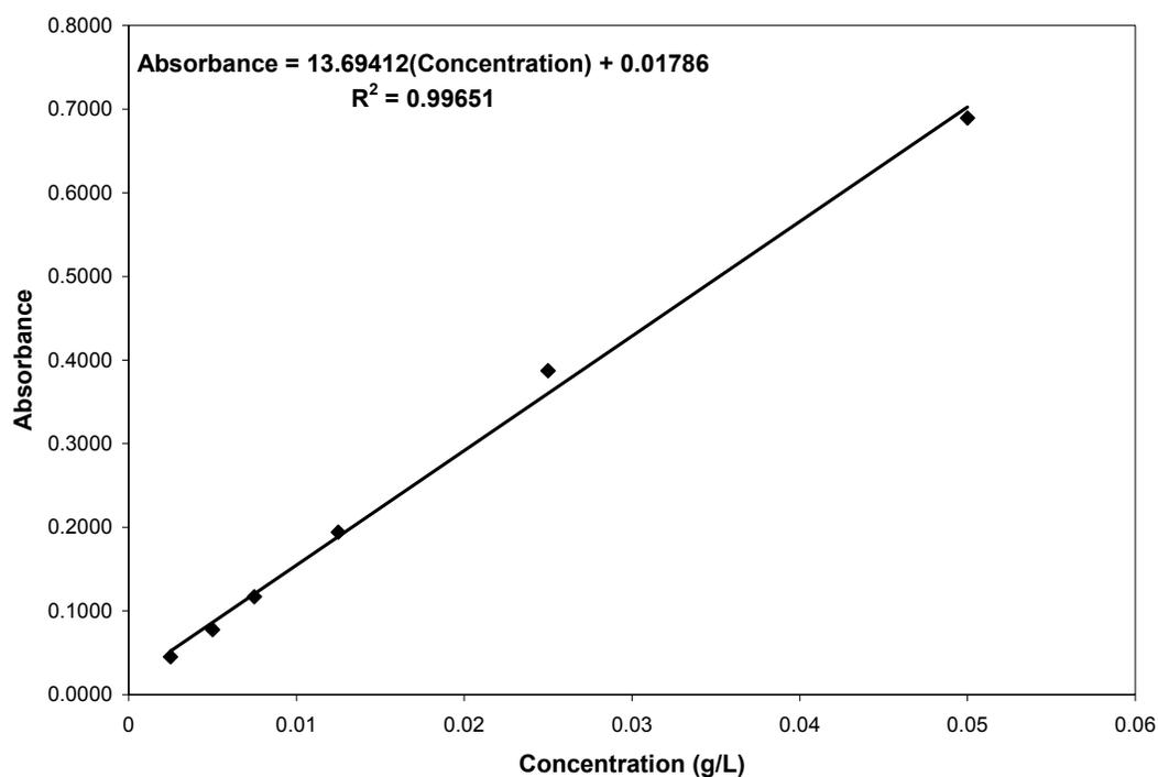
**Figure A-2 Equation for Determination of Dye Concentration in Solution for Reactive Yellow 86**
