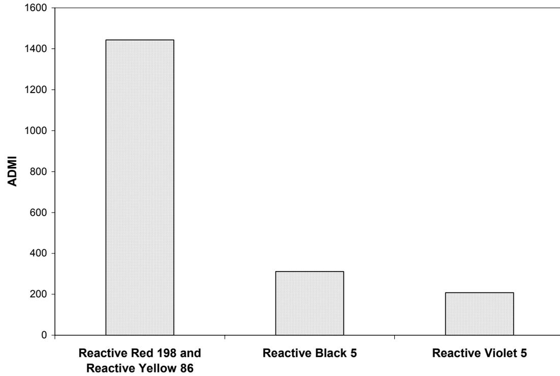
**Figure 4.66 Average Non-Degradable ADMI Remaining at End of Anoxic/Aerobic Process**
