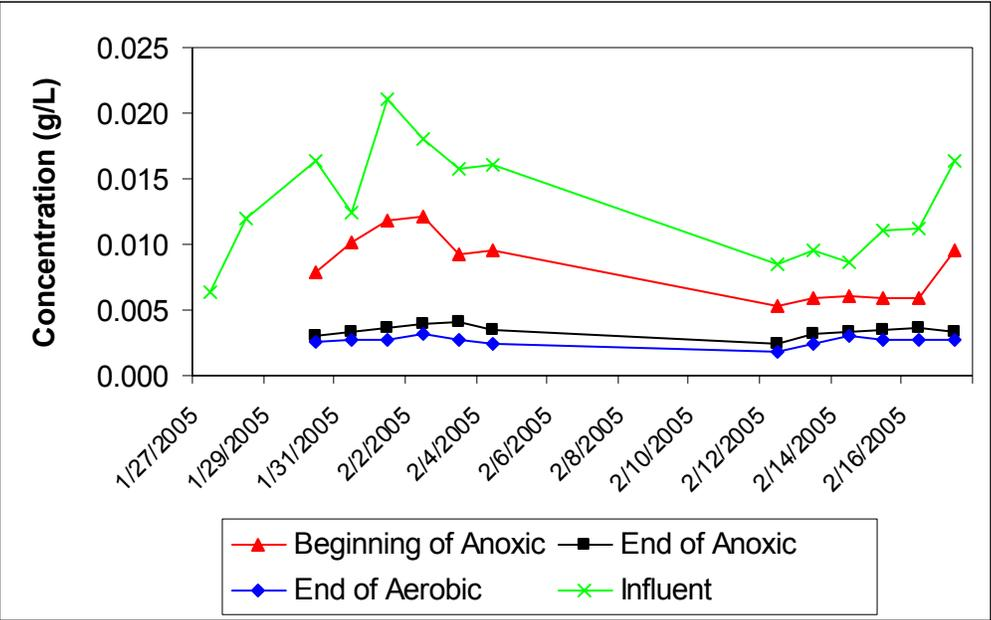
Figure 4.24 Reactor 2, Concentration of Reactive Black 5
