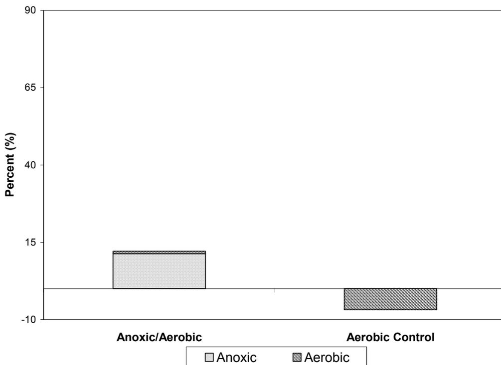
**Figure 4.34 Percent Color Removal (Concentration-Based) for Reactive Yellow 86, Anoxic/Aerobic vs. Aerobic Control**
