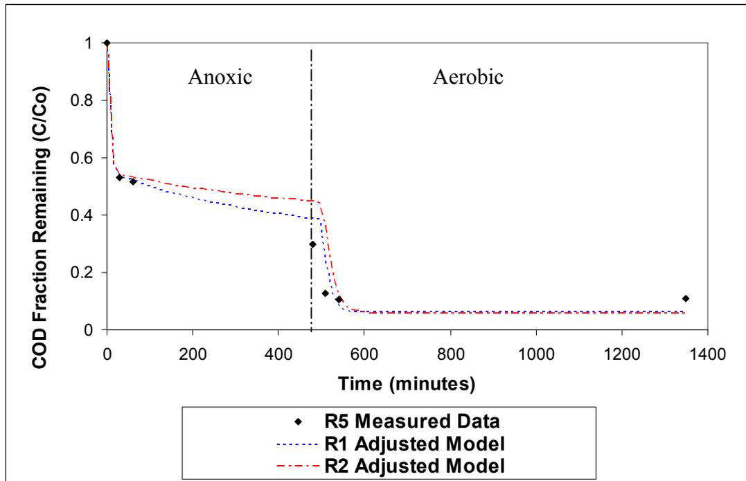
**Figure 4.12 Comparison of Adjusted Models to Reactor 5 Experimental Data**
