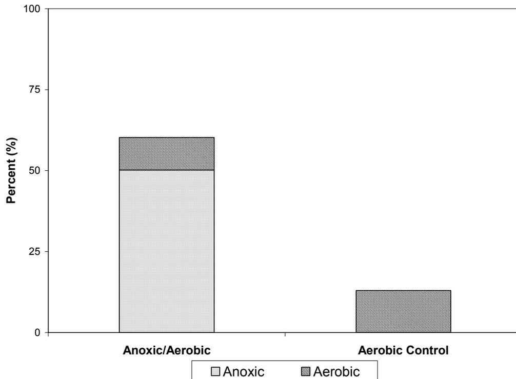
**Figure 4.38 Percent Color Removal (Concentration-Based) for Reactive Black 5, Anoxic/Aerobic vs. Aerobic Control**
