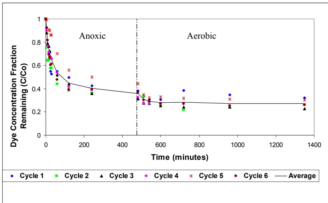
**Figure 4.35 Reactive Black 5, Concentration Fraction Remaining vs. Time (Reactor 2)**
