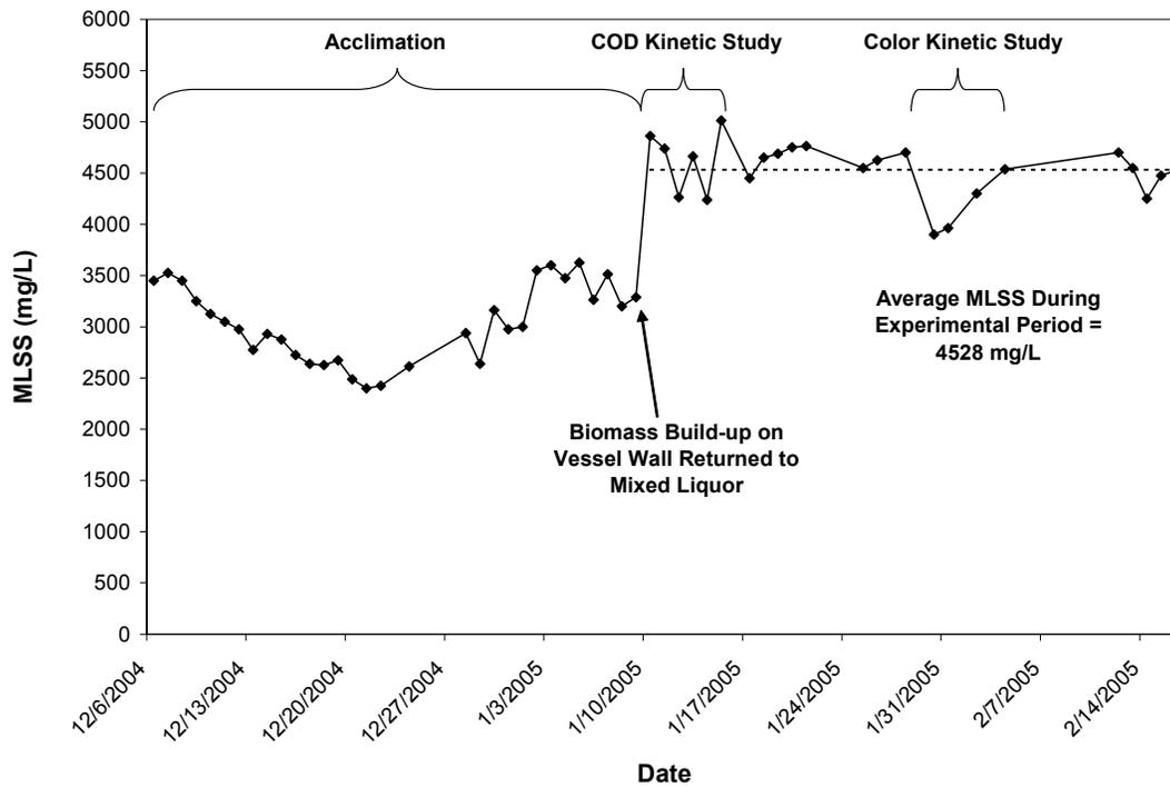
**Figure 4.1 MLSS vs. Time for Large Anoxic/Aerobic Reaction Vessel (Reactor 1)**
