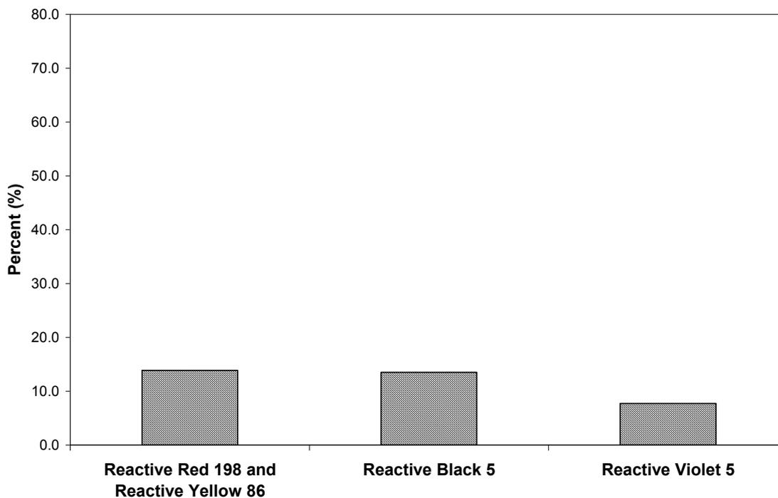
**Figure 4.70 Percent Color Removal by Aerobic Control, ADMI-Based**
