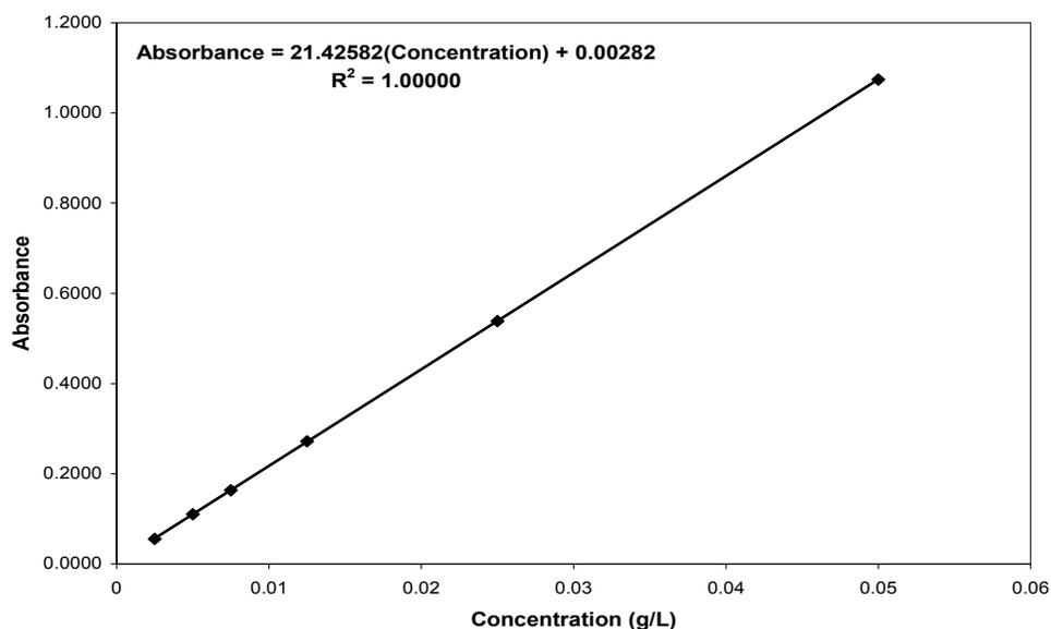
**Figure A-1 Equation for Determination of Dye Concentration in Solution for Reactive Red 198**
