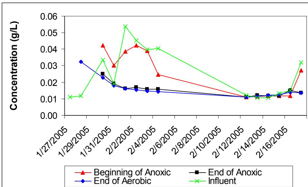
Figure 4.22 Reactor 1, Concentration of Reactive Yellow 86
