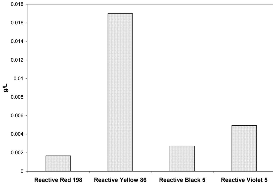
**Figure 4.46 Average Non-Degradable Dye Remaining at End of Anoxic/Aerobic Process**
