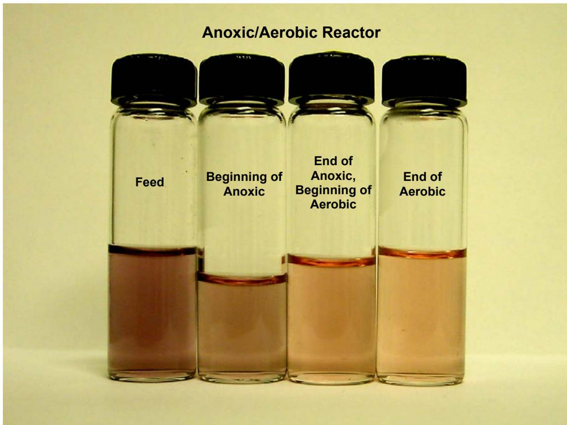
**Figure 6.2 Samples from Complex Effluent**
