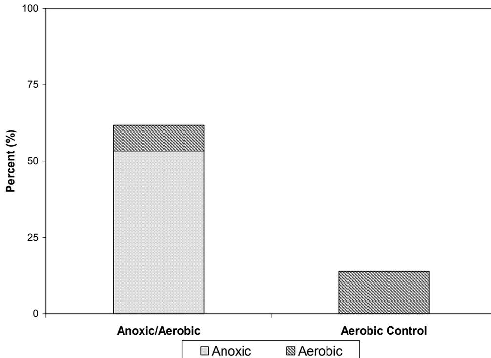
**Figure 4.42 Percent Color Removal (Concentration-Based) for Reactive Violet 5, Anoxic/Aerobic vs. Aerobic Control**
