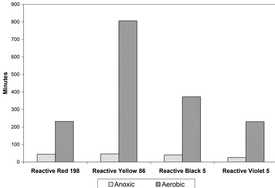
**Figure 4.45 Half-Life for Concentration-Based Color Removal, Anoxic Phase vs. Aerobic Phase of Anoxic/Aerobic Process**
