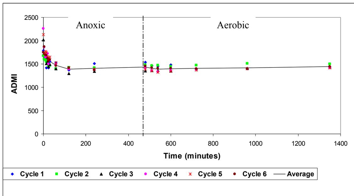
**Figure 4.47 Reactor 1, Adjusted ADMI vs. Time (Reactive Red 198 and Reactive Yellow 86)**
