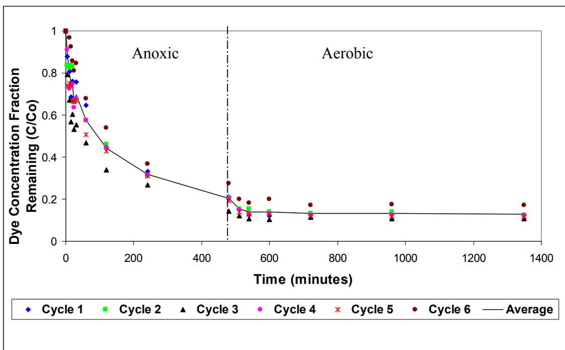
**Figure 4.27 Reactive Red 198, Concentration Fraction Remaining vs. Time (Reactor 1)**
