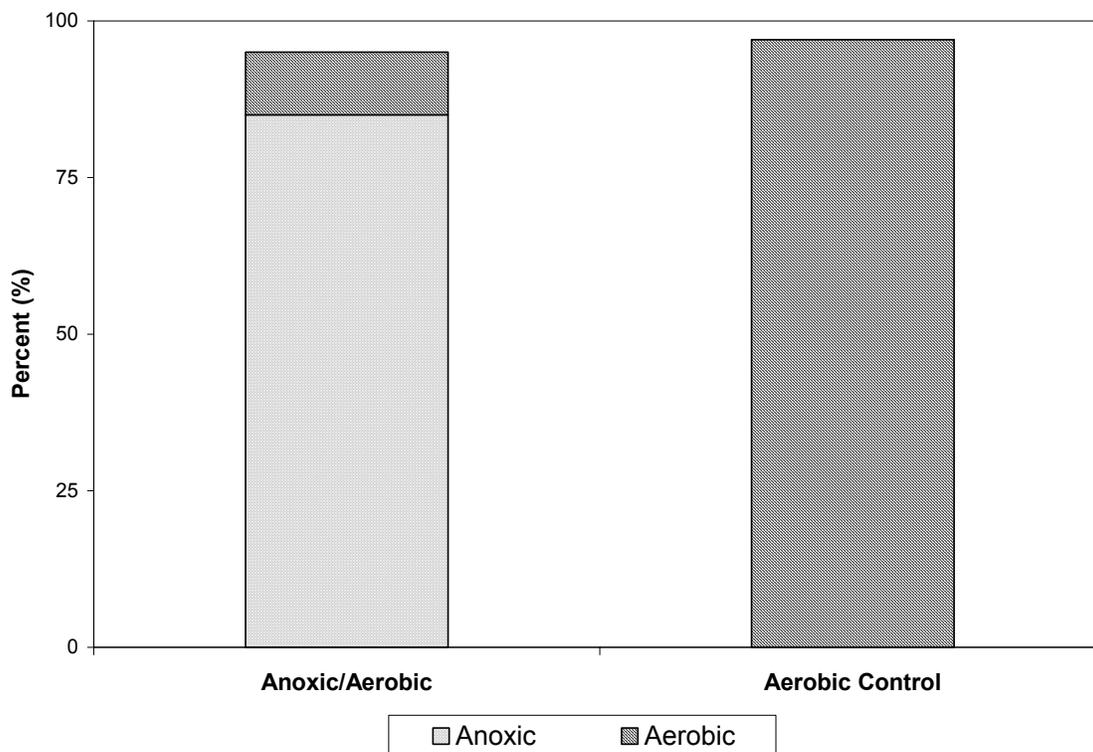
**Figure 4.19 Percent COD Removal for Anoxic/Aerobic Process vs. Aerobic Control**
