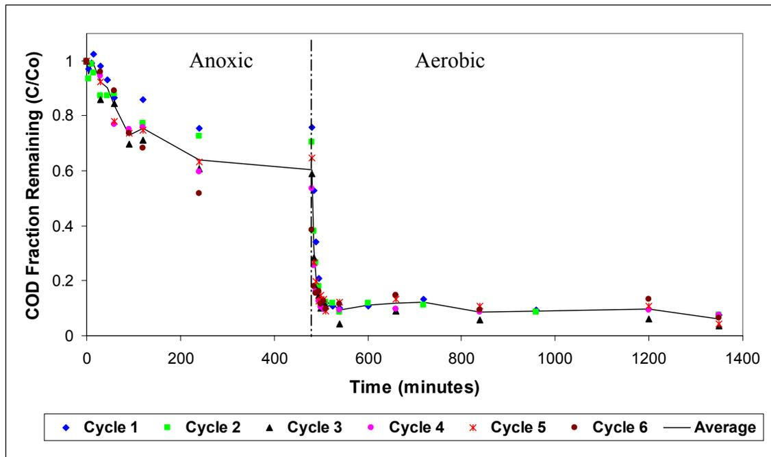
Figure 4.8 Anoxic/Aerobic Reactor 1, COD Fraction Remaining vs. Time
