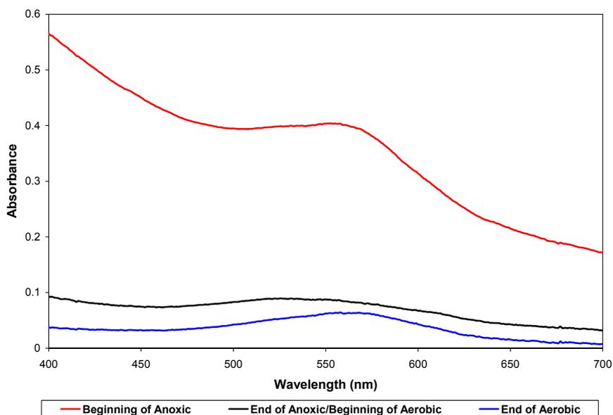
**Figure 4.62 Reactive Violet 5, Average Absorbance Spectra, Reactor 5**
