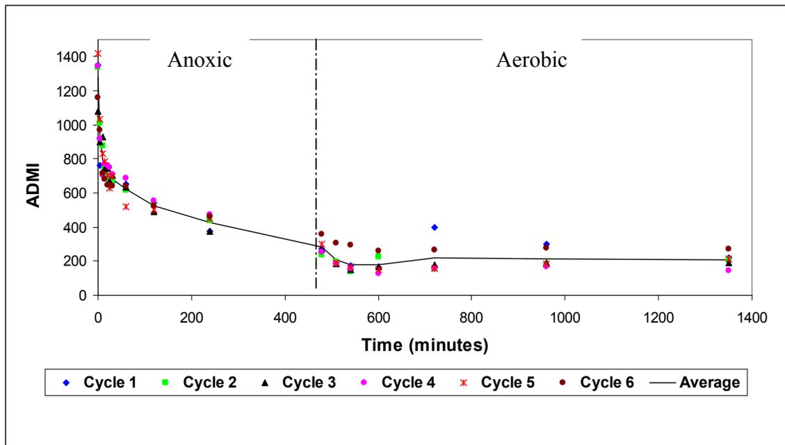
**Figure 4.57 Reactive Violet 5, Adjusted ADM I vs. Time**
