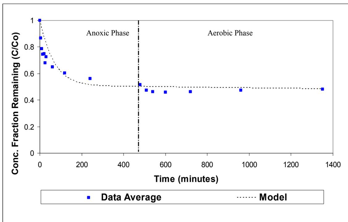
**Figure 4.32, Reactive Yellow 86, Model vs. Average Measured Data for Anoxic/Aerobic Reactor 1**
