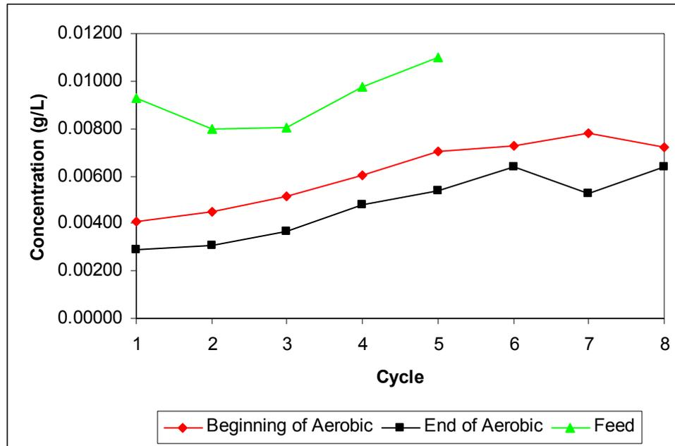
**Figure 4.29 Reactive Red 198, Concentration Data for Aerobic Control (Reactor 7)**
