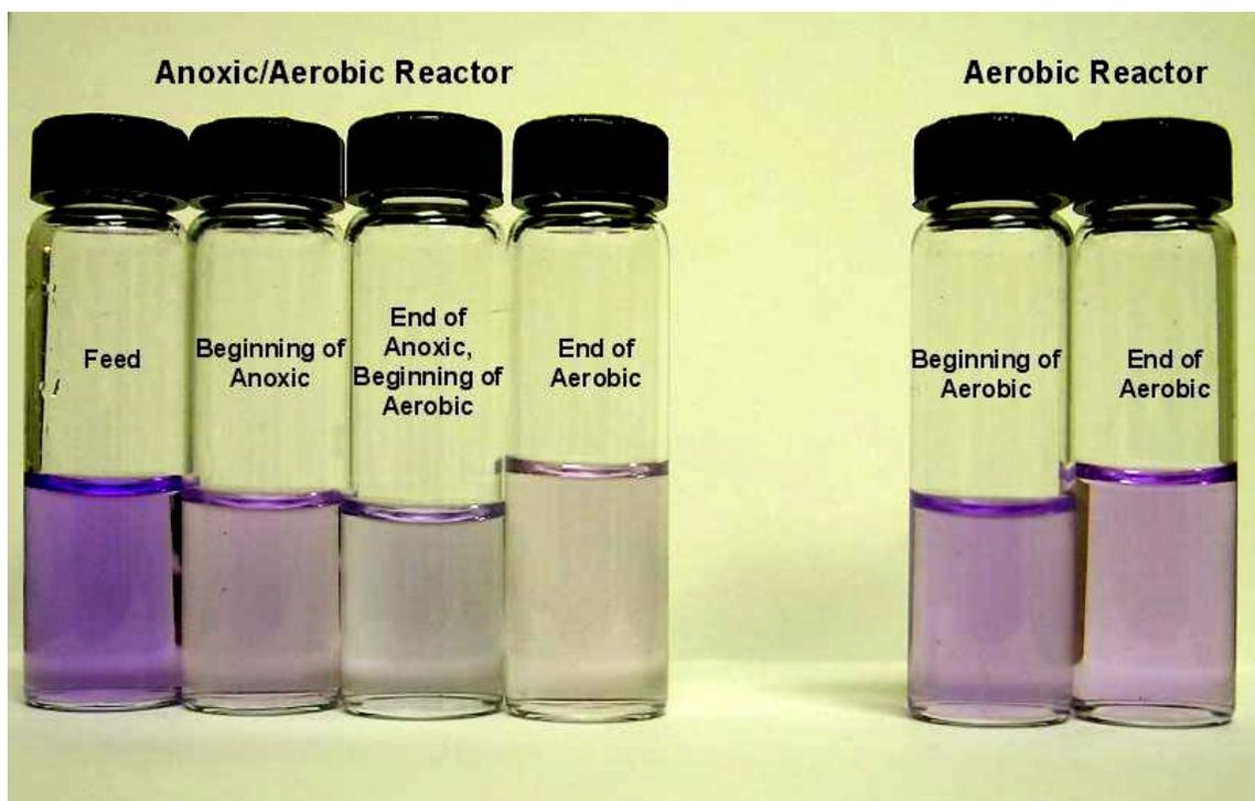
**Figure 4.61 Visual Comparison of Samples Containing Reactive Violet 5**
