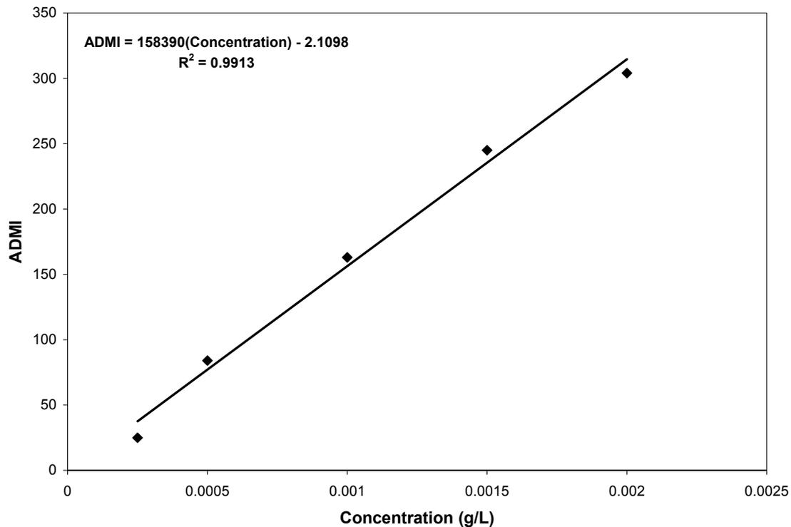
Figure C-1 Correlation Between Dye Concentration and ADMI for Reactive Red 198
