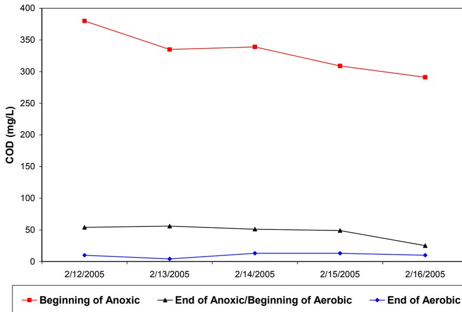
**Figure 4.16 Reactor 2, COD Measurements from 5-Day Period when Acclimated to Colored Influent**
