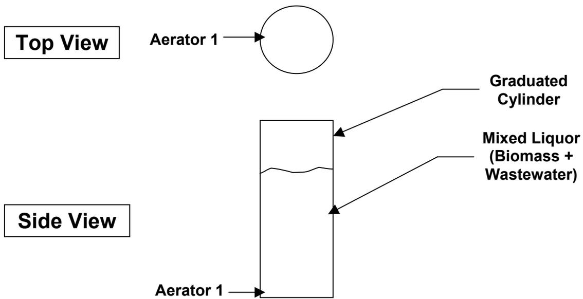
**Figure 3.3 Aerobic Control Vessel**
