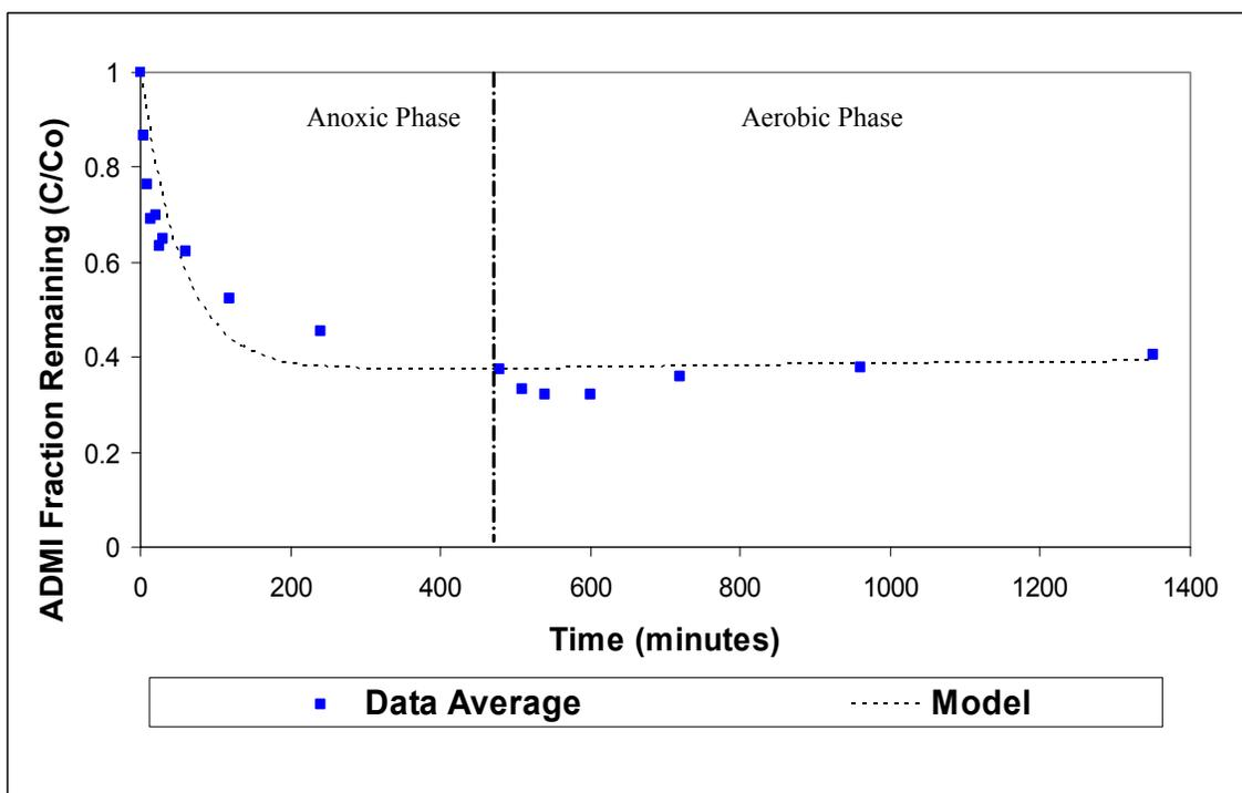
**Figure 4.53 Reactive Black 5, Model vs. Average Measured Data for Anoxic/Aerobic Process**
