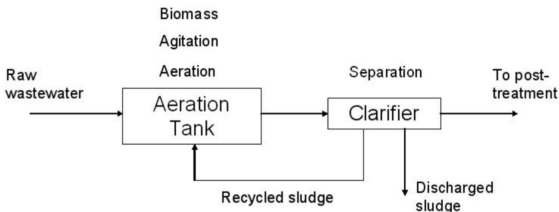
**Figure 1.6 Activated Sludge Process**
