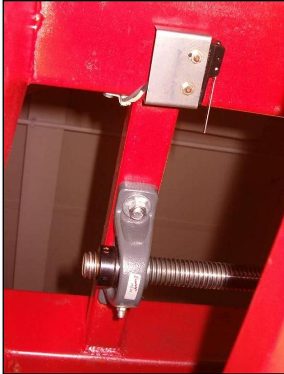
Figure 3.5: Eccentric lock pillow block bearing.
