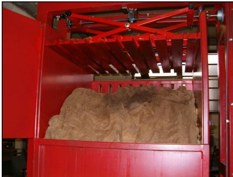
Figure 3.8: Plunger fully retracted.
