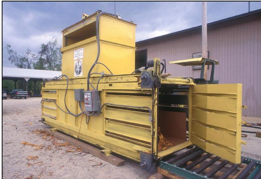
Figure 1.1: A single stroke, horizontal baler.
