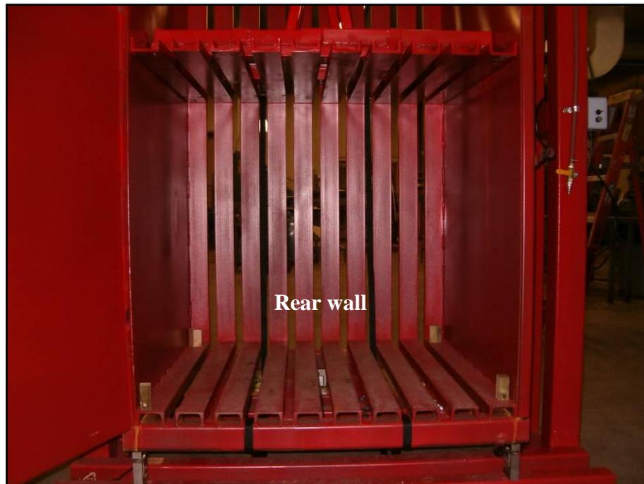
Figure 3.2: Baling chamber floor and rear wall C-channel.
