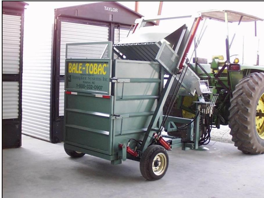
Figure 1.2: A multiple stroke, vertical baler.
