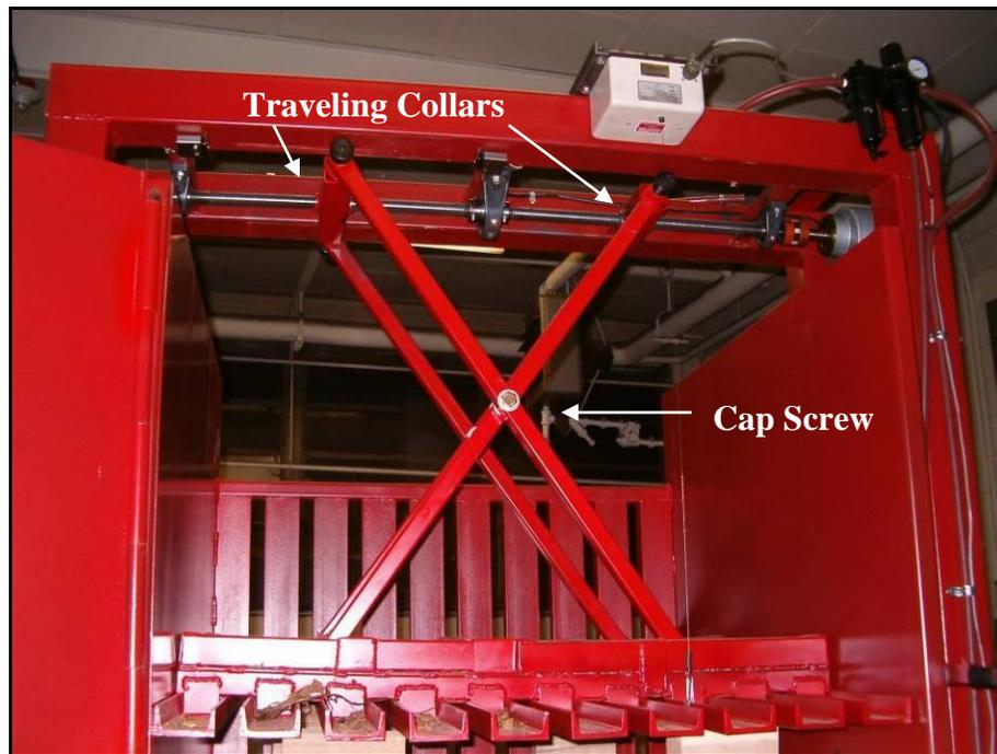
Figure 3.3: Double scissor press
