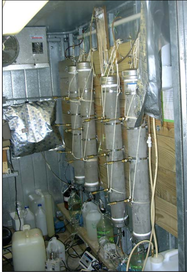
Figure 1: Photograph of 10 cm by 100 cm long continuous flow columns.
