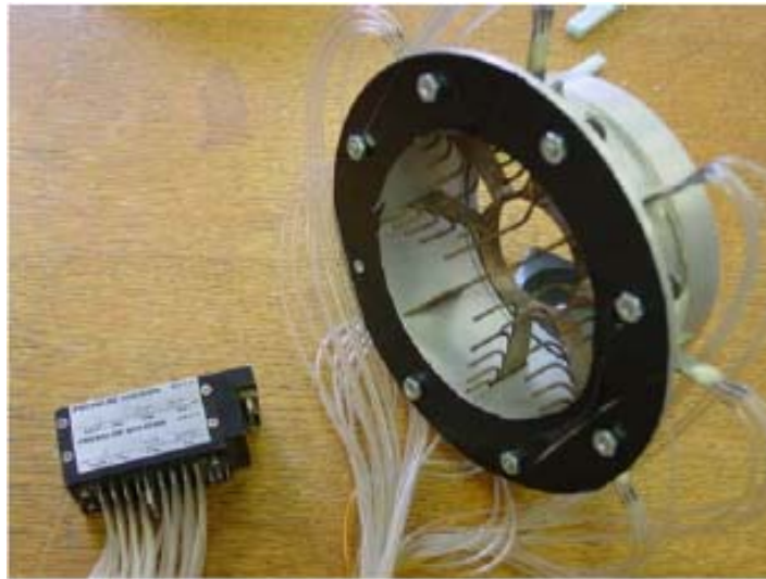
Figure 2-4: PSI ESP Pressure Transducer and Inlet Rake 5
