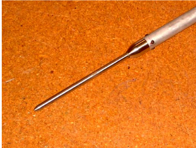
Figure 2-6: NCSU Pitot-Static Probe
