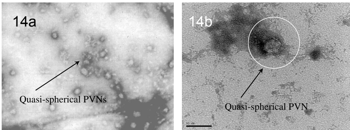
Figure 14: TEM images of CBD PVN – Trial 1. (a) 63,000x magnification (b) 140,000x magnification
