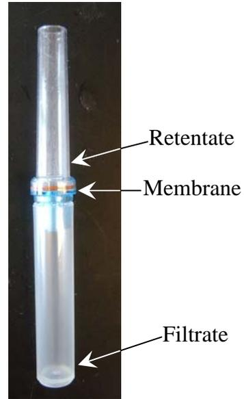
Figure 8: Centricon 100,000 MWCO centrifugation filter.
