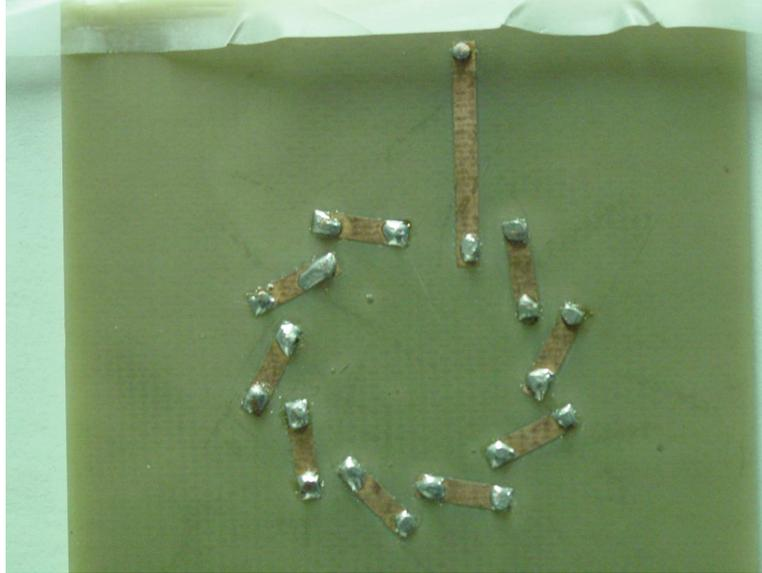
Figure 4.18: Bottom view of the toroidal structure with approximately equal angles between each pair of top and bottom metal strips.
