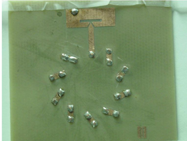
Figure 4.17: Top view of the toroidal structure with approximately equal angles between each pair of top and bottom metal strips.
