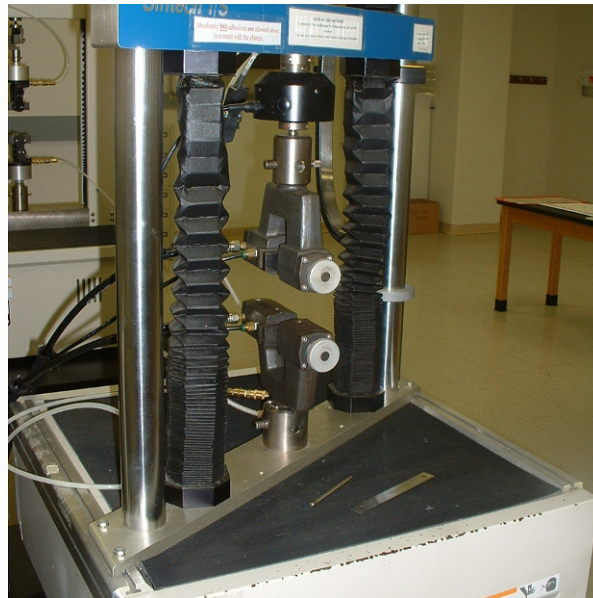
Figure 3-6 Sintech Tear Tester
