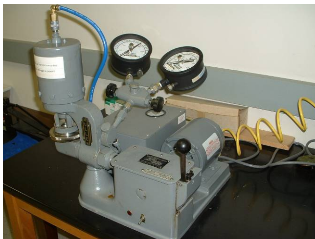
Figure 3-7 Mullen Burst Tester
