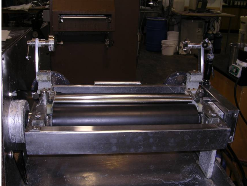
Figure 3-1 NCSU Werner Mathis AG Padder- Rolls Vertical and Flushed
