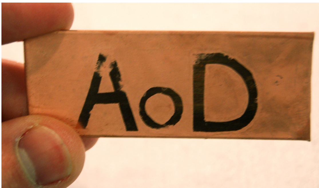
Figure 6.7. Bulk copper sample following “Acid on Demand” etching.
