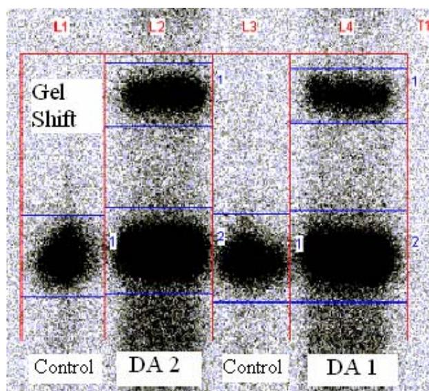
**Figure 4.3.** 6% denaturing polyacrylamide, 8.3 M Urea gel for Diels-Alder cycloaddition product analysis. The lower mobility bands, gel shifts correspond to the Diels-Alder products, which were excised and brought forward to next cycle. The higher mobility bands were ligation products, which were also the unreacted Diels-Alder products.
