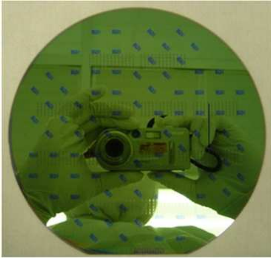
Figure 3.6: Nanowire patterns created in 100 and 110 orientations using the ASML scanner
