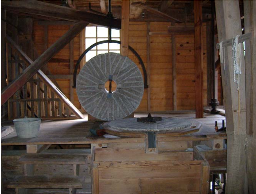
Figure 1: Quartzite millstones found inside Yates Mill. Notice the pattern carved into the stones. This pattern does the sheering, or cutting, of the corn kernels during the grinding process. When set up to grind, the upper, or runner stone, balances on the driving bar above the bottom, or bed stone. A case that is placed over the stones before the grinding process begins forces the meal to collect in the bin in the front of the picture.
