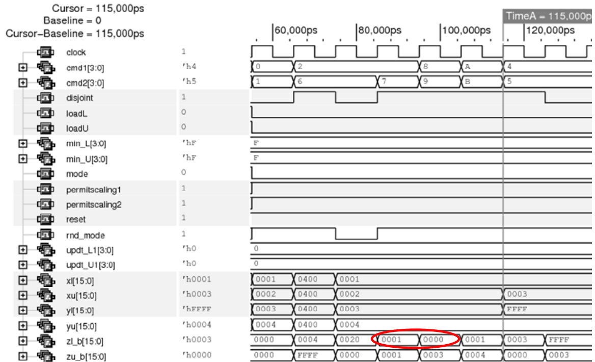
Figure 6.4: Independent pointwise operation in the interval ALU
