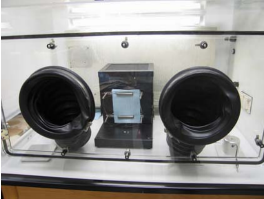
Figure 32: The charge decay test instrument –ETS Model 406D-
