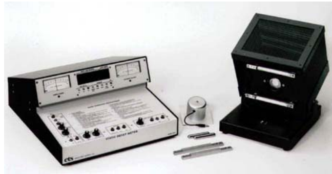
Figure 19: Charge Decay Instrument, ETS, Model 406D
