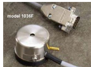
Figure 37: The probe that was used, Monroe Electronics, model 1036F
