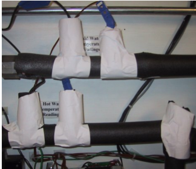
Figure 4.4 Most of the Additional Insulation Applied to House Pipe Sections
