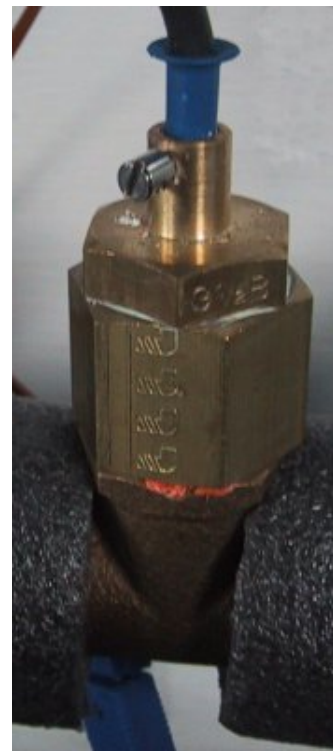
Figure 2.5 Temperature Probe Assembly
