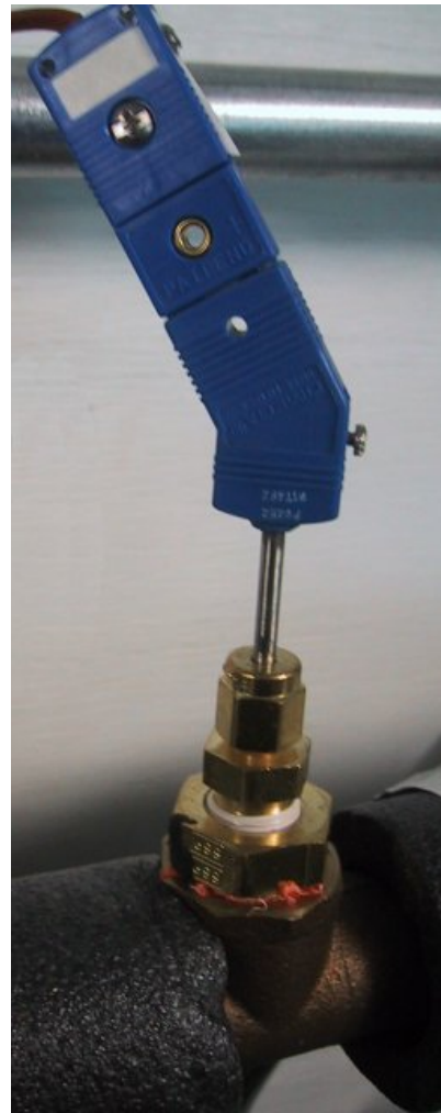
Figure 2.8 Pipe Thermocouple
