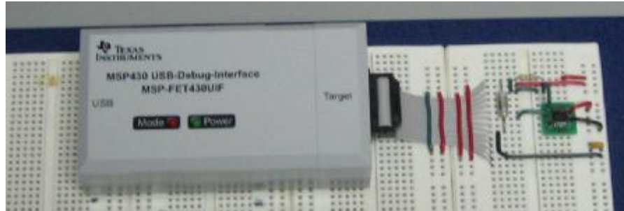
Figure 3.9: On-board programming setup.
