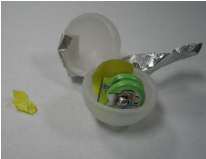
Figure 4.4: A sensor packaged in 1" sphere.
