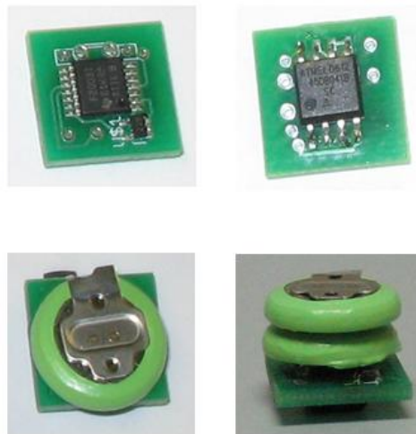
Figure 3.8: Off-the-shelf temperature sensor (left top: front view w/o battery; left bottom: front view with batteries; right top: back view; right bottom: horizontal view with two batteries).
