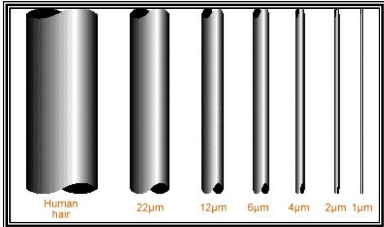
**Figure 6: Metallic Fiber Diameters Compared to Human Hair**
