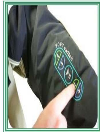
**Figure 24: Sleeve Integrated Textile Keypad**
