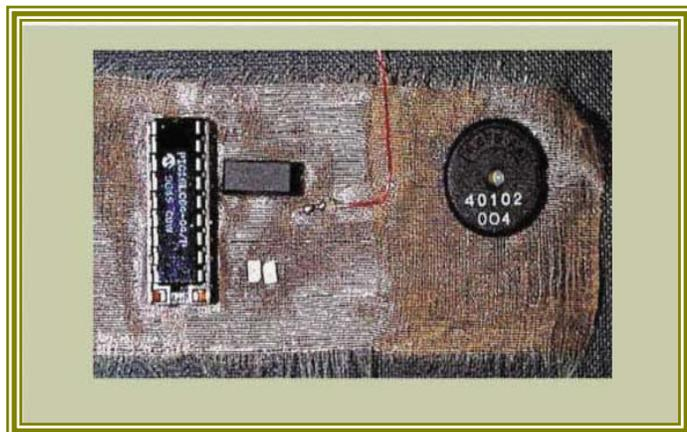
**Figure 14: Micro Controller Circuit on Silk Organza**
