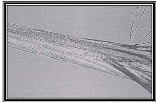
**Figure 10: 100% Stainless Steel Thread**
