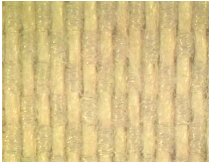
Figure 5. 22: Optical image of woven finished elastomeric fabric (In-loom fabric tightness: 0.64, 89 EPI x 42 PPI) with 152D filling) Magnification 25x
