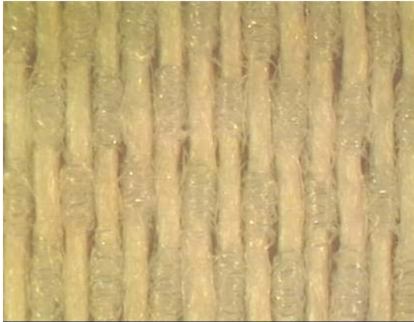
Figure 5. 21: Optical image of woven finished elastomeric fabric (In-loom fabric tightness: 0.57, 89 EPI x30 PPI) with 152D filling) Magnification 25x
