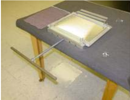
4.3a) Fabric sample and Straining Device
