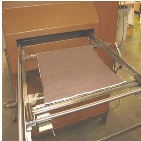
Figure 4. 11: Fabric pinned to the frame enters the heat-setting unit
