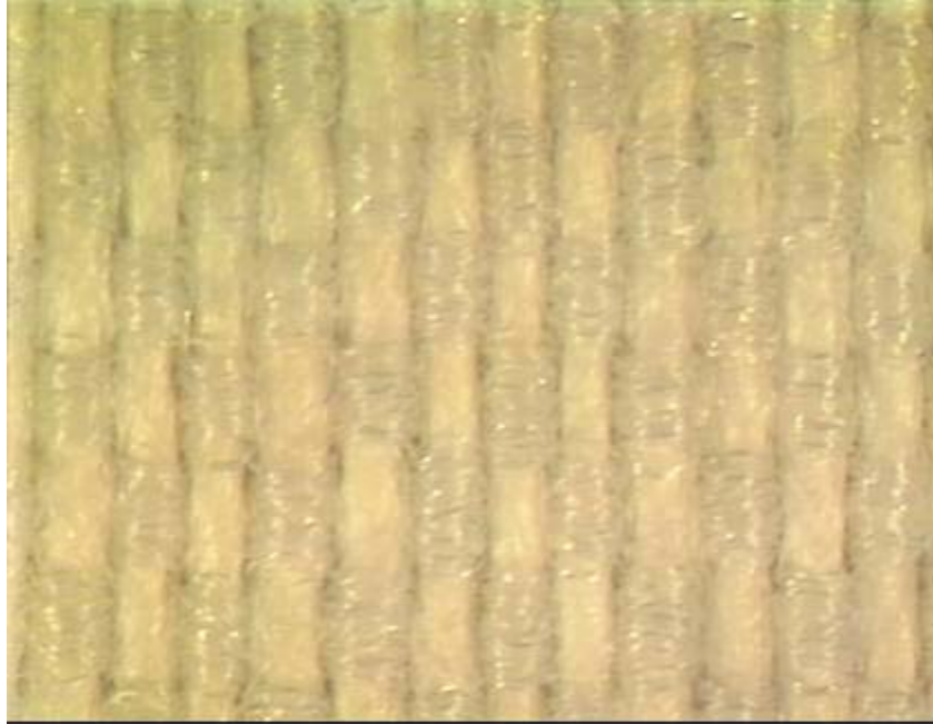
Figure 5. 23: Optical image of woven finished elastomeric fabric (In-loom fabric Tightness: 0.74, 84 EPI x 55 PPI) with 152D filling) Magnification 25x
