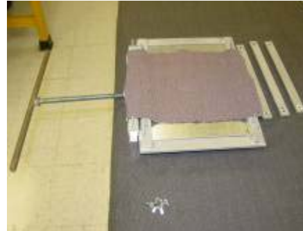
4.3b) Fabric sample placed on frames of platform
