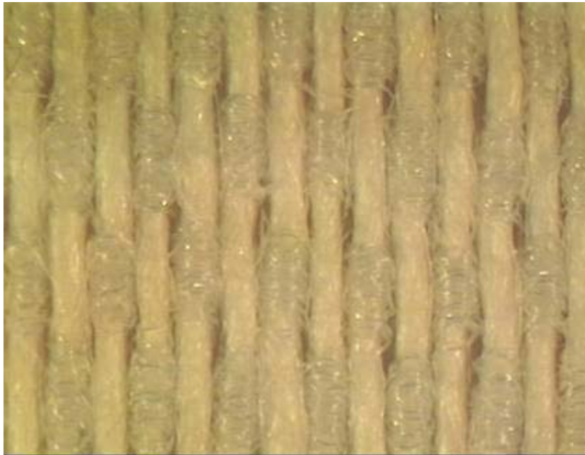
Figure 5. 10: Optical image of finished elastomeric fabric at 0% strain [Fabric construction detail: 89 EPI x 30 PPI) with 152 D filling] Magnification 25x
