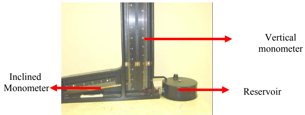
Figure 4. 13c: Position of reservoir, Inclined Monometer and reservoir
