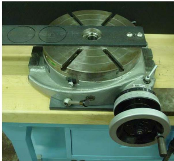
Figure 4.4: Rotary table with plank attachment.
