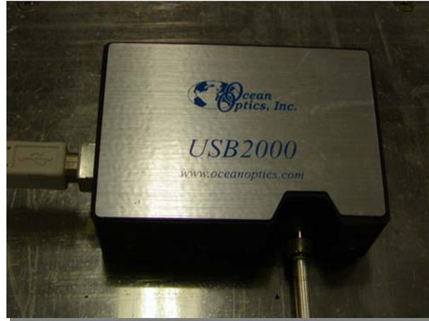
Figure 4.13: USB2000 spectrometer used in high temperature experiments.
