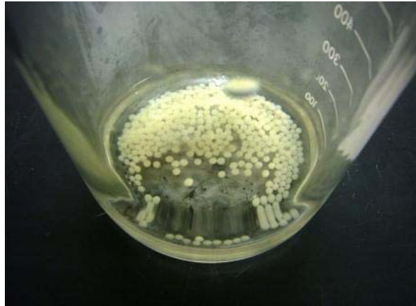
Figure 5. 2 Yeast culture immobilization in Ca-alginate beads
