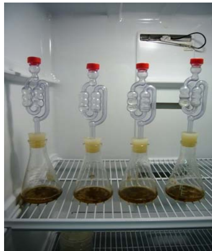
Figure 5. 3 Equipment for immobilized yeast cell fermentation
