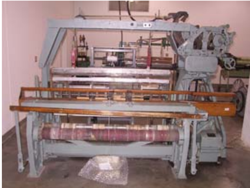
Figure 3. 7. Loom used for weaving tubular structures
