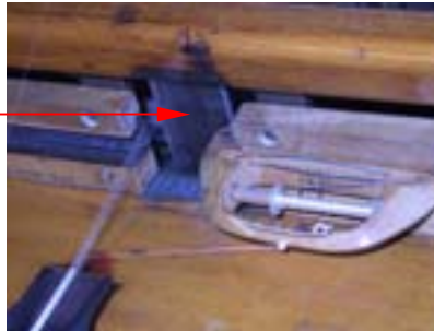
C. Shuttle after placing a fill yarn in the shed
