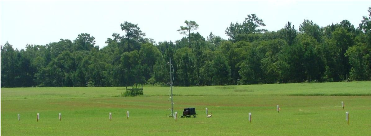
**Figure 3.11. Arrangement of catch cans in the traveling gun plot before land application**
