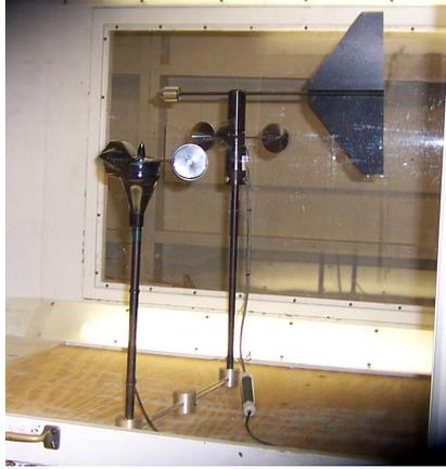
**Figure 3.3. Arrangement of two anemometers in wind tunnel.**
