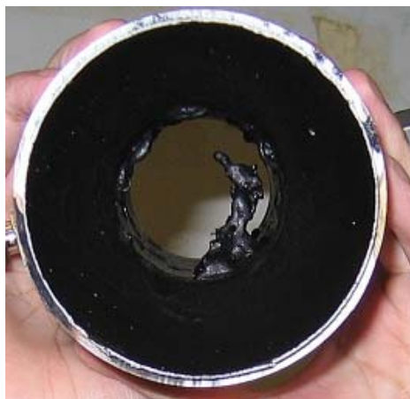
Figure 14. Picture of the black residue, which collected on the venturi from burning animal fat derived glycerol.
