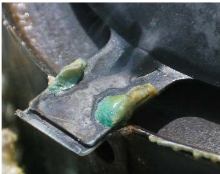
Figure 15. A close up picture of the residue found on the top of the flame enclosure after burning animal fat derived glycerol.
