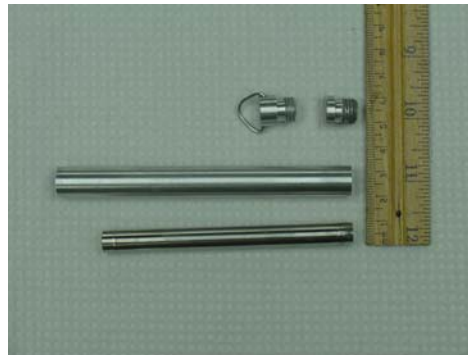
Figure E-2. Outer Aluminum Capsule and End Caps (top) & Inner Stainless Steel (bottom) Capsule
