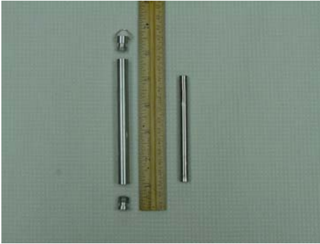
Figure E-1. Outer Aluminum Capsule and End Caps (left) & Inner Stainless Steel (right) Capsule
