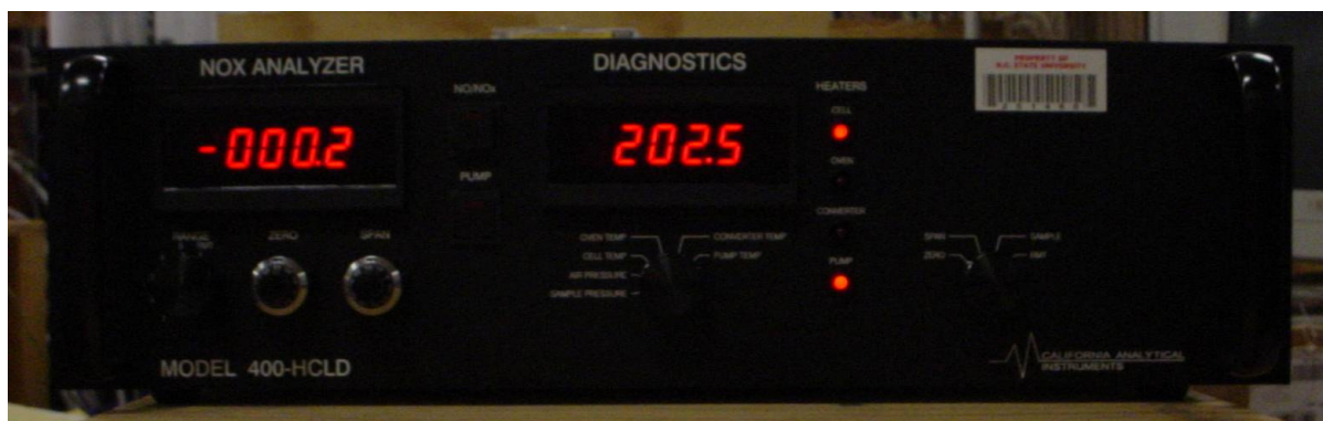
Figure 2.3 – California Analytical Instruments Model 400 HCLD NO/NO x analyzer used in experiments.
