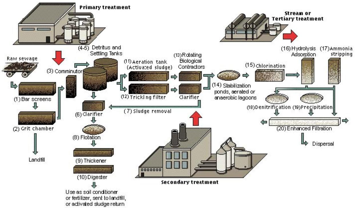
**Figure 1.** Diagram of a wastewater treatment plant. Adapted from Carroll, 2007.
