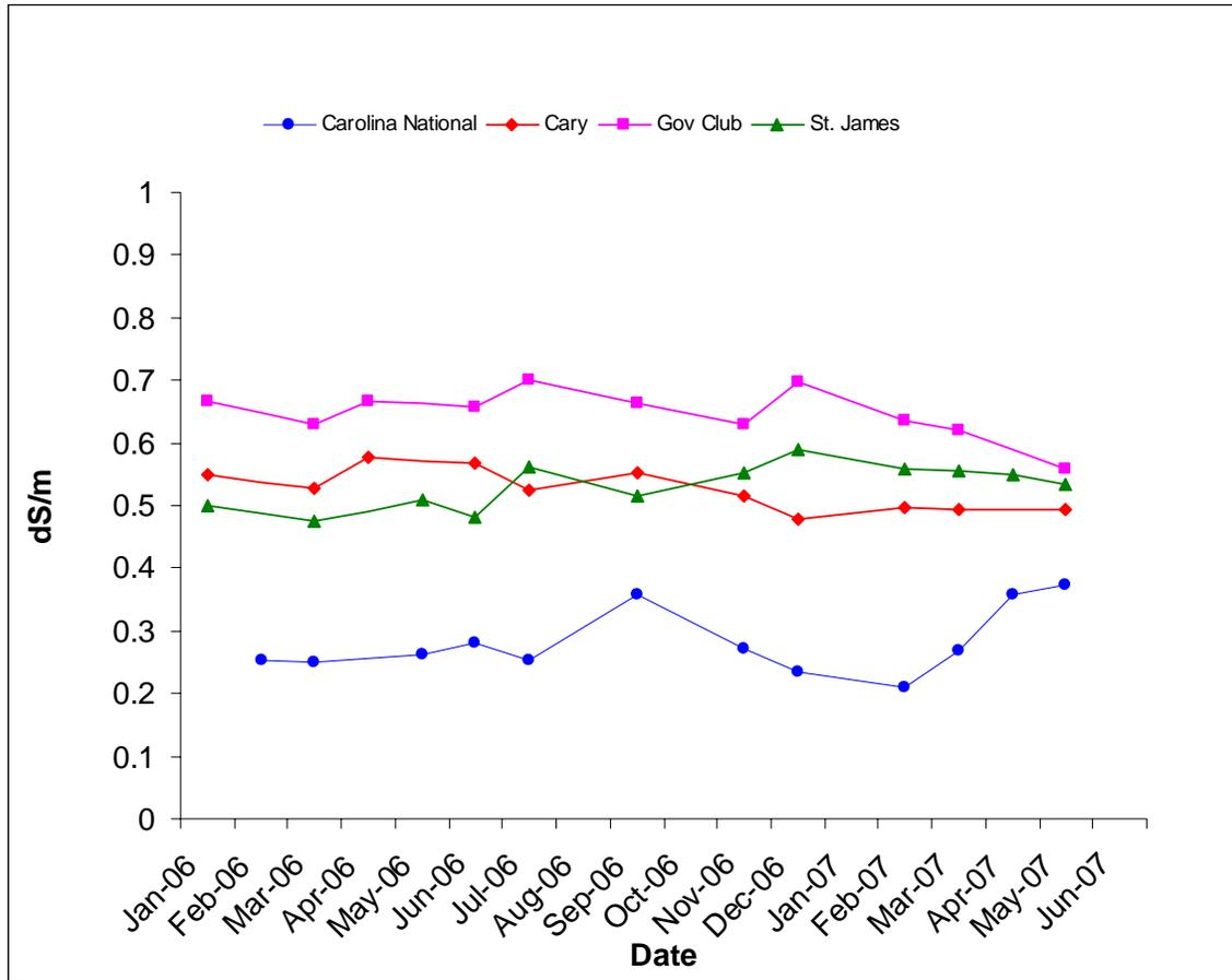
**Figure 3.** Conductivity levels for all four effluent locations from January 2006 to May 2007.
