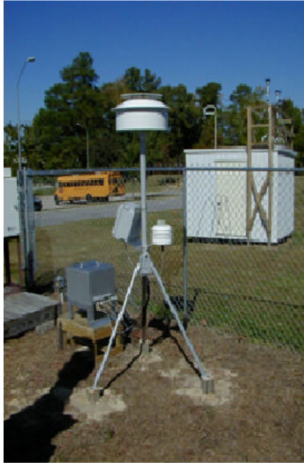
Figure 7: “SASS” Met One’s Particulate Matter Speciation Samplers operated by NC Division of Air Quality.
