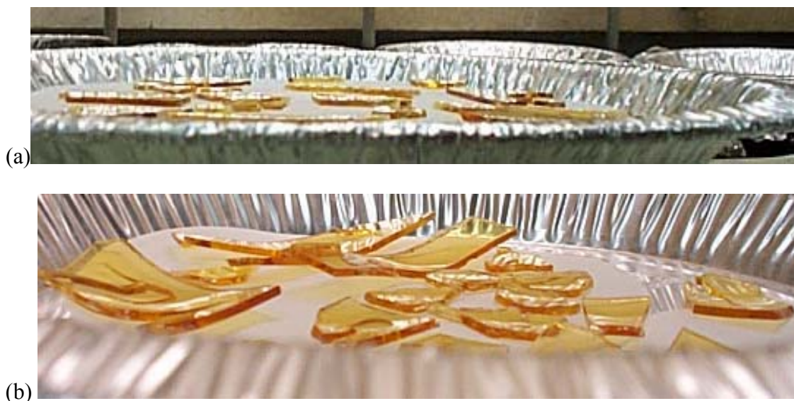
Figure 4.2 Films dried on an elevated rack in aluminum pans (a) did not curl while films dried on flat filter paper (b) did curl during drying. Uniform drying thus eliminates film curling.
