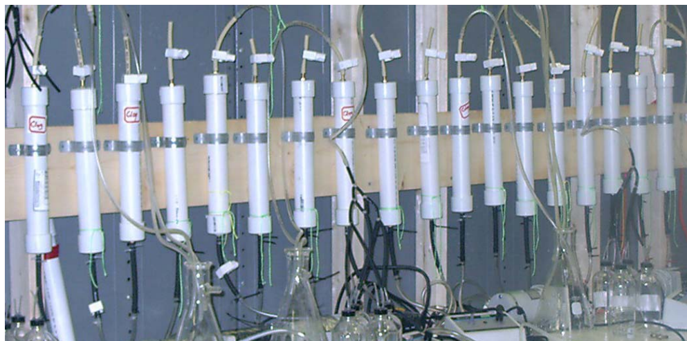
Figure 5. Set up of the intermittent flow columns.
