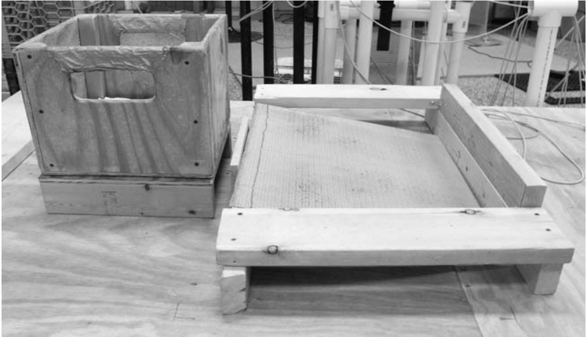
Figure 2.2 Wooden platform (10° inclined slope) and weight box
