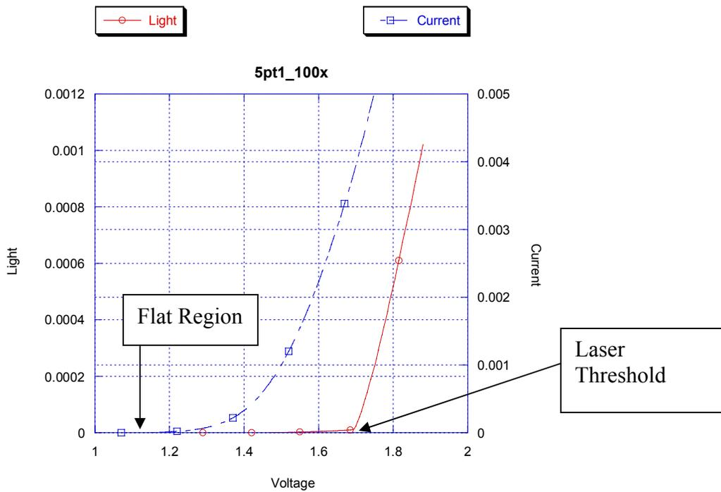
**Figure 20** Current versus voltage and light versus voltage measurements plotted on the same graph to show similarities. The similarities start with the flat region before laser threshold, after laser threshold both curves have rapidly rising slopes.
