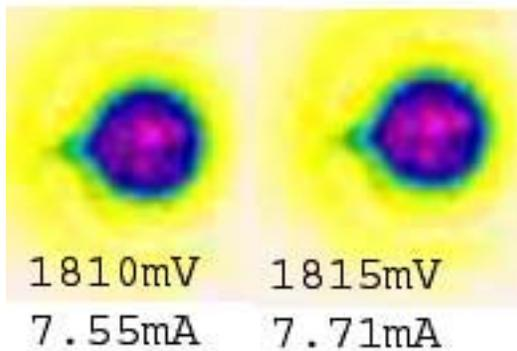
**Figure 26 Modal pattern of Proton number five test number five. These images show the optical modes at 1810mV (~7.55mA) and 1815mV (~7.71mA), above laser threshold 1665mV (~3.68mA).**
