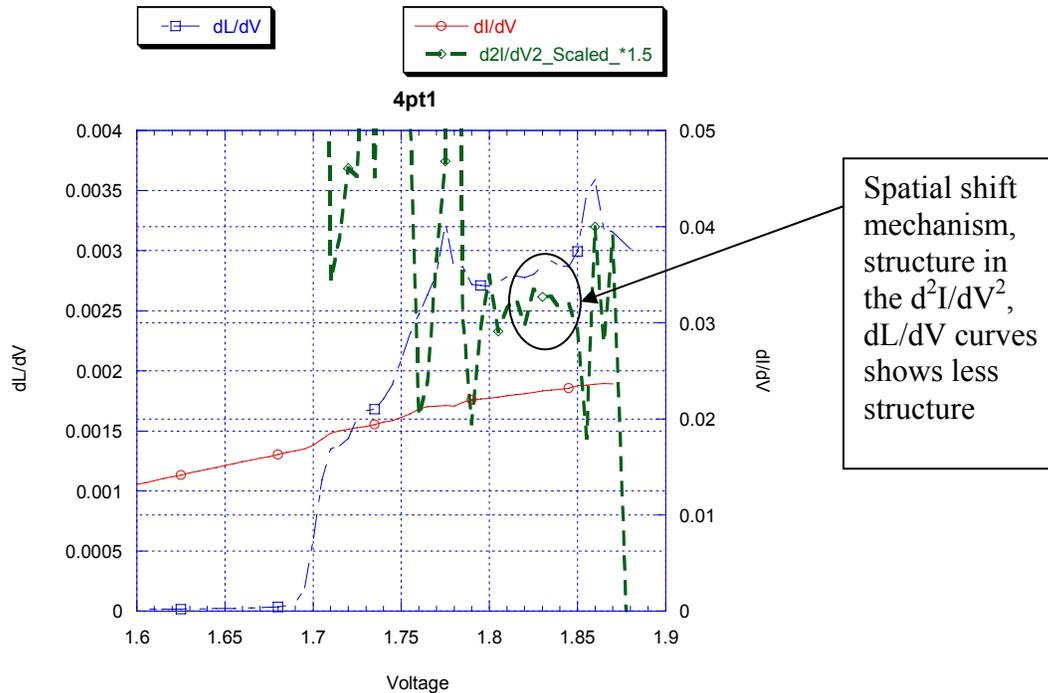
**Figure 39. Spatial mode shift of the light output. Second derivative of current shows a large amount of structure while the  $dL/dV$  curve shows a region with less structure. One would also expect only minor variations in the light output since no new laser filaments evolve, only spatial shifting of the existing filaments.**
