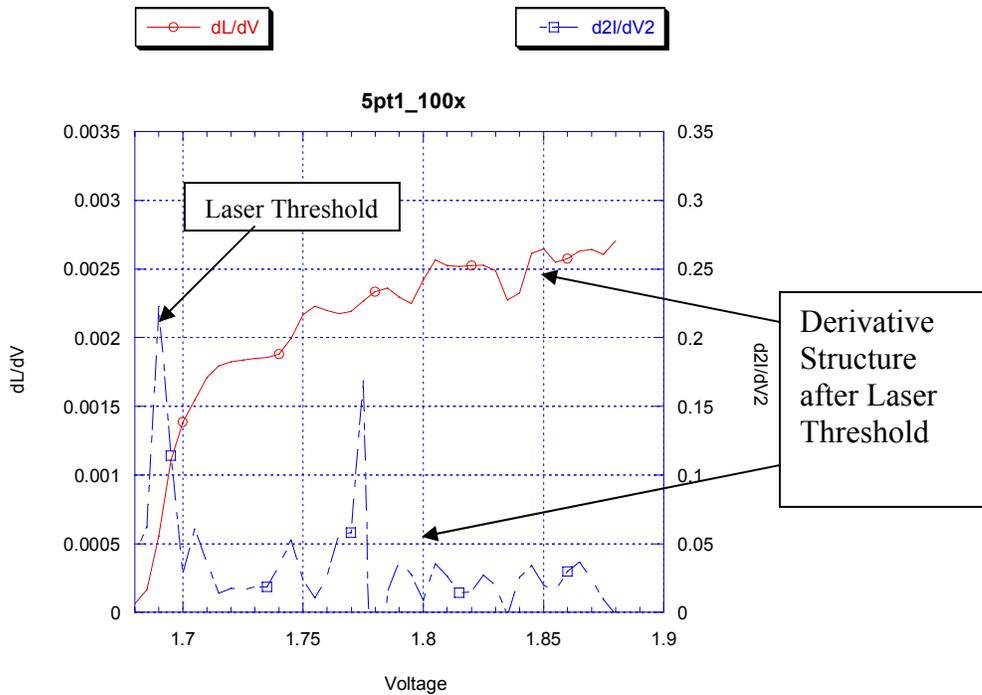
**Figure 24 First derivative of Light and Second derivative of Current zoomed in to view the structure of both plots.**
