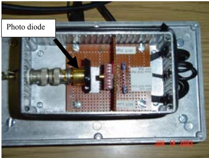
**Figure 13 Full view of the Voltage Photodiode test fixture without the inner cover and external light shield removed.**
