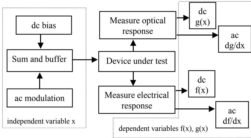
**Figure 1** The response to an applied current (voltage) to a device under test results in a response of voltage (current or light output). The first derivative is proportional to magnitude of the ac signal. Improved signal to noise is obtained by using phase sensitive detection to recover the ac signal.
