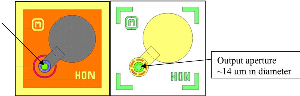
**Figure 5** On the left is the Proton VCSEL, where the smaller dot (pointed out by arrows) surrounded by the blue ring is the output aperture. On the right the Oxide VCSEL is shown, the output aperture is also the light green area inside the slotted orange circle.
