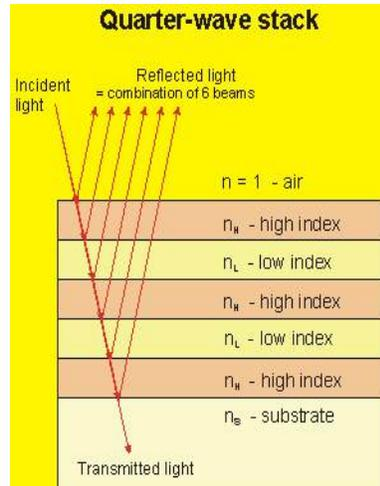
**Figure 6 Dielectric mirror stack; at dielectric interfaces there is a reflection due to the change in refractive indexes**
