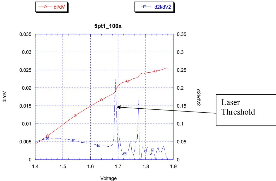
**Figure 22 First and Second derivative plots. The first bulge in the second derivative is the spontaneous emission of the device, this part of the curve directly relates to the change slope in the first derivative. The large peak in the second derivative shows laser threshold, this peak highlights the slope change in the first derivative.**
