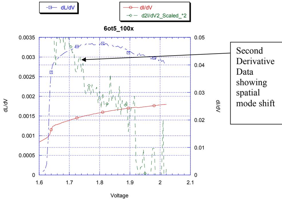
**Figure 44 Spatial shift of the light output, second derivative of current shows a large amount of structure while the  $dL/dV$  curve shows a region with less structure. One would also expect only minor variations in the light output since no new laser modes evolve, only spatial shifting of the existing modes.**
