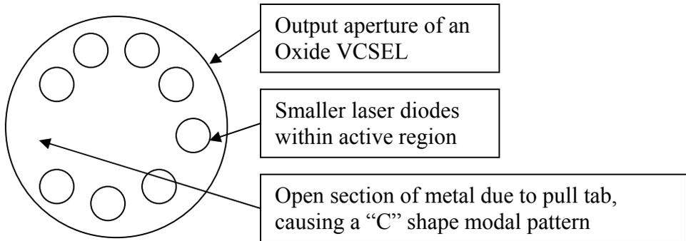
**Figure 43 Representation of output aperture of an oxide VCSEL with a number of smaller laser modes inside the active region of the device. Note the modes form a “C” shape, this is due to a hole in the metal contact which causes little or no current to flow in the open portion of the “C” so no modes can start to lase.**
