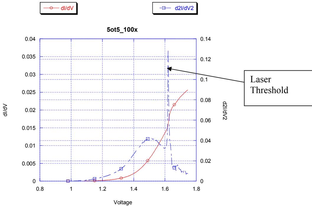
**Figure 30 First and Second derivative of current versus voltage. The first maximum in the second derivative corresponds to spontaneous emission from the device. The large peak in the second derivative shows laser threshold, this peak highlights the slope change in the first derivative.**
