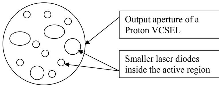
**Figure 38 Representation of output aperture of a proton VCSEL with a number of smaller laser filaments inside the active region of the device. The random mode pattern may be due to low optical confinement allowing different regions to lase better than others.**
