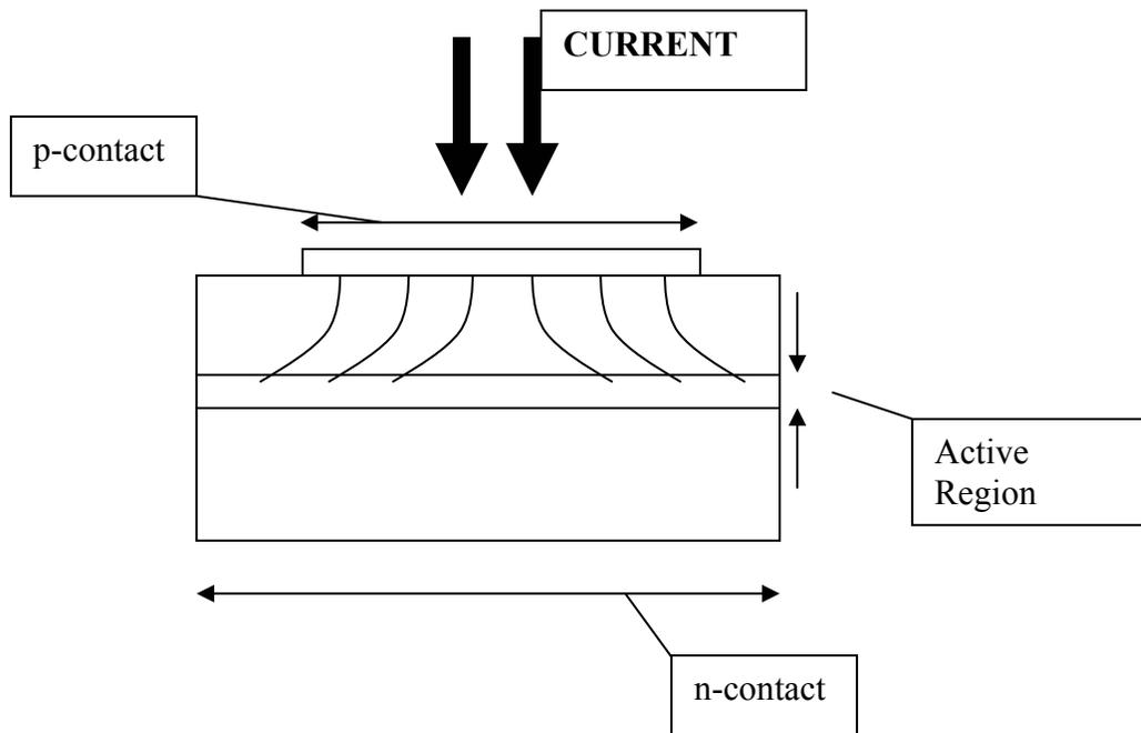
**Figure 7 Example of Current Spreading in a device without a current confinement mechanism in place.**
