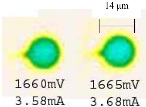
**Figure 25 (Left) Proton number five test run five, 1660mV (~ 3.58mA) just before laser threshold. (Right) Proton number five test run five, 1665mV (~ 3.68mA) laser threshold. An increase in the light intensity can be seen from left to right. The image has been false colored to better view the change light intensity.**
