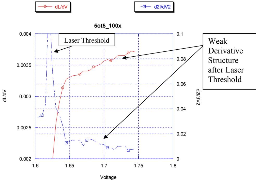
**Figure 32 First derivative of Light and Second derivative of Current zoomed in to view the structure of both plots.**
