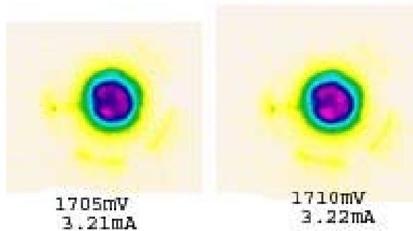
**Figure 34 Modal pattern of Oxide number six test number nine. These images show the optical modes at 1705mV (~ 3.21mA) and 1710mV (~ 3.22mA), above laser threshold 1635mV (~ 1.89mA). The center of the cavity does not seem to have as much laser action as the perimeter of the output aperture.**
