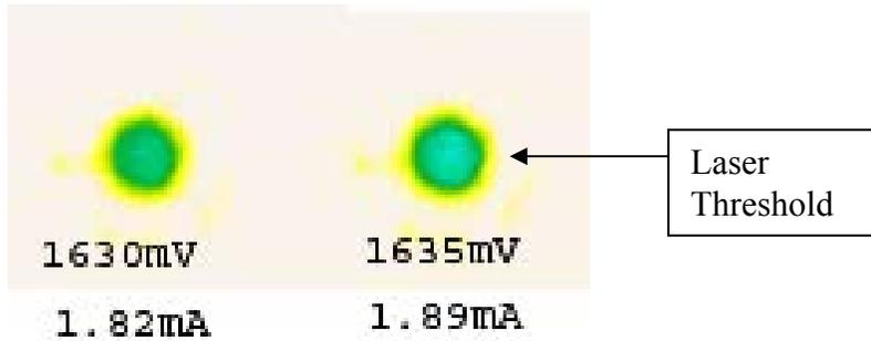
**Figure 33 (Left) Oxide number six test run nine, 1630mV (~ 1.82mA) just before laser threshold. (Right) Oxide number six test run nine, 1635mV (~ 1.89mA) laser threshold. An increase in the light intensity can be seen from left to right. The image has been false colored to better view the change light intensity.**
