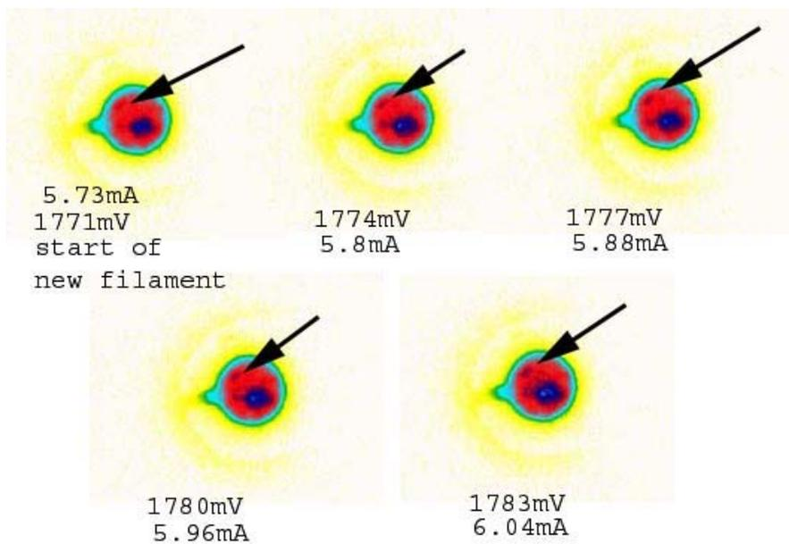
**Figure 37** New mode starts at  $\sim 1770\text{mV}$  pointed out by the arrow. These modal patterns correspond with the derivative curves in Figure 36.
