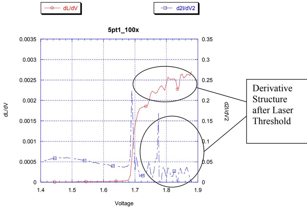
**Figure 23 First derivative of Light ( $dL/dV$ ) and Second derivative of the current ( $d^2I/dV^2$ ). The first peak in the second derivative corresponds to the sharp rise in the first derivative of light. There is additional structure in the plots after threshold.**
