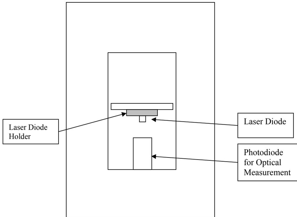
**Figure 11 Block diagram of the Voltage Photodiode Test Fixture.**
