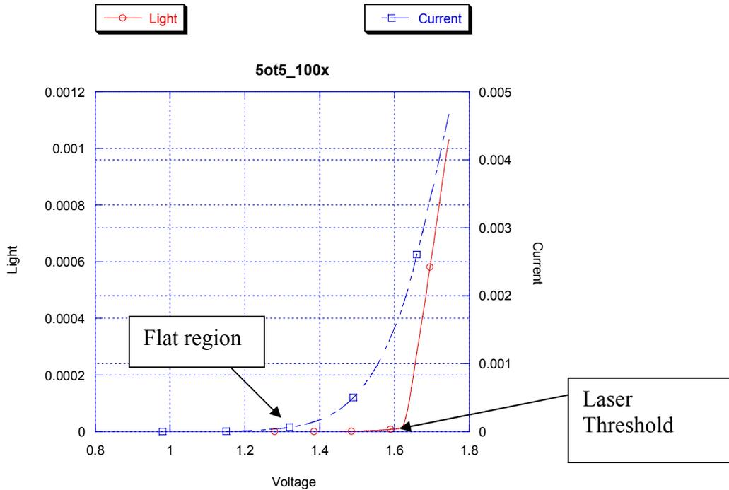
**Figure 28** Current versus voltage and light versus voltage measurements plotted on the same graph to show similarities. The similarities start with the flat region before laser threshold, after laser threshold both curves have rapidly rising slopes.
