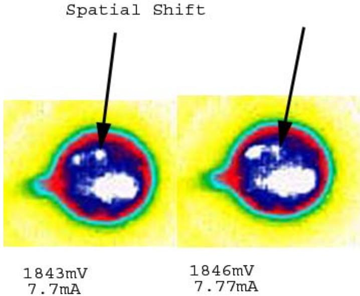
**Figure 40** Optical image of a spatial shift, corresponding with the derivative structure displayed in Figure 39. One explanation for a spatial shift of a laser filament is that a new section of the active region provides a better (lower resistance) path to the current. This change in the preferred path of the current could be due to localized heating, current crowding, etc but the specific cause is not important at this point, only that the shift can happen.
