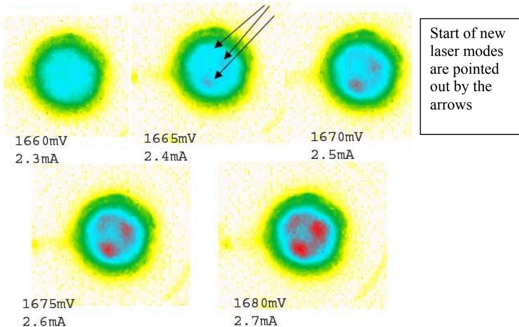
**Figure 42** New mode starts at  $\sim 1660\text{mV}$  pointed out by the arrow. These modal patterns correspond with the derivative curves in Figure 41.
