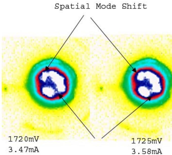
**Figure 45. Optical image of a spatial shift, corresponding with the derivative structure displayed in Figure 44. One explanation for a spatial shift of a laser mode is that a new section of the active region provides a better (lower resistance) path to the current. This change in the preferred path of the current could be due to localized heating, current crowding, etc.**
