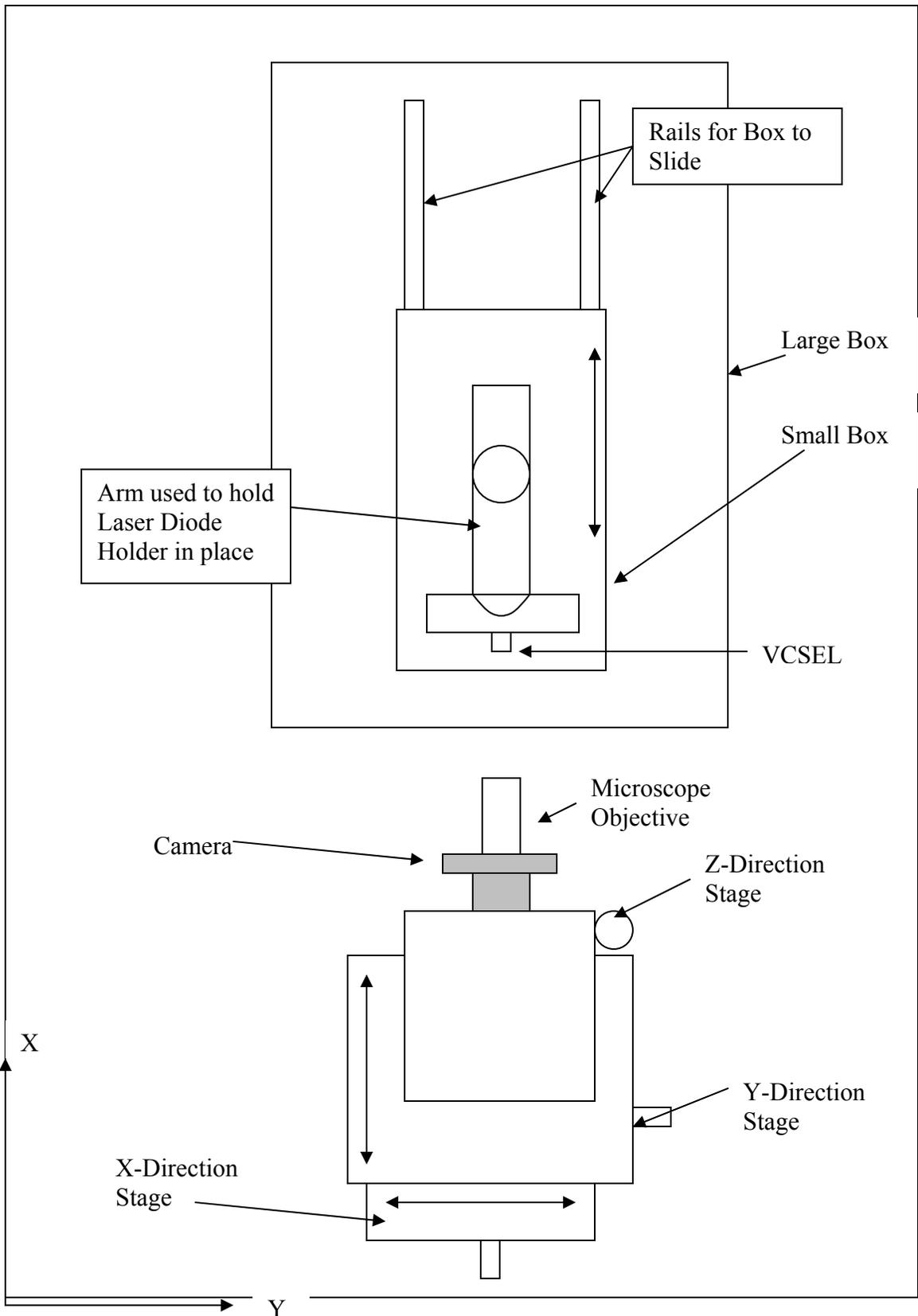
**Figure 16 Block Diagram of the Camera Voltage Test Fixture.**
