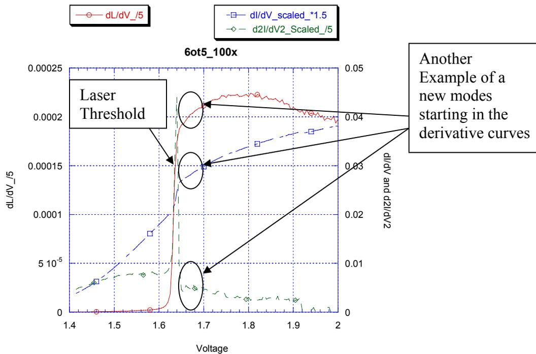
**Figure 41** The first mechanism is seen at threshold where a new laser mode is formed. Note that at threshold there is a rapid rise in  $dI/dV$ ,  $dL/dV$ , and a narrow peak in  $d^2I/dV^2$ .
