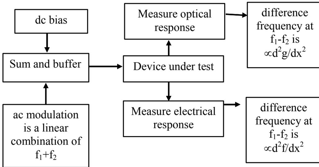
**Figure 2 The second derivative is obtained in a low noise environment by using the difference frequency method of Paoli. The generation of a low distortion ac modulation signal in conjunction with time-continuous digitally tunable filters has enable us to construct a derivative system that used analog phase sensitive signal recovery in conjunction with computer control.**
