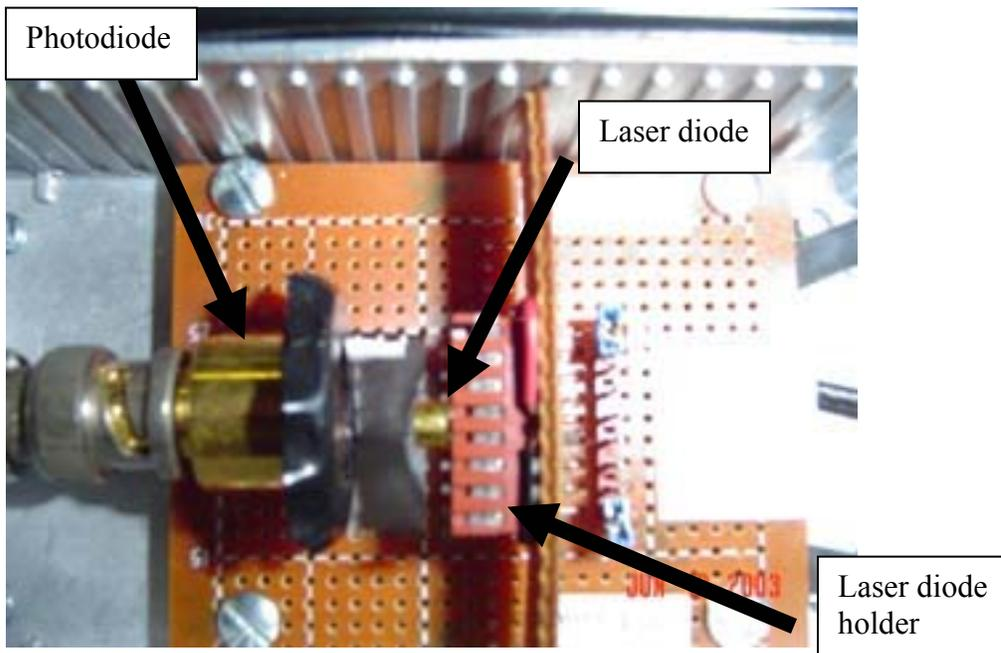
**Figure 12 Close up of Laser diode held in front of a photodiode in voltage photodiode box.**
