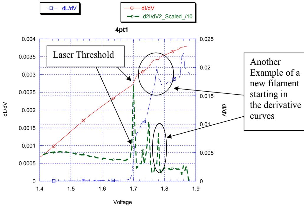
**Figure 36** The first mechanism is seen at threshold where a new laser mode is formed. Note that at threshold there is a rapid rise in  $dI/dV$ ,  $dL/dV$ , and a narrow peak in  $d^2I/dV^2$ .
