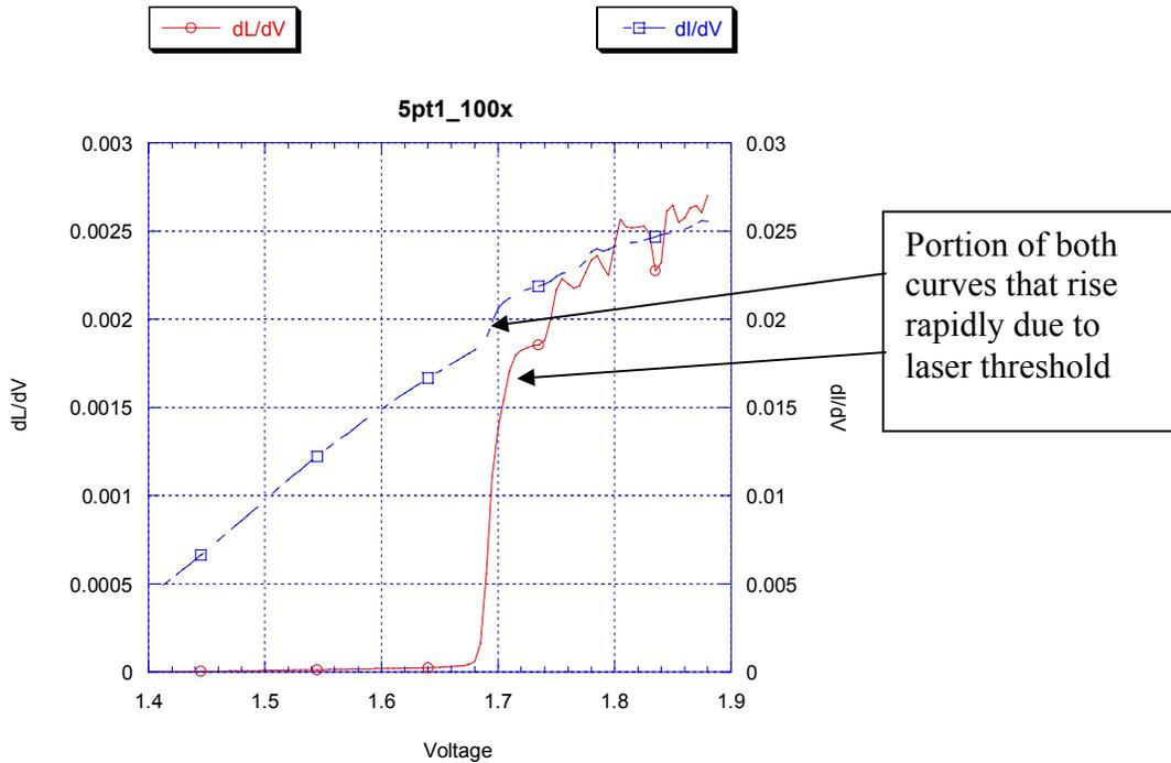
**Figure 21 First derivative of the light and current versus voltage. The first derivative curves show a sharp rise at laser threshold and roll over at approximately the same drive voltage.**
