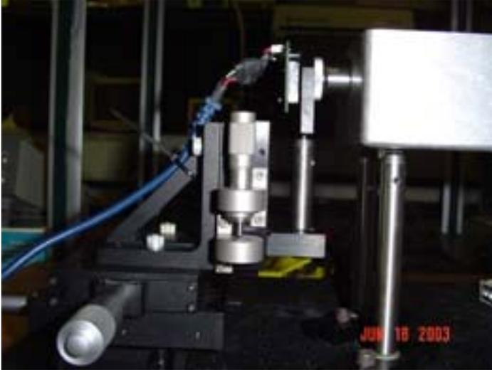
Figure 17 Three translation stages used to hold camera and objective lens for optical camera box.
