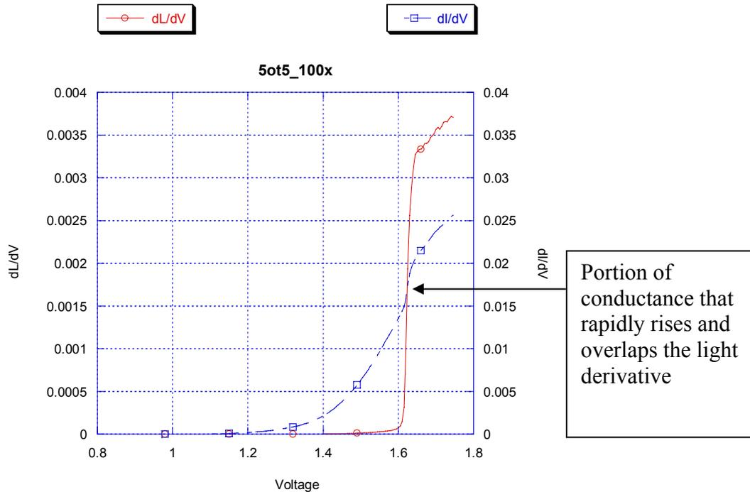
**Figure 29** First derivative of the light and current versus voltage. The first derivative curves show a sharp rise at laser threshold and roll over at approximately the same drive voltage.
