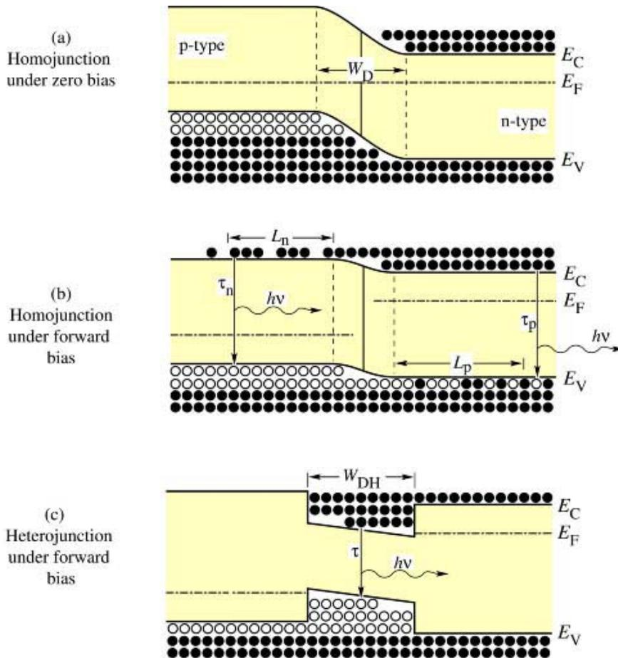
Figure 3 P-N homo and double heterojunctions. The heterojunction improves the confinement of carriers and reduces laser threshold.
