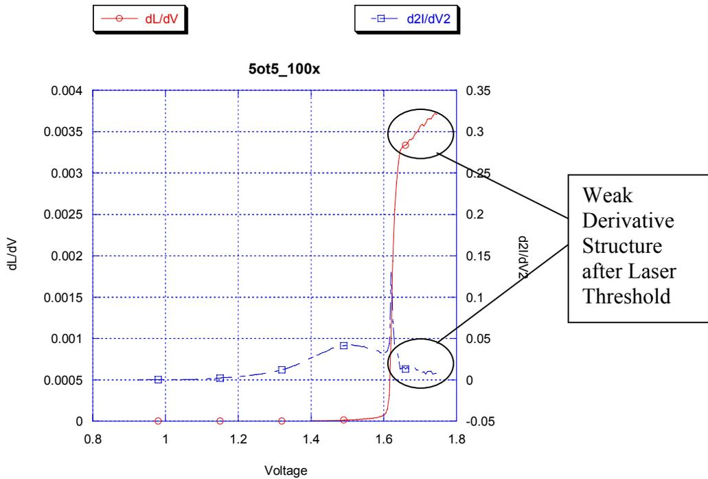
**Figure 31 First derivative of Light ( $dL/dV$ ) and Second derivative of the current ( $d^2I/dV^2$ ). The peak in the second derivative corresponds to the sharp rise in the first derivative of light. There is a small amount of structure in the plots after threshold.**
