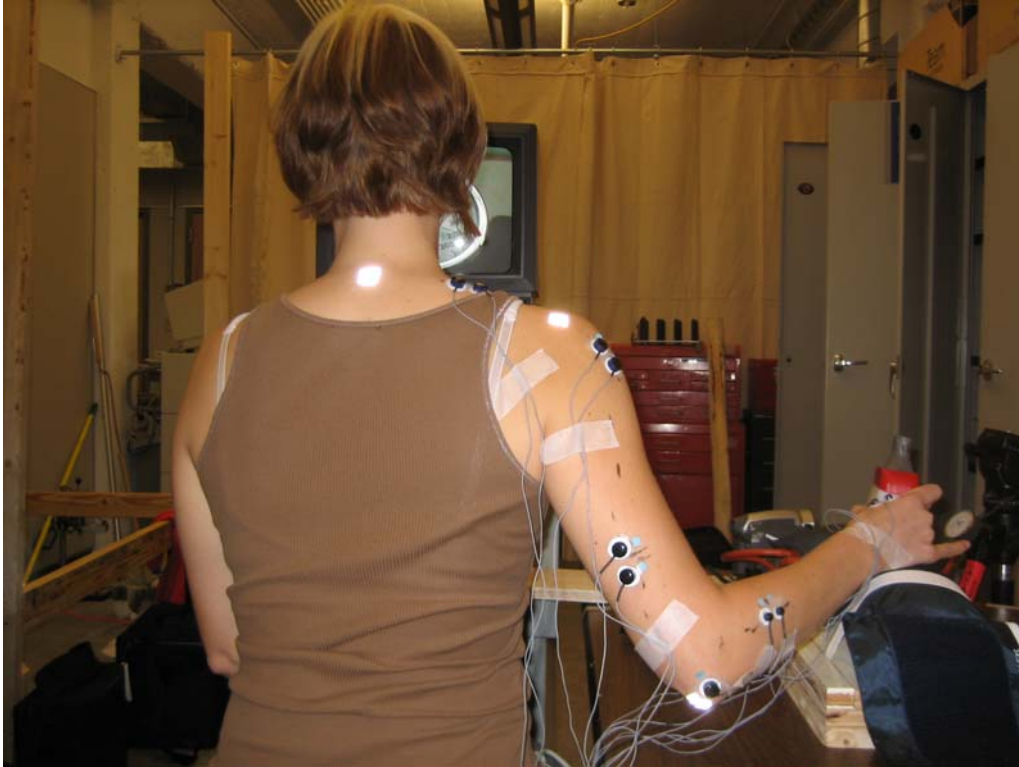
Figure 2.7. Experimental task setup, 0 degrees. A seated subject applies pressure against an abdomen-like surface at a 0 degree angle while viewing the pressure gauge on a monitor.
