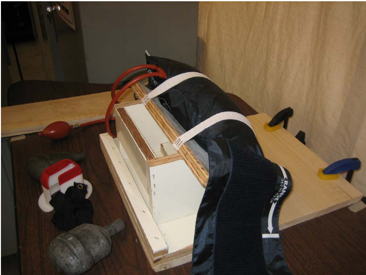
Figure 2.6. Experimental task apparatus. Abdomen-like surface (inflated blood pressure cuff) is positioned at 45 degrees.
