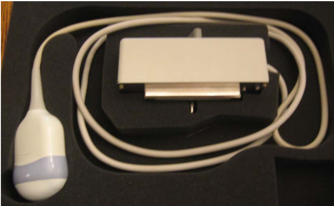
Figure 2.1. Ultrasound transducer. This functioning ultrasound transducer, used in the Duke Fetal Diagnostic Center, served as the model for the control and interventions used in the current study. The transducer is one unit as shown; the cable cannot be detached from the large box-like unit for connection to the ultrasound machine.
