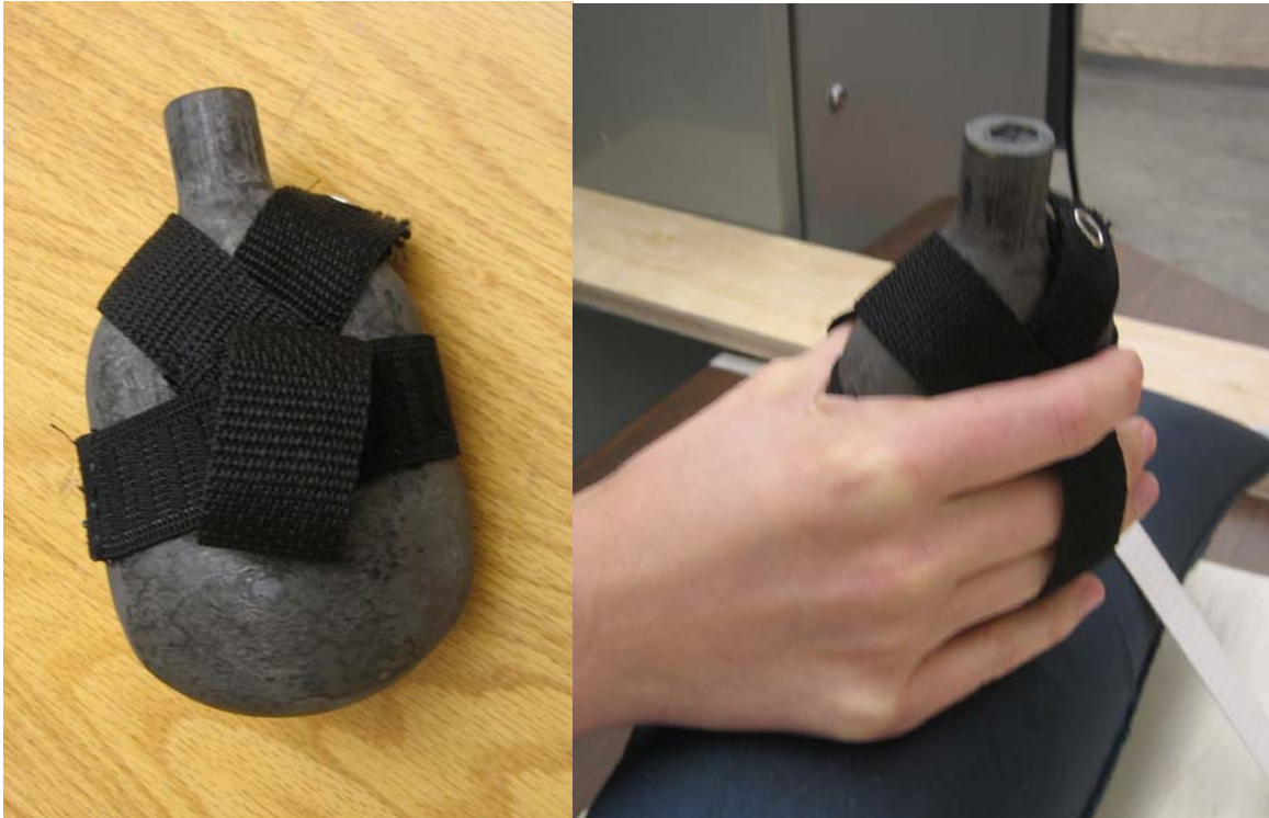
Figure 2.4. Transducer harness. The thumb and two middle fingers were secured to the transducer through the finger loops of the harness intervention as shown. Subjects were instructed to pull down on the loops rather than pinch and pull down on the transducer.
