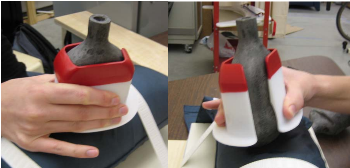
Figure 2.3. Transducer cover. The cover intervention featured a support ledge to be pushed down upon as shown.
