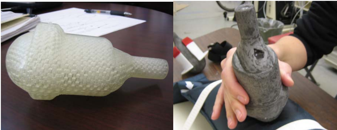
Figure 2.5. Wide grip transducer. The image on the left shows the wide grip transducer prior to the addition of the steel weight, and the right image shows the intervention held with fingers wrapped around in a power grip.
