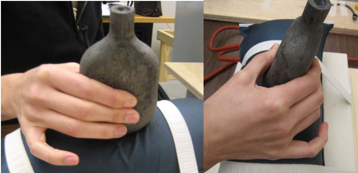
Figure 2.2. Control transducer. A rapid prototyped replica of an actual ultrasound transducer was made for use as the control transducer. Subjects were instructed to use a pinch/palmar grip with index and middle finger placed as shown.
