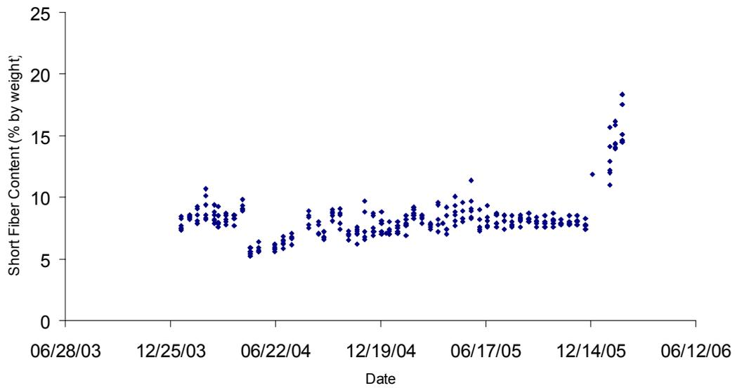
**Figure 5.7: Sliver short fiber content (% by weight) for card line 1**
