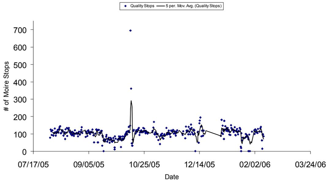
**Figure 5.15: Quality stops for spinning frame B**
