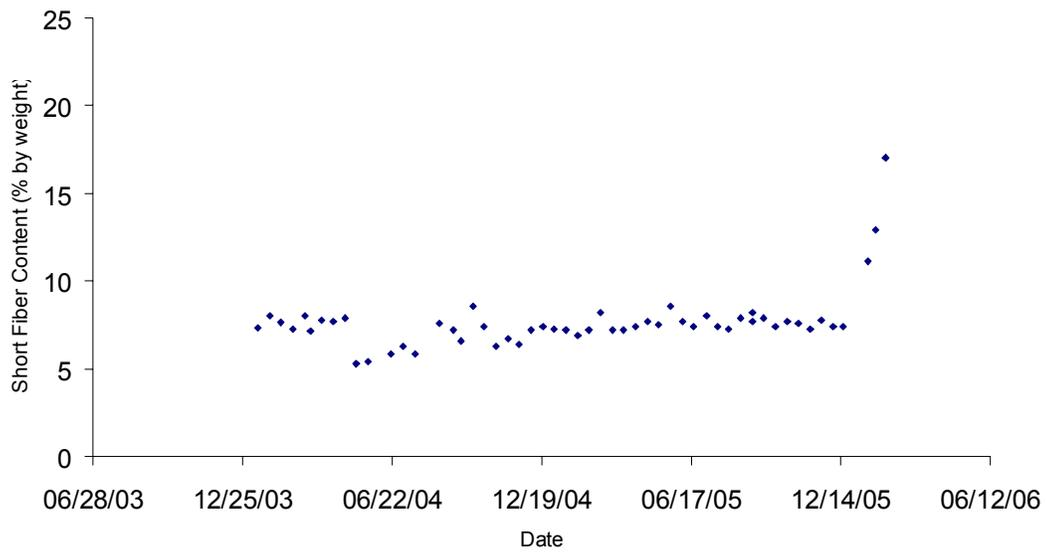
**Figure 5.6: Mat short fiber content (% by weight) for card line 1**
