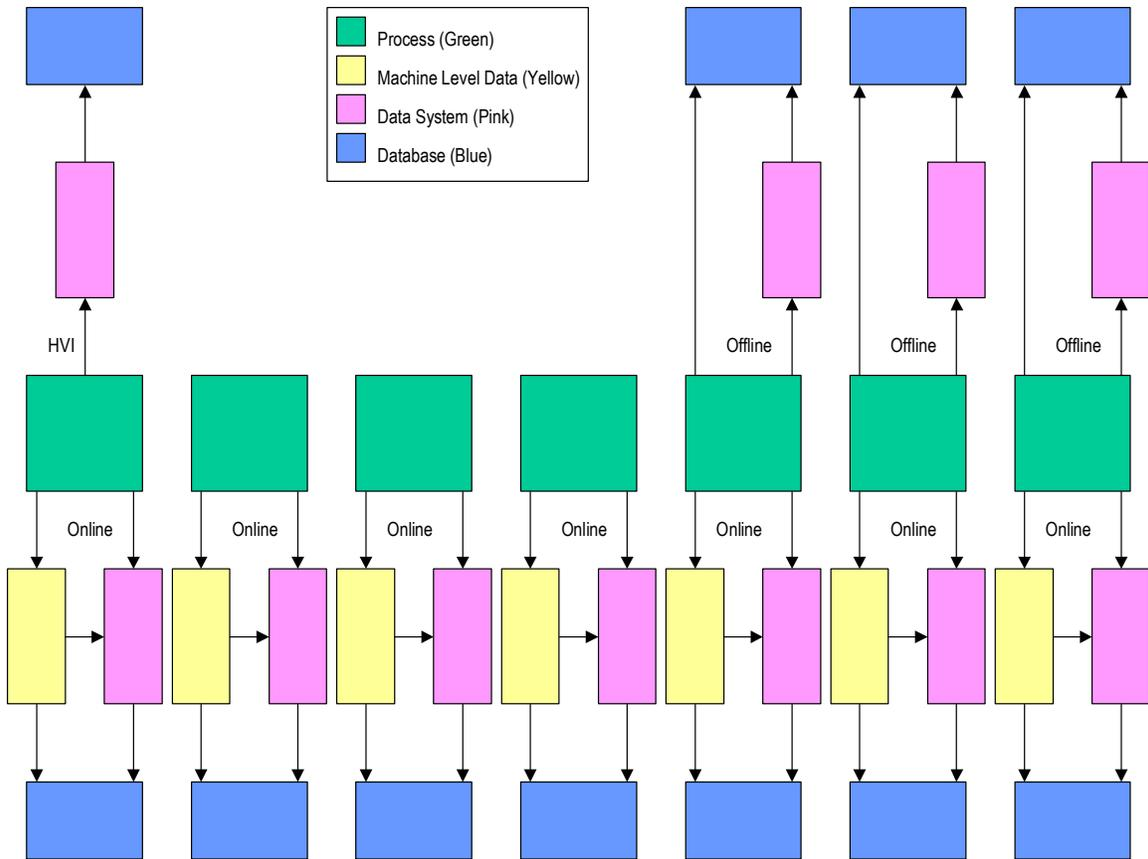
**Figure 4.5: Data flow in a spinning plant**
