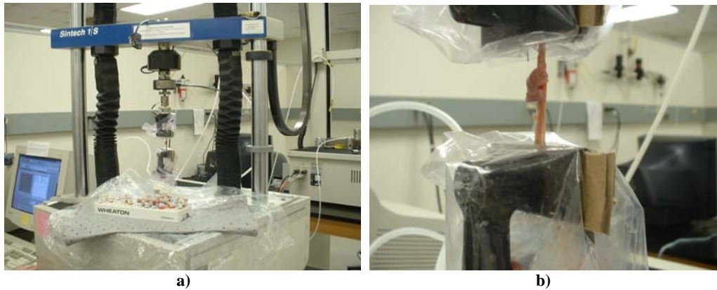
Figure 6: a) MTS Sintech 1/S Tensile Testing Machine, b) cardiac tissue sample mounted in machine grips
