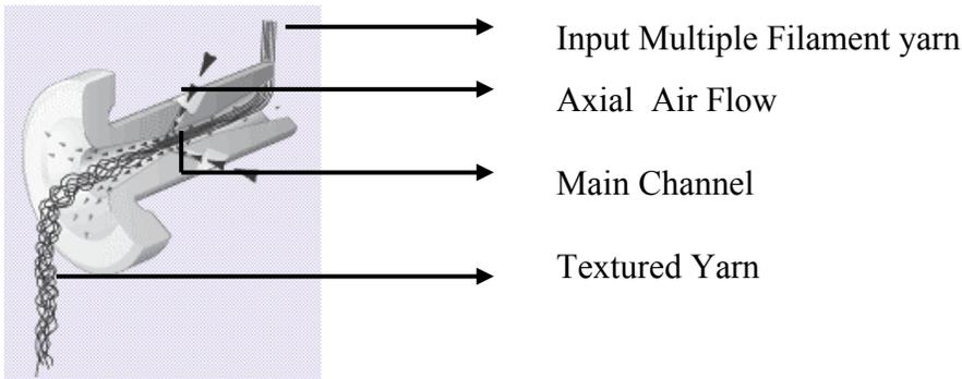
**Figure 2.2:** Flow of air and material within the jet [14]
