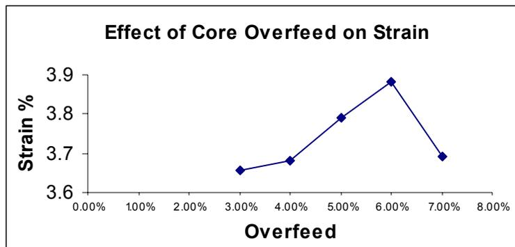
**Figure 3.8:** Effect of Core Overfeed on the Strain
