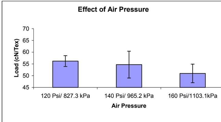
**Figure 2.7:** Effect of Air Pressure at a speed of 300 m/min and over feed of 50%
