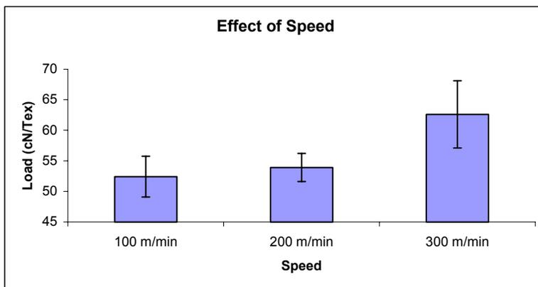
**Figure 2.8:** Effect of Speed at Air Pressure of 120 Psi/ 827.3 kPa and Overfeed of 50%
