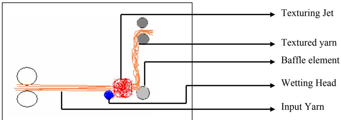
**Figure 2.1:** Schematic representation of the Air texturing Process
