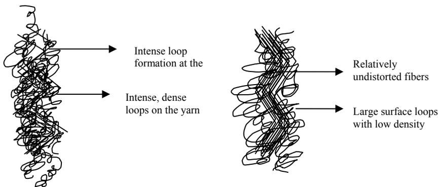
**Figure 2.15:** Structural comparison of intensely textured yarn(a) to poorly textured yarn(b) based on figure 2.12
