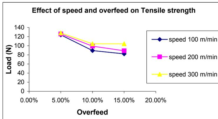
**Figure 3.4:** Effect of speed and overfeed on Tensile Strength
