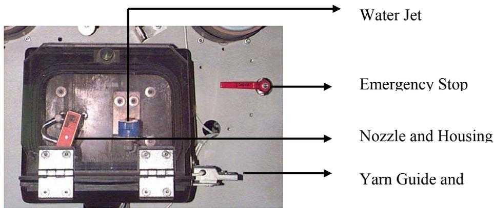
**Figure 4.5:**Texturing box , with jet and wetting head
