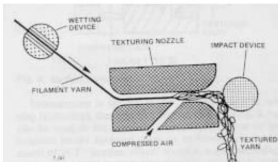
**Figure 2.4:** Flow of material from the wetting head to its withdrawal after texturing [8]
