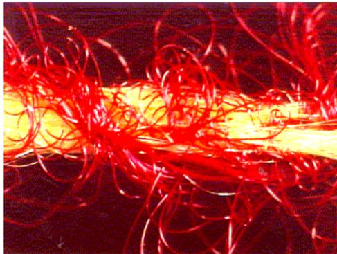
**Figure 3.1:** Structure of the sheath-core yarn.
