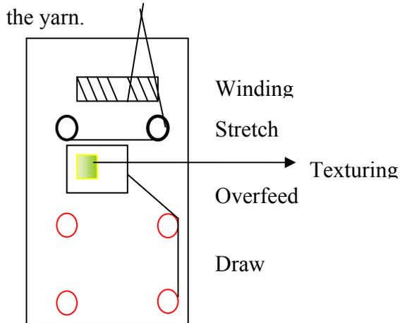
**Figure 2.5:** Yarn path on the texturing machine
