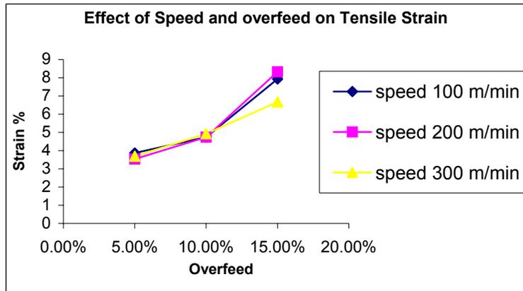
**Figure 3.5:** Effect of Speed and overfeed on the Tensile Strain
