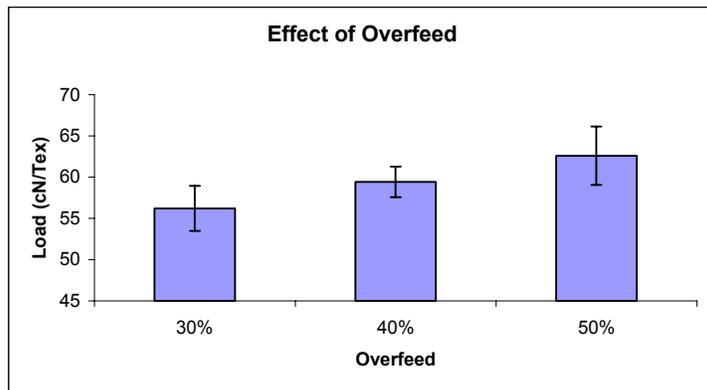
**Figure 2.9:** Effect of Overfeed at Air pressure of 120 Psi/ 827.3 kPa and speed 300 m/min
