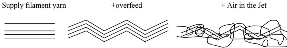
**Figure 2.14:** The Sequence of structural changes in the yarn
