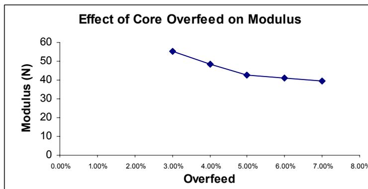
**Figure 3.9:** Effect of Overfeed on the Tensile Modulus
