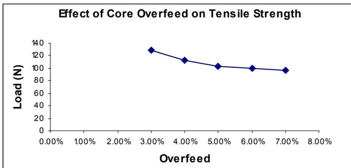
**Figure 3.7:** Effect of Overfeed on the Tensile Strength
