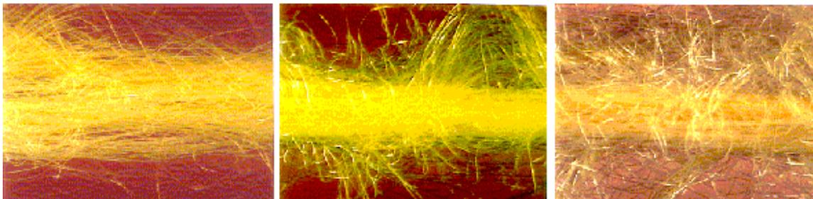
**Figure 3.2:** Relative loop sizes at overfeed of (a) 30% (b) 70 % (c) 100 %
