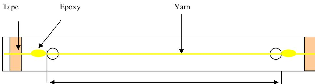
**Figure 2.6:** Cardboard with yarn, tape and epoxy
