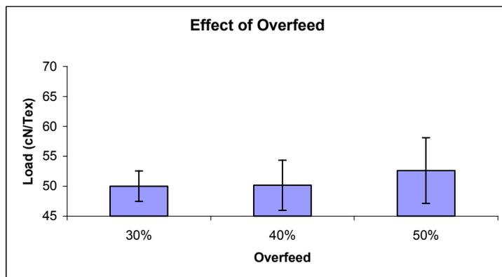
**Figure 2.10:** Effect of Overfeed at an Air pressure of 160 psi/ 1103.1 kPa speed of 300 m/min
