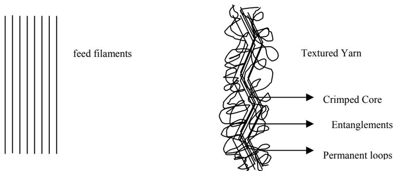
**Figure 2.13:** Components of Sheath Core yarns
