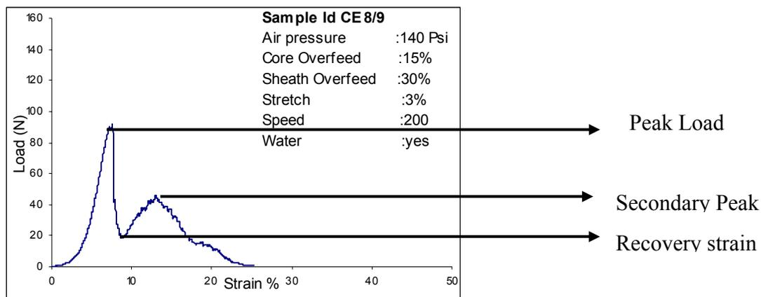
**Figure 3.3:** Tensile Behavior of Sheath-Core Yarns
