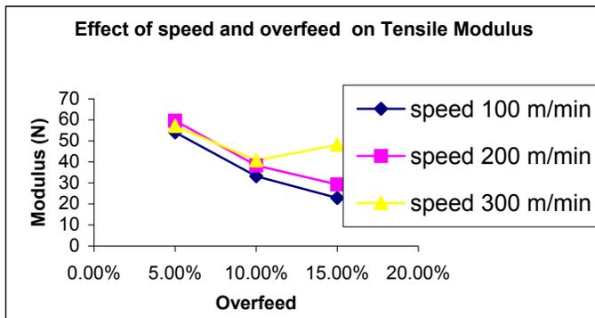
**Figure 3.6:** Effect on the Tensile Modulus
