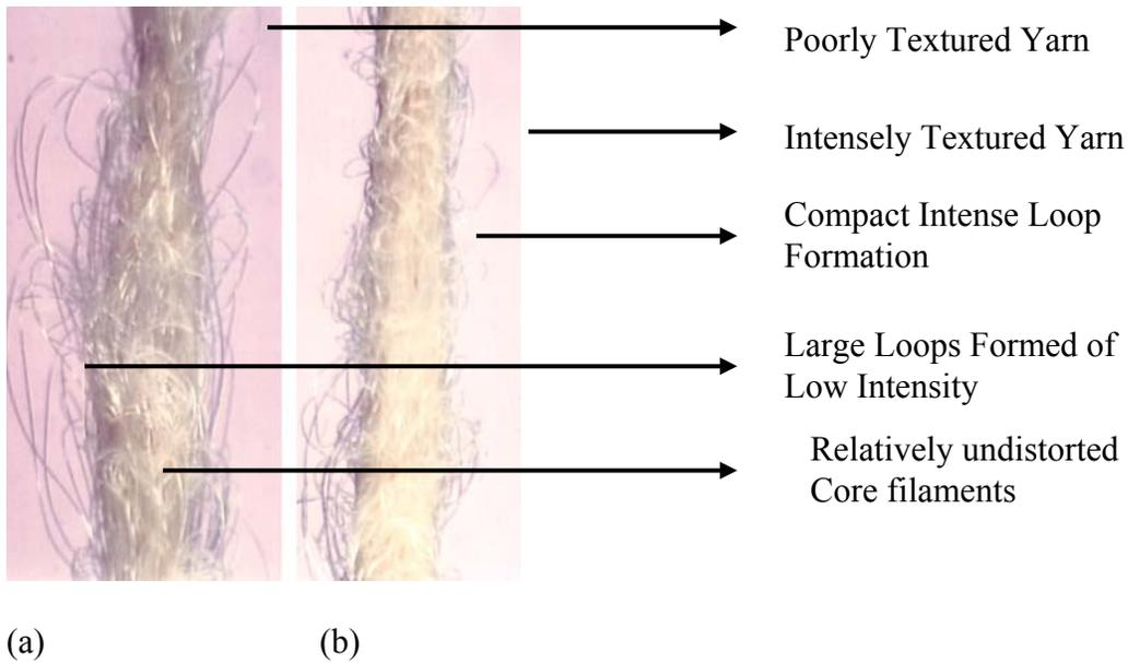
**Figure 2.12:** Comparison of (a) Poorly Textured yarn with (b) Intensely Textured Kevlar yarn
