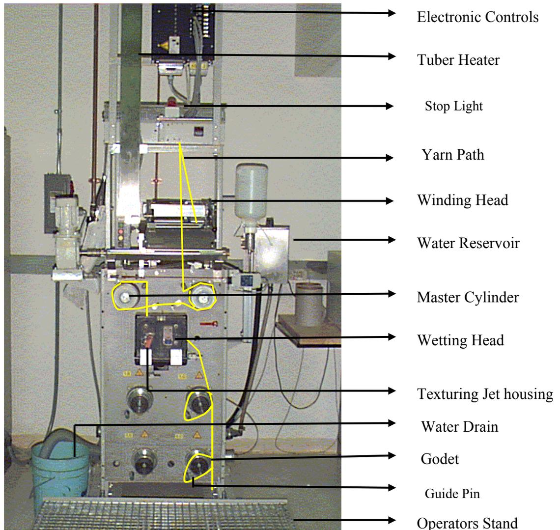
**Figure 4.2:** Complete Assembled Machine
