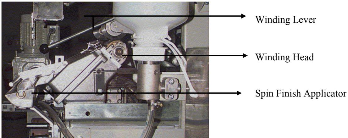
**Figure 4.4:** Winding unit profile
