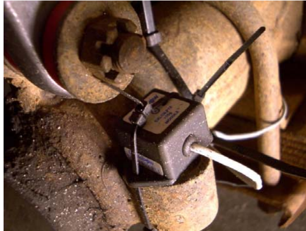
Figure 60. Unsprung mass accelerometer (note leaf-spring pack in background)
