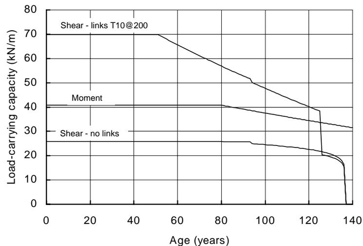
**Figure 8-7:** The effects of omitting shear links on the load-carrying capacity of corrosion-damaged concrete beams
