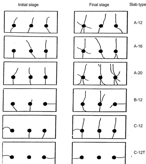
**Figure 2-9:** Observed crack patterns (Cabrera<sup>26</sup>)
