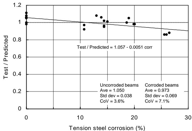
**Figure 5-6:** The variation in the ratio of test/predicted flexural load-carrying capacity with corrosion for beams with reinforcement in the compression zone, ignoring the effects of spalling and allowing for the apparent reduction in yield strength
