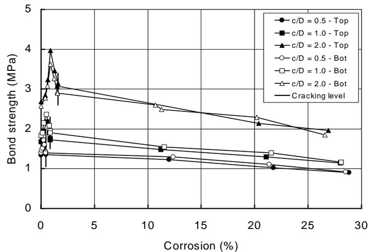
**Figure 2-12:** The relationship between bond strength and corrosion for plain bars (Saifullah<sup>35</sup>)
