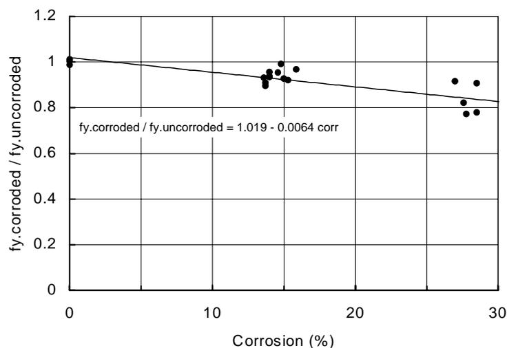
**Figure 5-5:** The variation in the ratio of corroded to uncorroded yield strength of 12 mm ribbed bars subject to accelerated corrosion (Andrade et al<sup>23</sup>)
