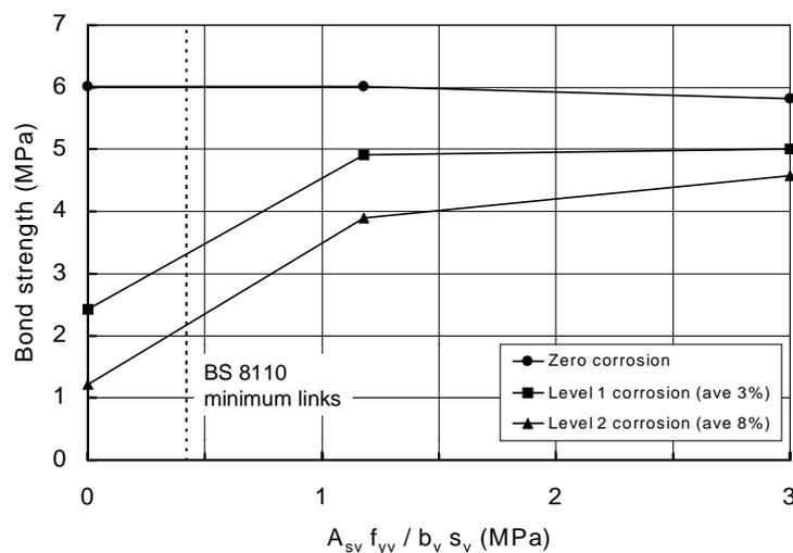
**Figure 4-9:** The effect of corrosion on the bond strength of ribbed reinforcing bars with links (Rodriguez et al<sup>45</sup>)
