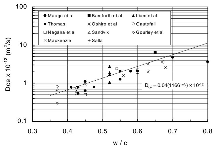
**Figure 2-3:** Relationship between effective diffusion coefficient,  $D_{ce}$ , for concrete and w/c for temperature corrected marine exposure XS3 (Hobbs and Matthews<sup>12</sup>)
