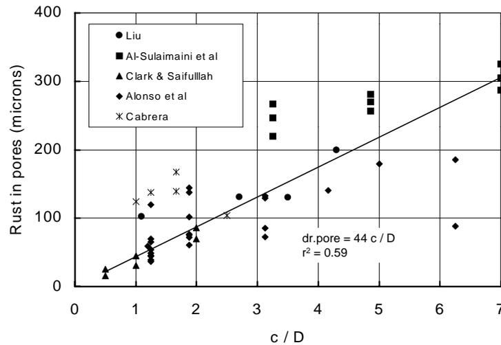
**Figure 3-1:** The relationship between  $\delta r_{pore}$  and cover to bar diameter ratio
