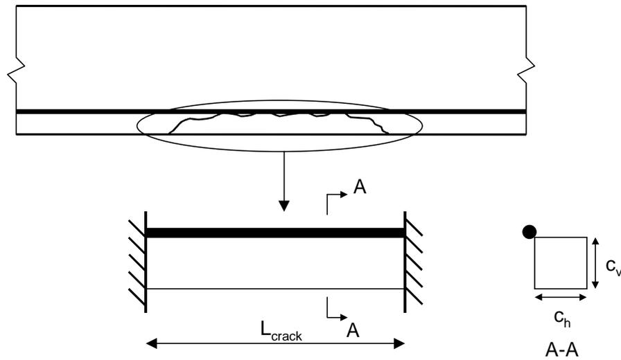
**Figure 3-6:** Idealisation of the spalling of cracked concrete cover to a corner bar
