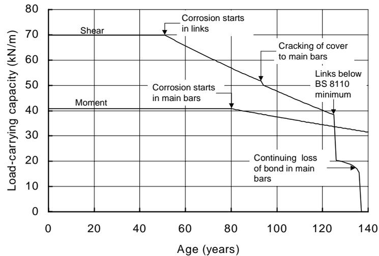
**Figure 8-2:** Reductions in load-carrying capacity for the default beam
