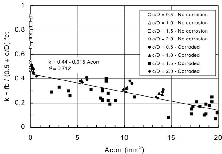
**Figure 4-6:** The relationship between  $A_{corr}$  and  $k$  for ribbed bars ( $c/D = 0.5, 1.0$  and  $2.0$  from Saifullah<sup>35</sup>;  $c/D=1.5$  from Rodriguez et al<sup>45</sup>)
