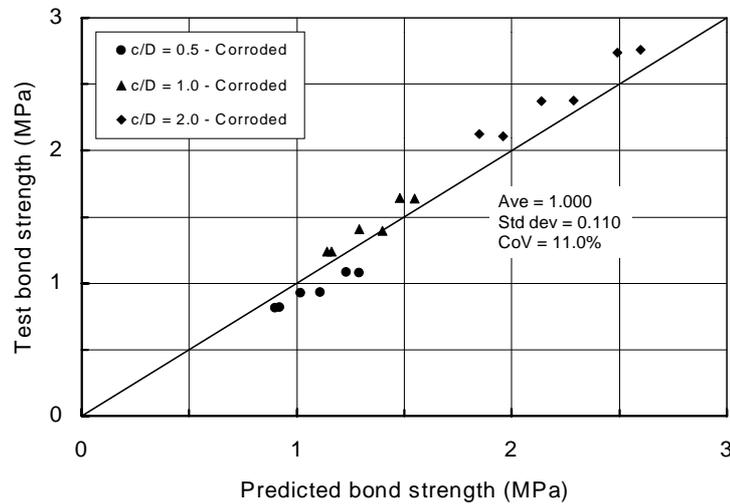
**Figure 4-12:** Comparison between predicted and test bond strength for the corroded plain bars tested by Saifullah<sup>35</sup>
