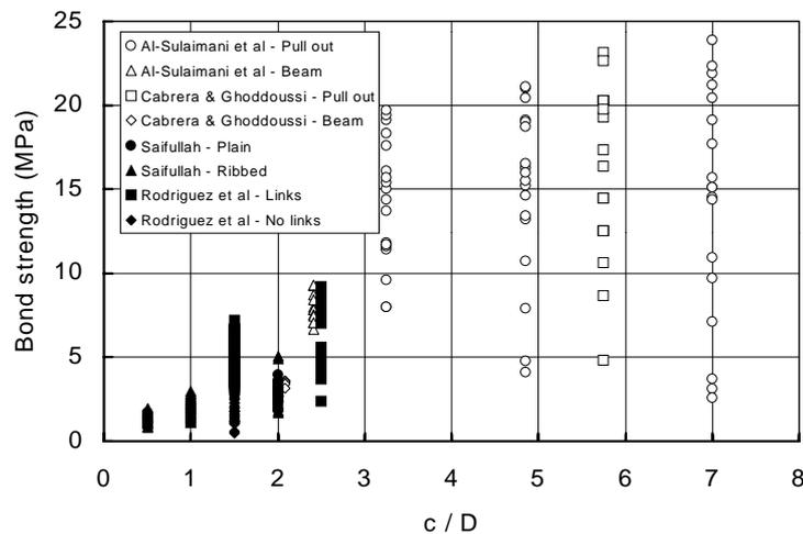
**Figure 4-2:** The effect of  $c/D$  ratio on the bond strength of corroded and non-corroded reinforcement bars
