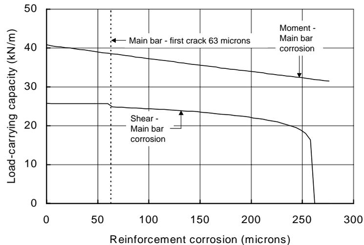
**Figure 8-9:** The relationship between link and main tension reinforcement section loss and load-carrying capacity for the default beam with no shear links
