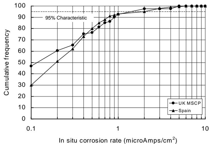
**Figure 2-8:** In situ chloride-induced corrosion rates measured in UK and Spanish structures<sup>17,19</sup>
