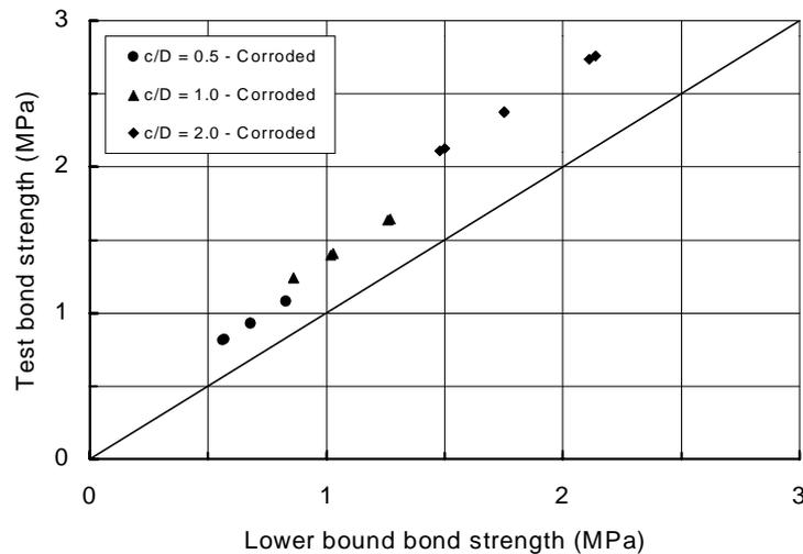
**Figure 4-13:** Comparison between lower bound and test bond strength for the corroded plain bars tested by Saifullah<sup>35</sup>
