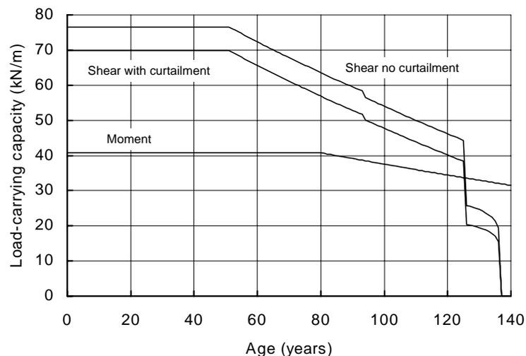
**Figure 8-3:** The effects of curtailment at simple supports on the load-carrying capacity of corrosion-damaged concrete beams
