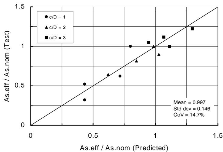
**Figure 6-4:** Comparison of test and predicted ratios of  $A_{s,eff}/A_{s,nom}$
