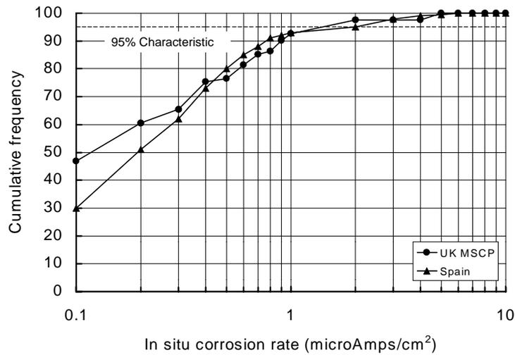
**Figure A3-1:** In situ chloride-induced corrosion rates measured in UK and Spanish structures
