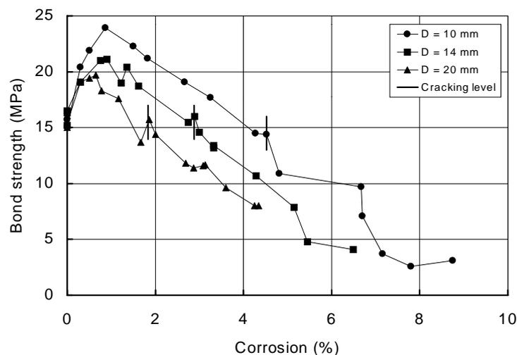
**Figure 2-11:** Relationship between corrosion and bond strength for deformed bars (Al-Sulaimani et al<sup>38</sup>)
