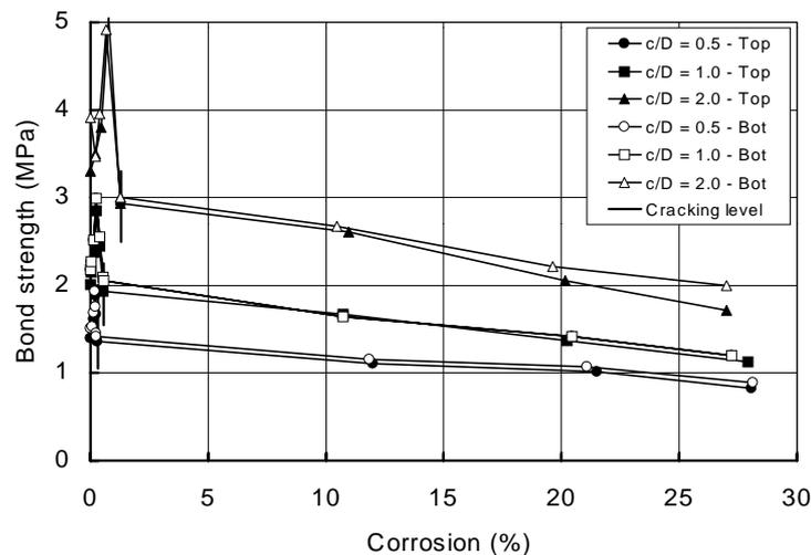
**Figure 2-13:** The relationship between bond strength and corrosion for ribbed bars (Saifullah<sup>35</sup>)
