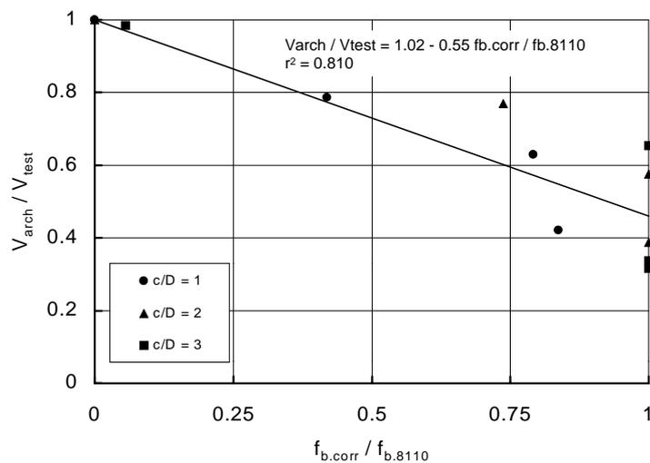
**Figure 6-9:** Variation in the ratio  $V_{\text{arch}}/V_{\text{test}}$  with the ratio  $f_{\text{b,corr}}/f_{\text{b,8110}}$
