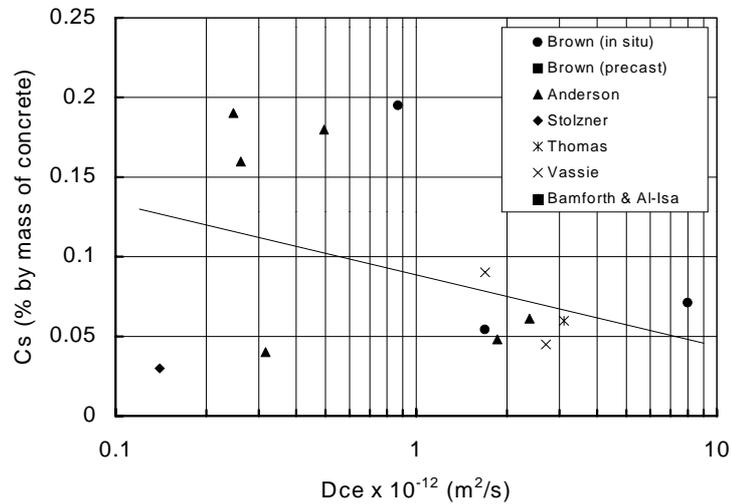
**Figure 2-7:** Relationship between effective diffusion coefficient,  $D_{ce}$ , and surface chloride level,  $C_s$ , for de-icing salt exposure XD3 (Hobbs and Matthews<sup>12</sup>)
