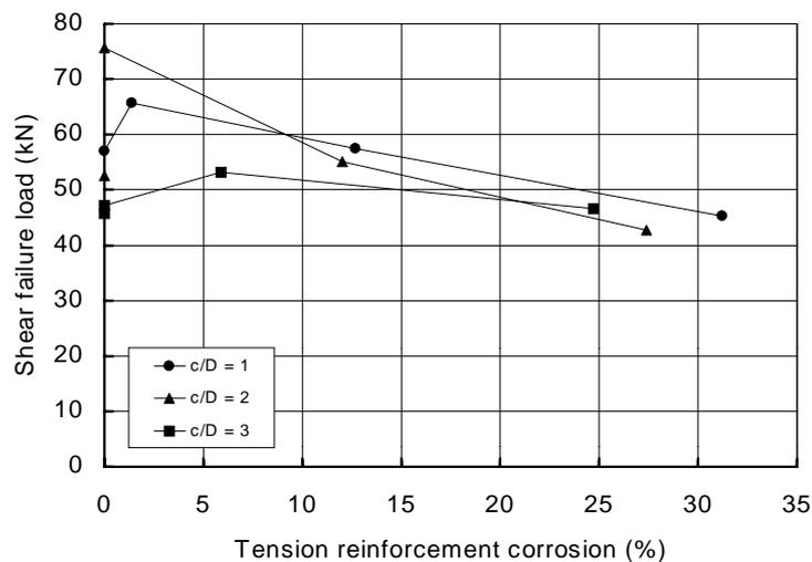
**Figure 6-6:** The variation in shear load-carrying capacity with corrosion for beams with plain bars
