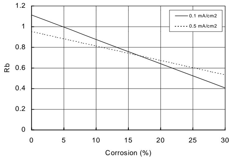
**Figure 4-5:** Possible variations in the ratios of corroded to uncorroded bond strength for corrosion rates used by Rodriguez et al<sup>45</sup> (0.1mA/cm<sup>2</sup>) and Saifullah<sup>35</sup> (0.5mA/cm<sup>2</sup>)
