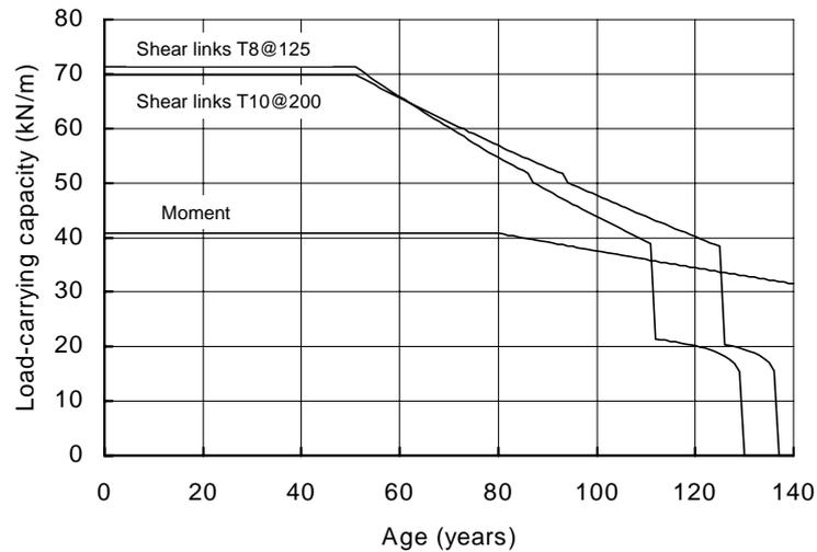
**Figure 8-5:** The effects of varying link size and spacing on the load-carrying capacity of corrosion-damaged concrete beams
