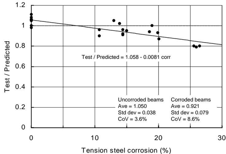
**Figure 5-4:** The variation in the ratio of test/predicted flexural load-carrying capacity with corrosion for beams with reinforcement in the compression zone and including the effects of spalling
