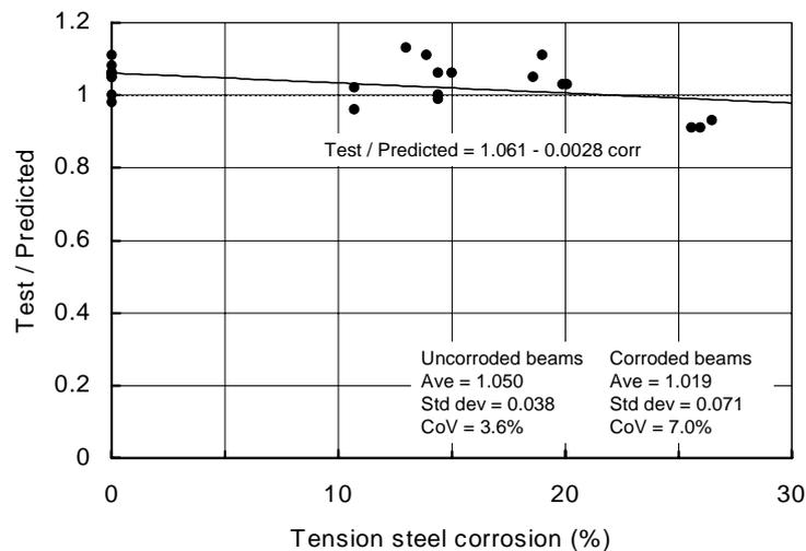
**Figure 5-7:** The variation in the ratio of test/predicted flexural load-carrying capacity with corrosion for beams with reinforcement in the compression zone, including the effects of spalling and allowing for the apparent reduction in yield strength
