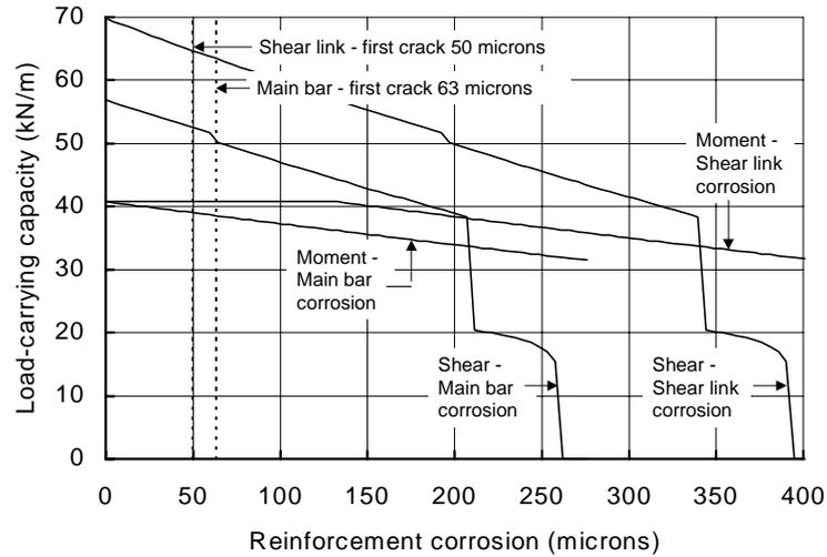
**Figure 8-8:** The relationship between link and main tension reinforcement section loss and load-carrying capacity for the default beam
