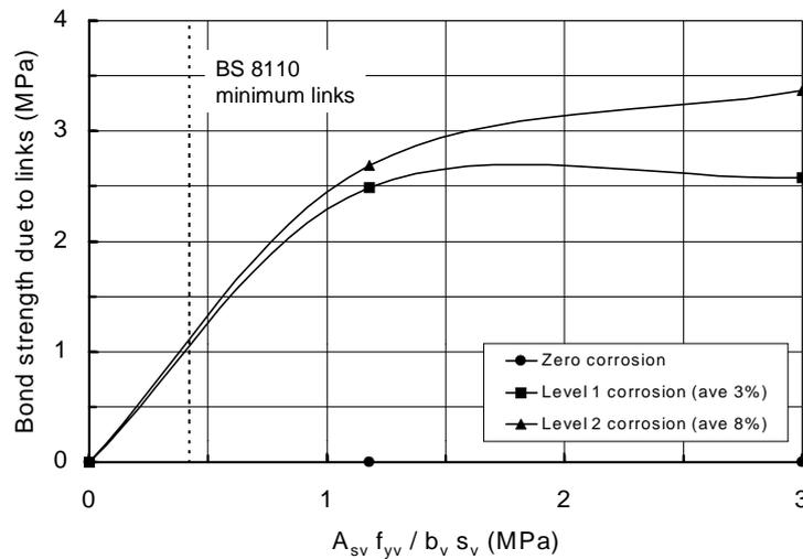
**Figure 4-10:** The enhancement of corroded bond strength due to the presence of links for varying levels of corrosion (Rodriguez et al<sup>45</sup>)
