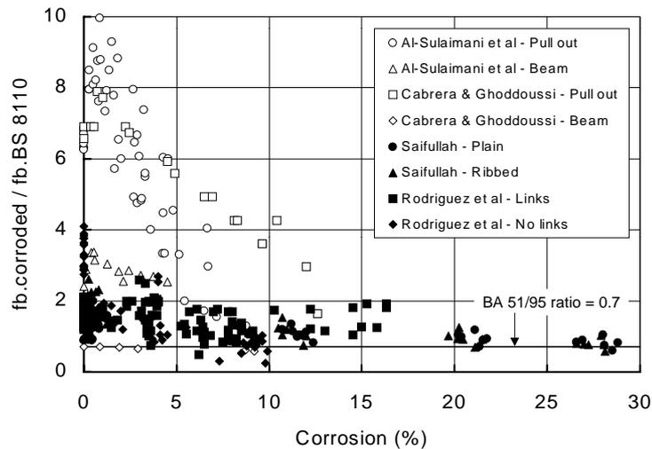
**Figure 4-1:** The effect of corrosion on the bond strength of reinforcing bars in comparison to the ultimate bond strength requirement of BS 8110 for all test data (reference numbers are given in Table 4-2)
