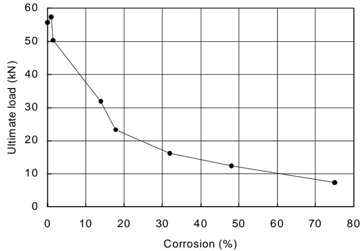
**Figure 2-14:** The variation in slab load-carrying capacity with corrosion (Almusallam et al<sup>53</sup>)
