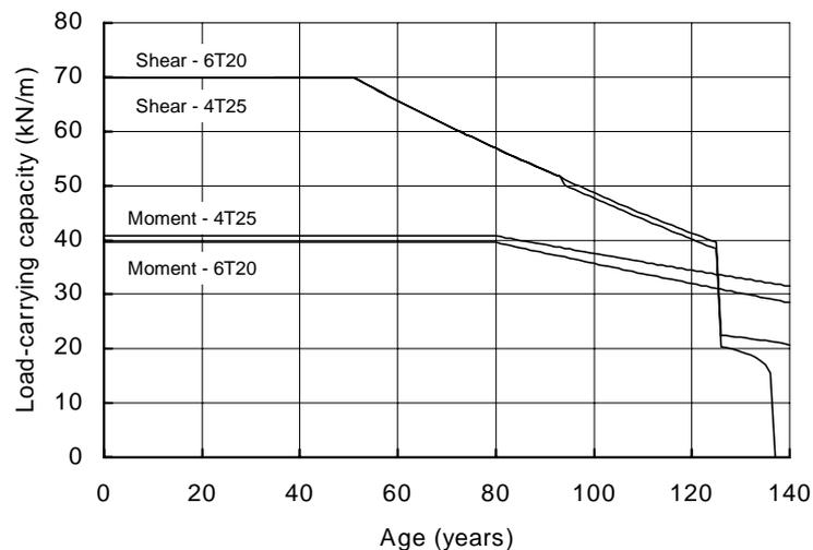
**Figure 8-4:** The effects of different tension reinforcement bar diameters on the load-carrying capacity of corrosion-damaged concrete beams
