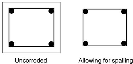
**Figure A11-1:** The effects of spalling on reinforced concrete column cross-sections
