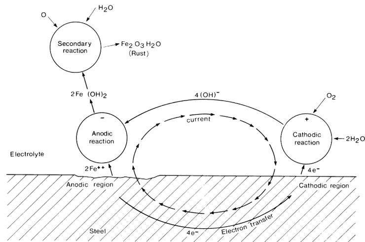
**Figure 2-2:** Anodic and cathodic reactions (Beeby<sup>7</sup>)
