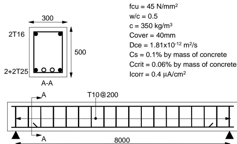
**Figure 8-1:** Reinforced concrete beam with default parameters
