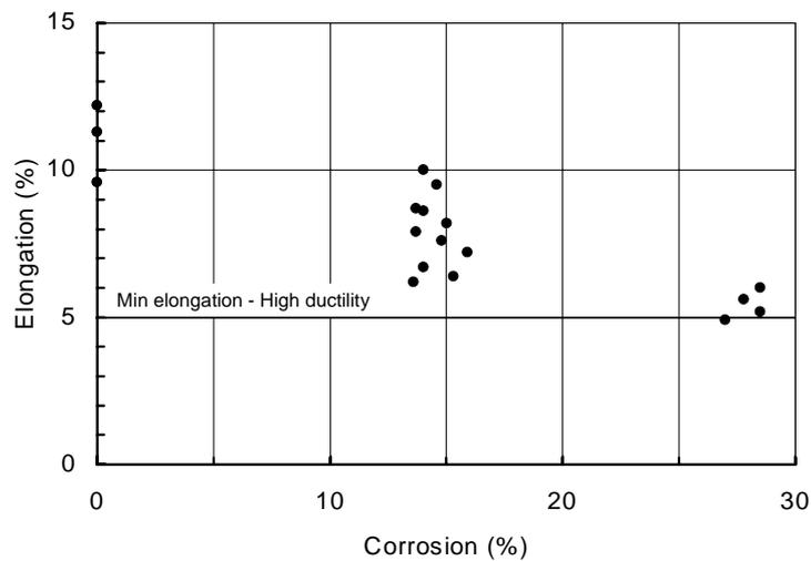
**Figure 5-8:** The effects of accelerated corrosion on the elongation at maximum load of 12 mm diameter ribbed bars (Andrade et al<sup>23</sup>)
