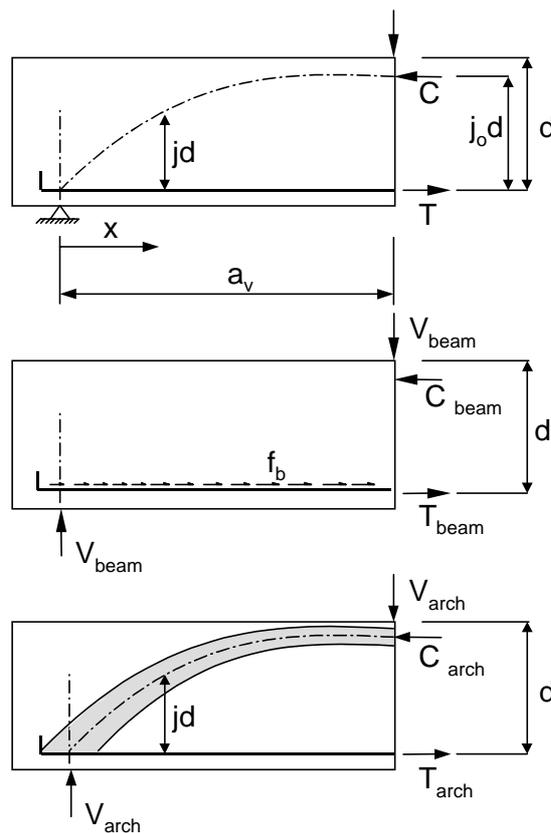
**Figure 6-8:** The beam shear and arch components of shear resistance
