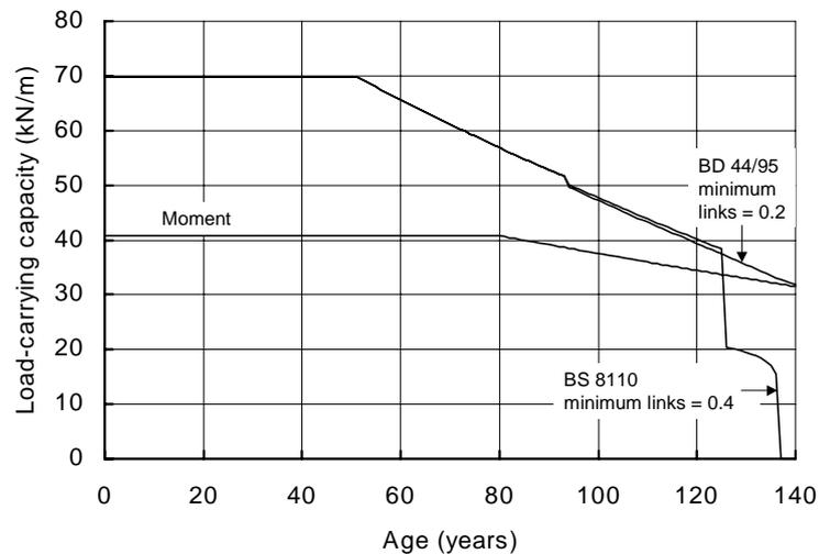
**Figure 8-6:** The effect of varying the requirement for the minimum amount of shear links on the load-carrying capacity of corrosion-damaged concrete beams
