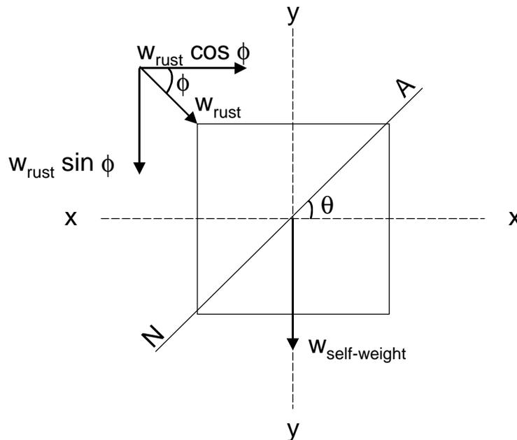
**Figure 3-7:** Components of bending in a section of cover concrete
