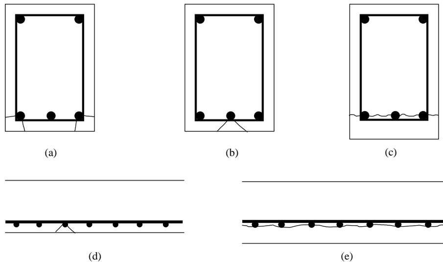
**Figure 3-5:** Types of spalling
