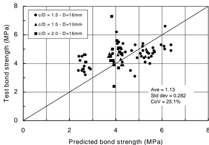
**Figure 4-11:** The comparison of test and predicted bond strength for corroded ribbed bars with uncorroded links (Rodriguez et al<sup>45</sup>)
