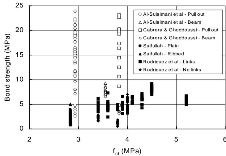
**Figure 4-3:** The effect of concrete tensile strength on the bond strength of corroded and non-corroded reinforcement bars
