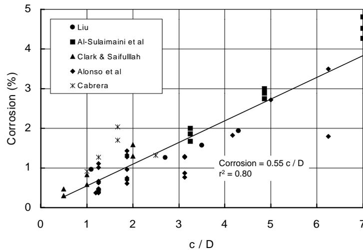
**Figure 3-3:** The relationship between bar weight loss due to corrosion and the  $c/D$  ratio
