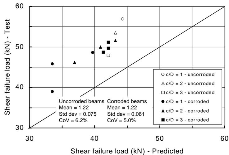
**Figure 6-5:** Comparisons of test and predicted shear load-carrying capacities
