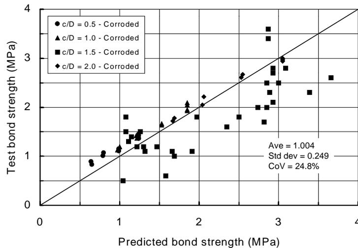
**Figure 4-7:** Comparison between predicted bond strength and test bond strengths for corroded ribbed bars with no links ( $c/D = 0.5, 1.0$  and  $2.0$  from Saifullah<sup>35</sup>;  $c/D=1.5$  from Rodriguez et al<sup>45</sup>)
