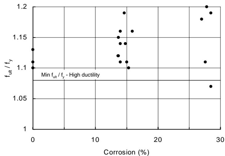
**Figure 5-9:** The effects of accelerated corrosion on the ratio  $f_{ult}/f_y$  of 12 mm diameter ribbed bars (Andrade et al<sup>23</sup>)
