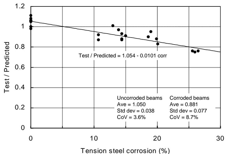
**Figure 5-3:** The variation in the ratio of test/predicted flexural load-carrying capacity with
