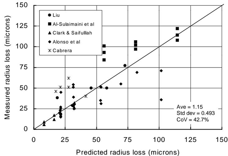
**Figure 3-2:** Comparison of measured and predicted radius loss to induce cracking
