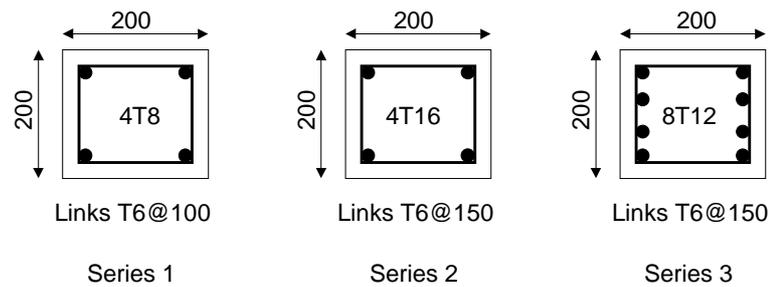
**Figure 7-2:** Cross-sections of the columns tested by Rodriguez et al<sup>68</sup>
