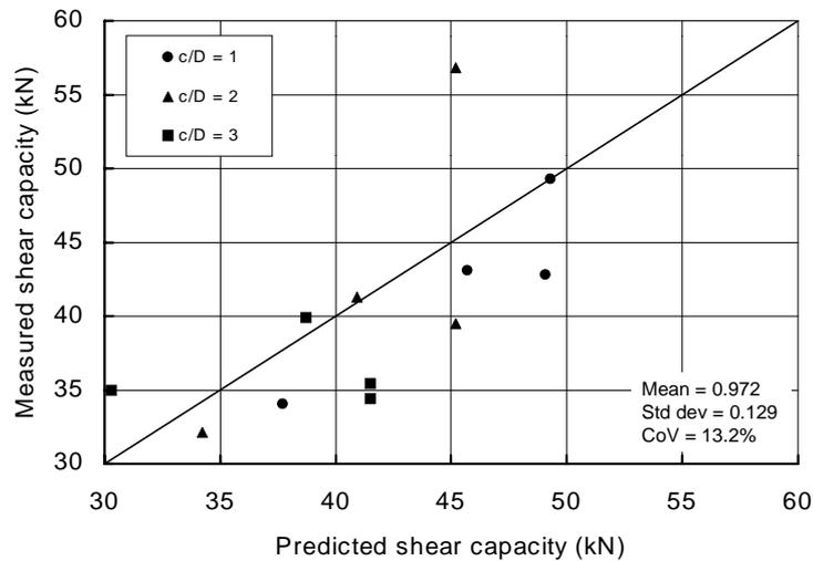
**Figure 6-11:** Comparison of measured and predicted shear load-carrying capacity for the beams tested by Daly<sup>66</sup> and containing corroded plain reinforcement
