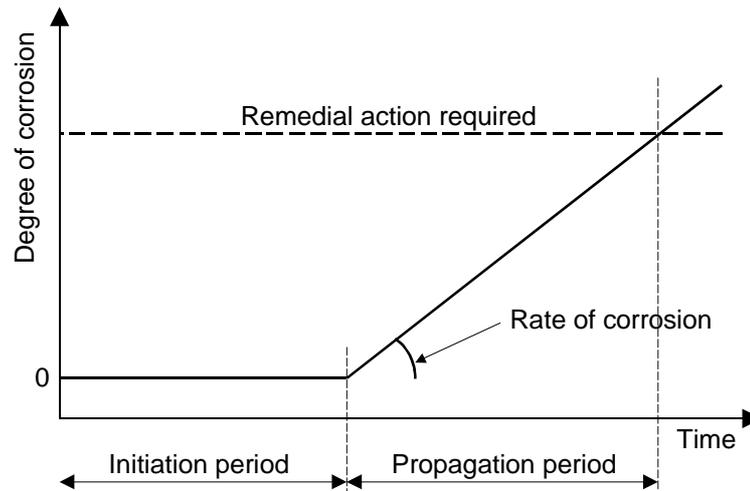
**Figure 2-1:** The corrosion process (Tuutti<sup>5</sup>)
