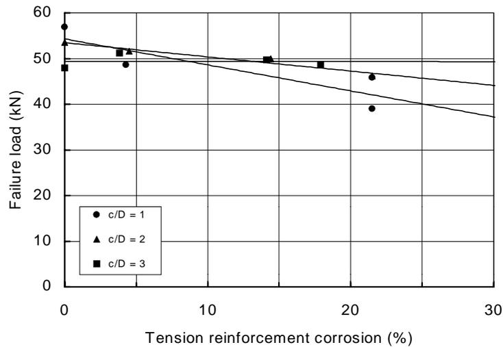
**Figure 6-1:** The variation in load-carrying capacity with corrosion for beams failing in shear (Daly<sup>66</sup>)
