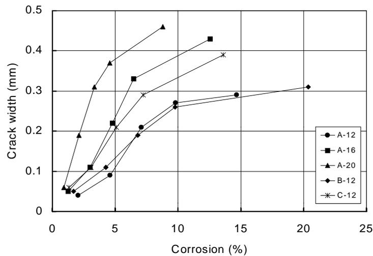
**Figure 2-10:** Relation of average crack width to corrosion (Cabrera<sup>26</sup>)
