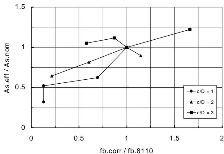
**Figure 6-2:** The variation in  $A_{s,eff}/A_{s,nom}$  with the ratio  $f_{b,corr}/f_{b,8110}$
