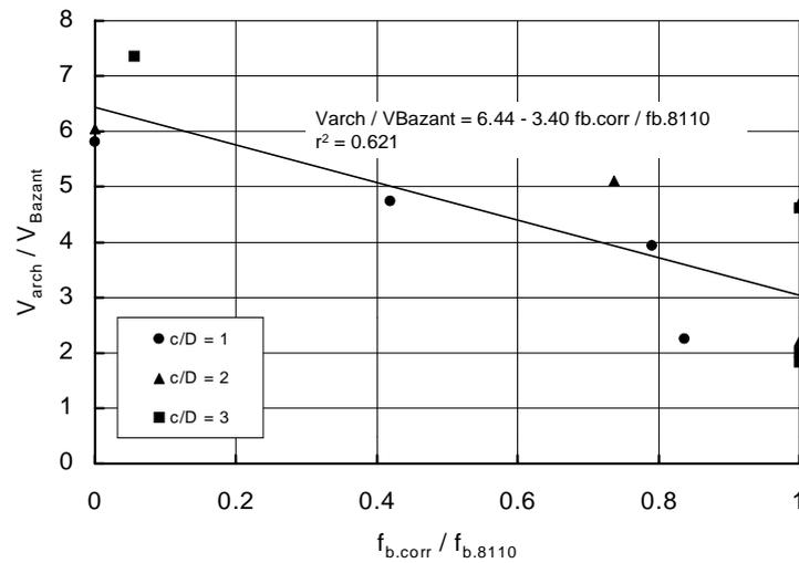
**Figure 6-10:** Variation in the ratio  $V_{arch} / V_{Bazant}$  with the ratio  $f_{b.corr} / f_{b.8110}$
