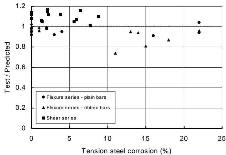
**Figure 5-1:** The ratio of test/predicted load-carrying capacity for singly-reinforced beams with varying amounts of corrosion and failing in flexure (Daly<sup>64, 66</sup>)
