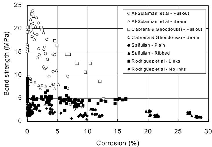
**Figure 4-4:** The effect of corrosion on the bond strength of reinforcement bars
