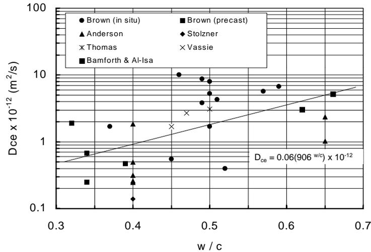
**Figure 2-6:** Relationship between effective diffusion coefficient,  $D_{ce}$ , for concrete and w/c ratio for de-icing salt exposure XD3 (Hobbs and Matthews<sup>12</sup>)
