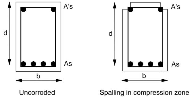
**Figure A8-1:** The effects of spalling in the compression zone of reinforced concrete beams
