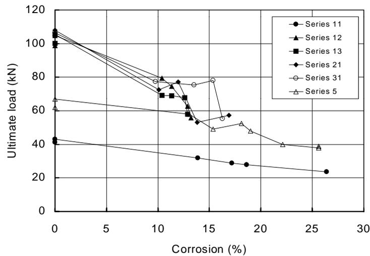
**Figure 2-15:** The variation in load-carrying capacity with tension reinforcement corrosion (Rodriguez et al<sup>45</sup>)
