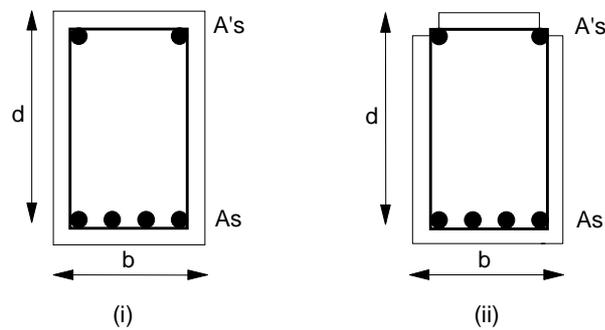
**Figure 5-2:** Sections used to analyse test specimens (i) Ignoring spalling in the compression zone; (ii) Considering spalling in the compression zone
