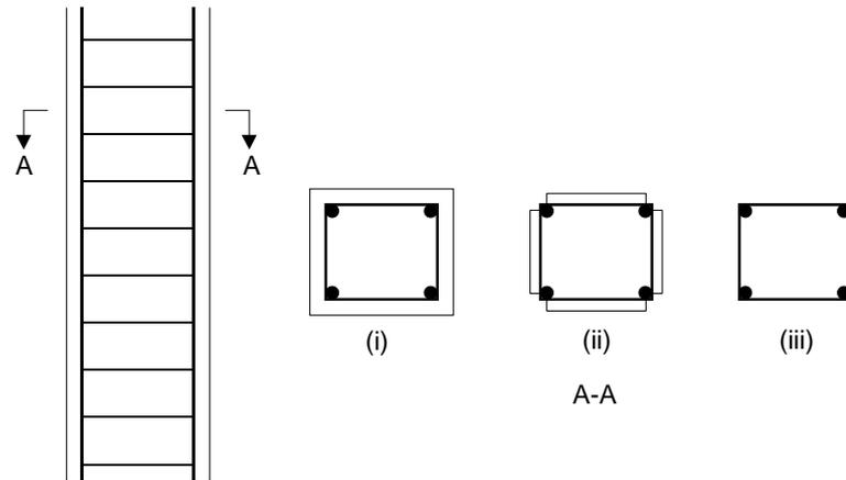
**Figure 7-1:** Various cross-sections used for the analysis of concrete columns with corroded reinforcement
