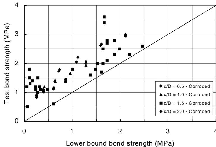
**Figure 4-8:** Comparison between predicted lower bound bond strength and test bond strength for corroded ribbed bars with no links ( $c/D = 0.5, 1.0$  and  $2.0$  from Saifullah<sup>35</sup>;  $c/D=1.5$  from Rodriguez et al<sup>45</sup>)
