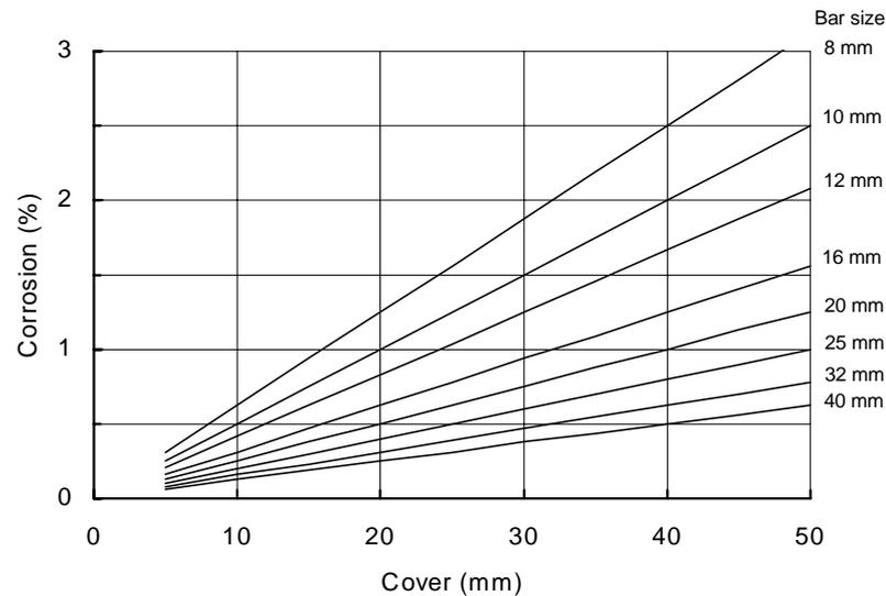
**Figure 3-4:** The predicted relationship between bar section loss required for corrosion-induced cracking and a range of covers and bar size
