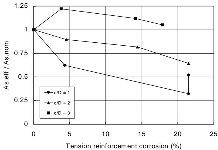
**Figure 6-3:** The variation in  $A_{s,eff}/A_{s,nom}$  with tension reinforcement corrosion
