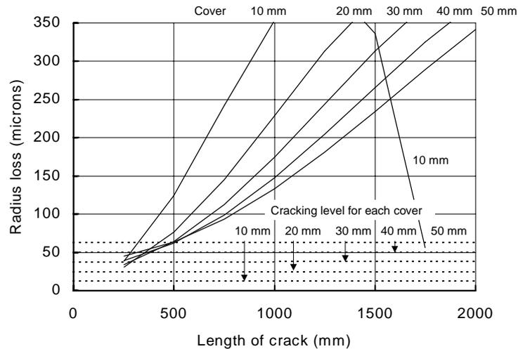
**Figure 3-8:** Predicted radius losses required to spall the cover concrete to a corner bar for various covers and crack lengths (C30 concrete and 20 mm reinforcing bar)
