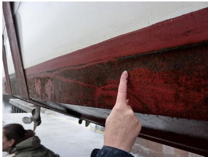
Figure 1.2: Ship's hull protected with FR/AF coating and colonised by filamentous brown algae, identify as ectocarpoid species (Photo: Callow J.A.).
