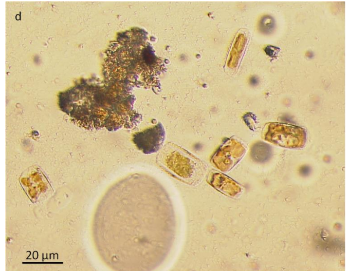
Figure 10.6: Visual appearance of slides on test surfaces in the open slide boxes, after 7 days (a and b) and representative microscope images of the surface biofilm on H2 after 7 days (c) and H1 after 10 days (d) showing presence of diatoms and agglomerations of detritus. No images of bacteria observed under UV microscope have been shown, as the staining was too weak.
