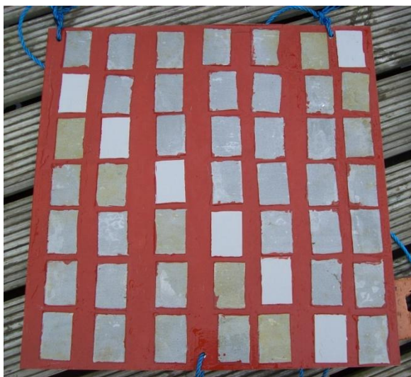
Figure 11.1: Panel before immersion. The panels were attached to a weight in order to be in vertical position. Two ropes were attached to the pontoons to keep the panel in the same position during the field experiment.
