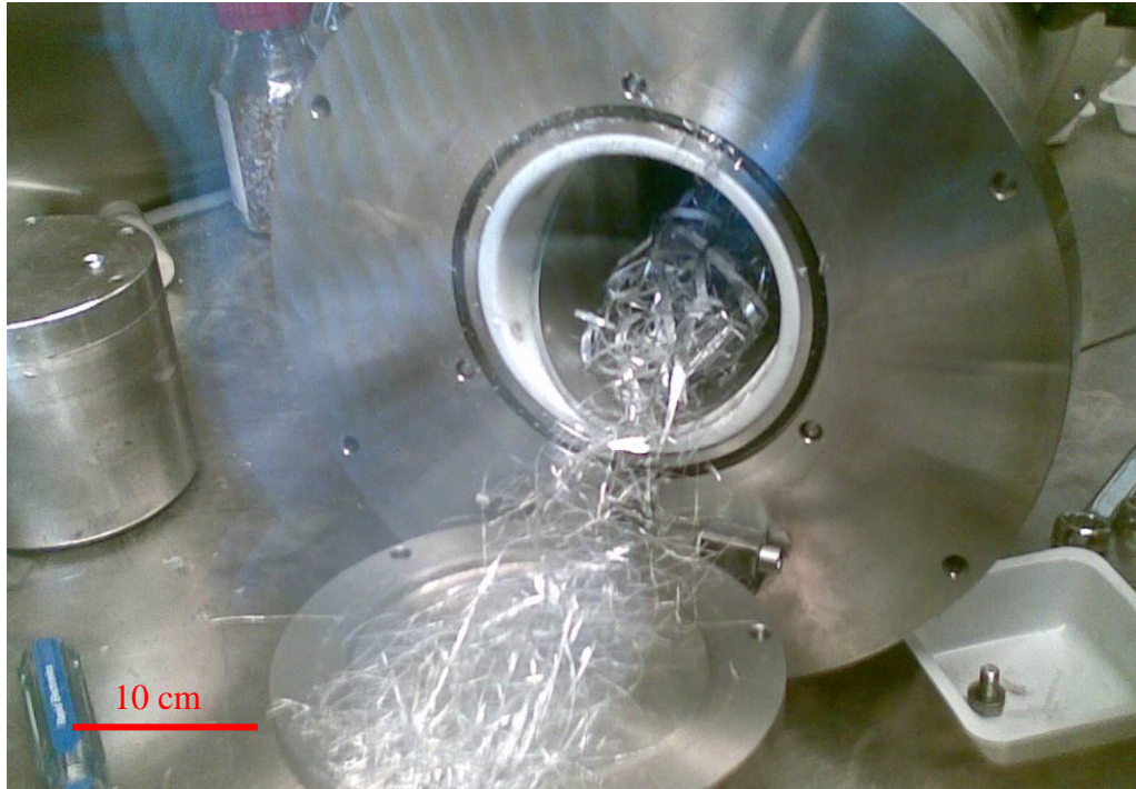
Figure 6-4 Melt-spun Mg ribbons collected from the inert collection tube inside an argon glove box
