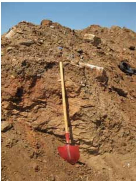
The overlying soil thickness at the site area can reach depths of approx. 5 m. Bedrock is occasionally observed at the surface of the upper parts of the dump site area. The colour of the soil is reddish to brown.
