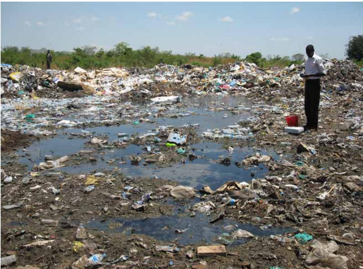
**Photo 6: Collecting a leachate sample from a logged pool, Sample No. 3**
