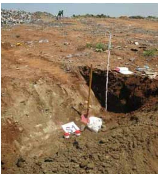
Photo 1: Excavation pit, Sample No. 1
