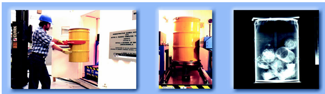
Waste inspection tomography identifies the characteristics of the contents of a waste drum without the risk of opening the container for analysis.
