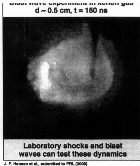
Fig. 8. Radiative shocks such as supernova blast waves can be simulated using scaled gas-filled targets illuminated by energetic laser beams. The photograph on the left is a Supernova Remnant (SNR) in Cassiopeia-A, which occurred in the year 1680. In the image on the right a beam incident from the left has initiated an expanding radiatively driven shock that is outrunning the material expansion from the target itself. This is seen as the faint glow surrounding the brighter inner sphere.
