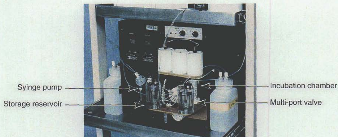
Figure 2. APDS sample preparation unit uses simple SIA hardware (syringe pump, holding coil, multi-port valves, incubation chamber) to reproduce lab bench protocols.
