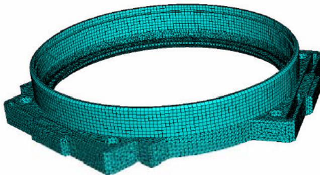
Figure 48. Finite Element Mesh of Lens Housing.
