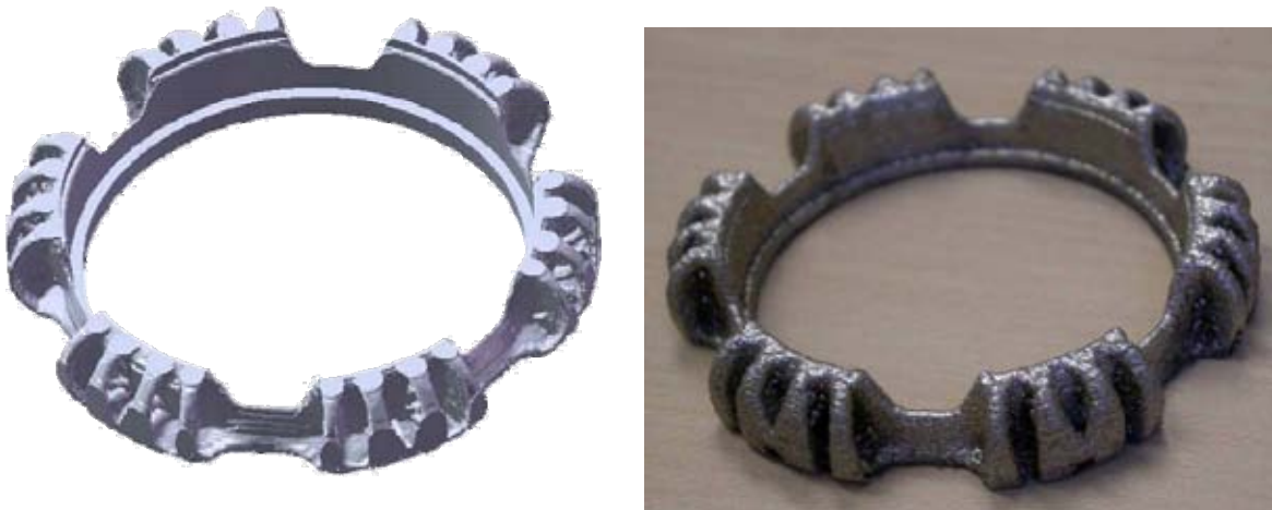
Figure 51. ATO Optimized 3D Lens Housing (left) and LENS Manufactured Housing (right).
