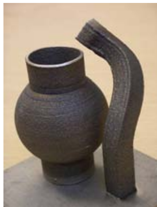
Figure 46. Curved 3D Parts Built From 316 Stainless Steel Using the LENS Process.
