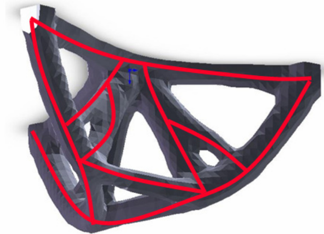
Figure 44. This optimized structure has medial axis splines that were sketched onto the surface of the part by a user.
