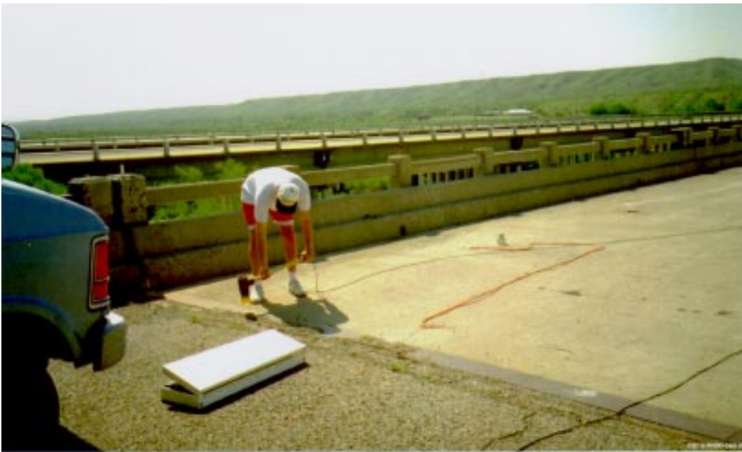
Figure 21. An impact being applied to position 2.
