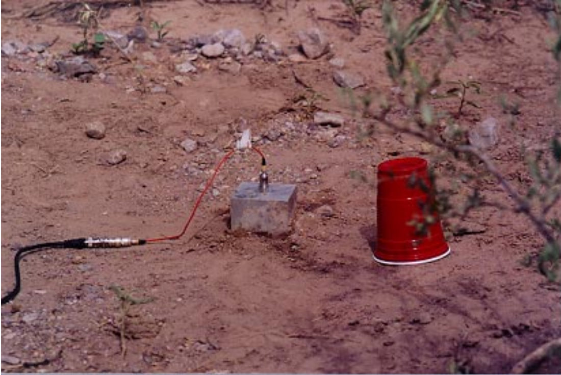
Figure 54. Accelerometer located midway between the I-25 Bridge and the Alamosa Canyon Bridge.
